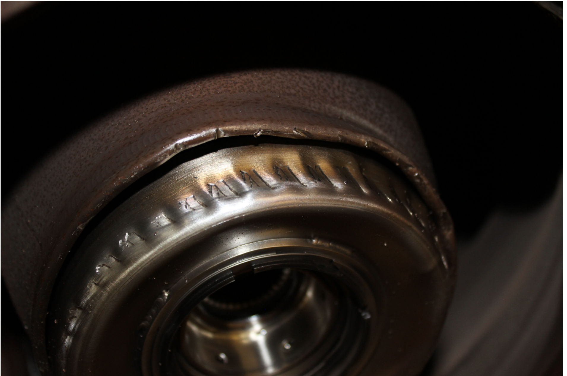
Photo 7 – Impact marks on #3 bearing cover
