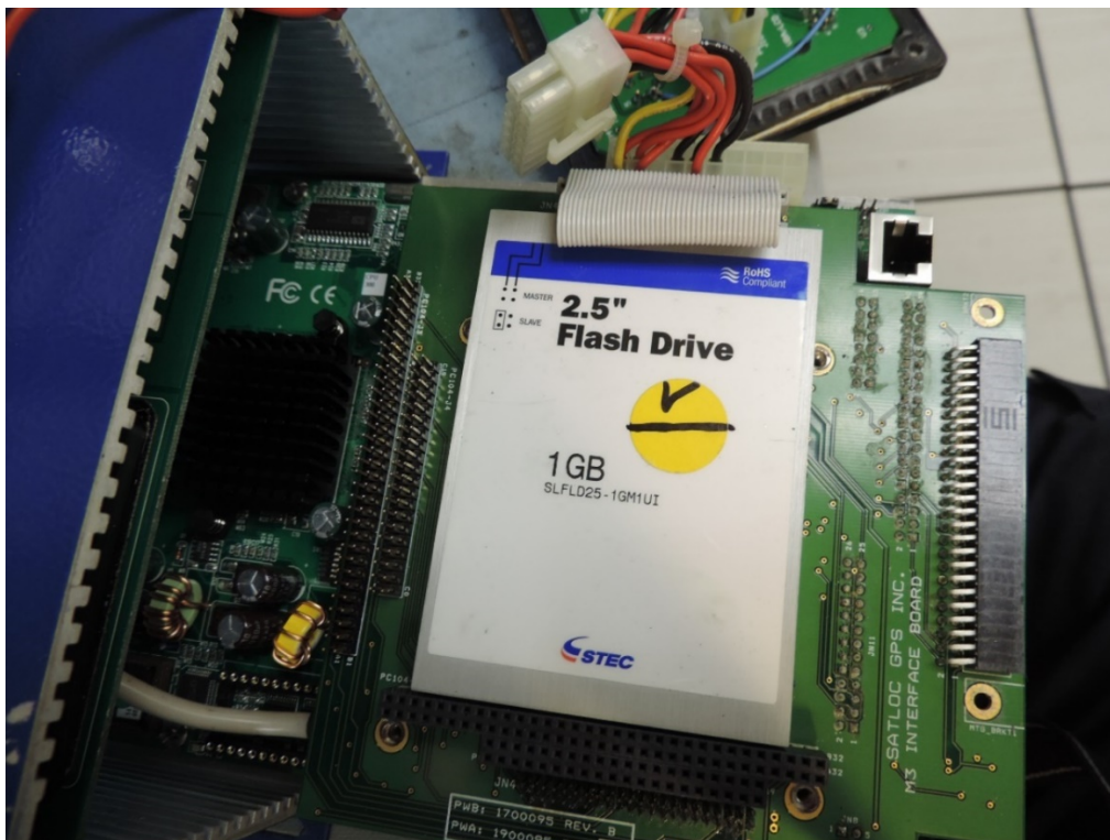
Figure 2. Internal view of the SATLOC M3 CPU showing internal Flash drive.
