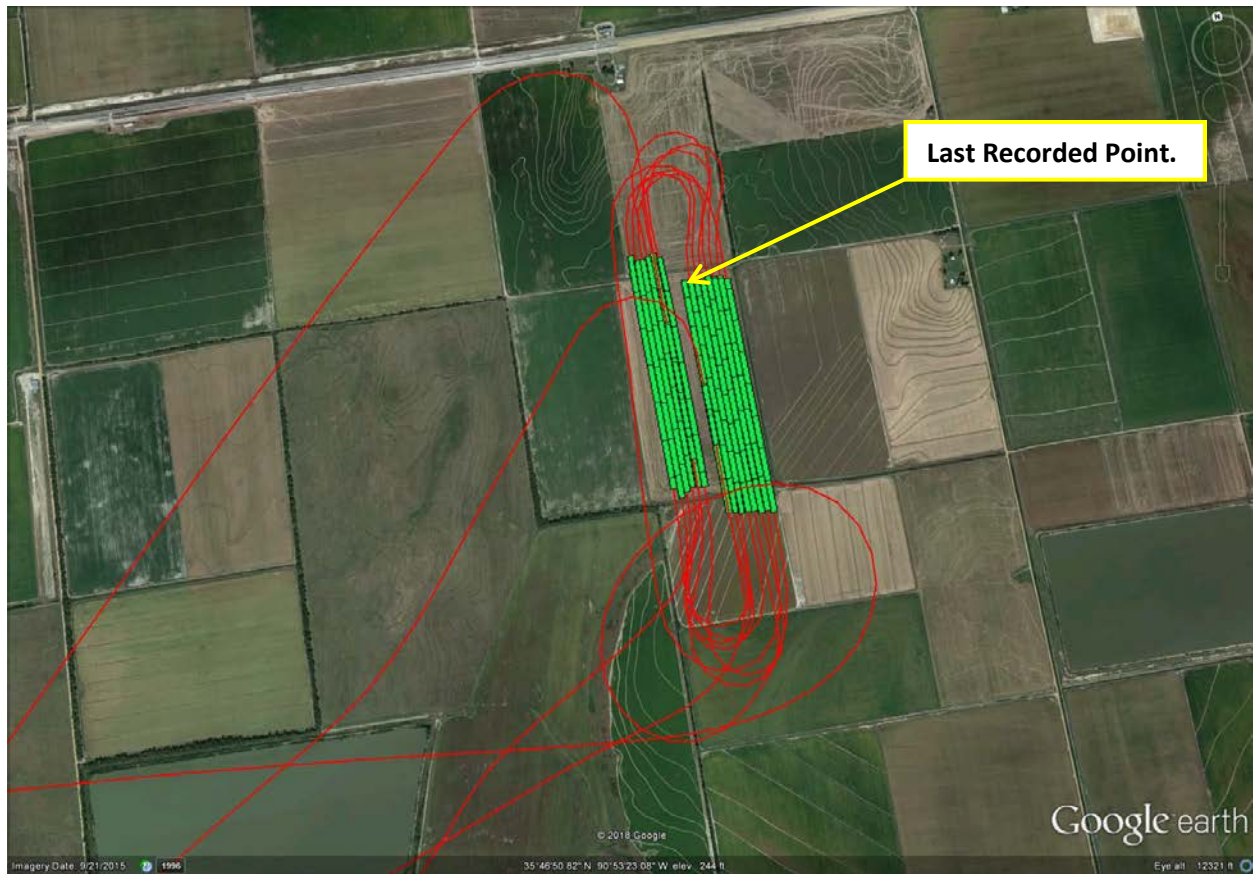
Figure 4. Google Earth 2-D overlay depicting the spray pattern followed at the last field to be treated during the accident flight.
