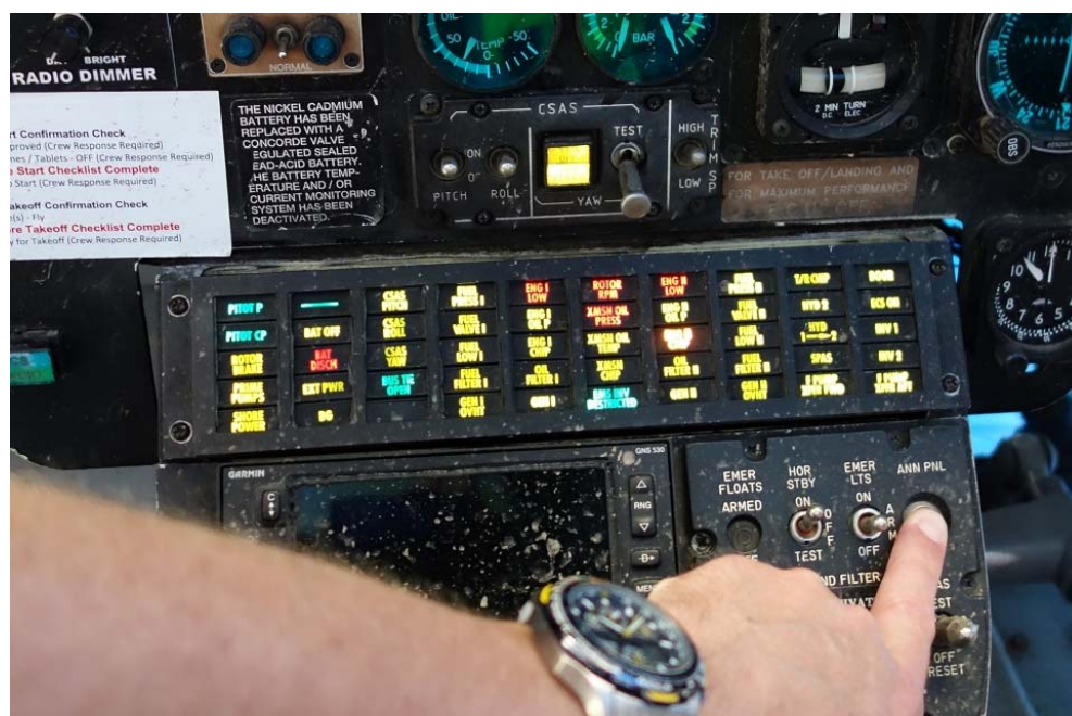
Figure 5. The advisory, caution, and warning annunciator panel with the dimming function turned off and the annunciator panel test button depressed. (courtesy of Air Methods)
