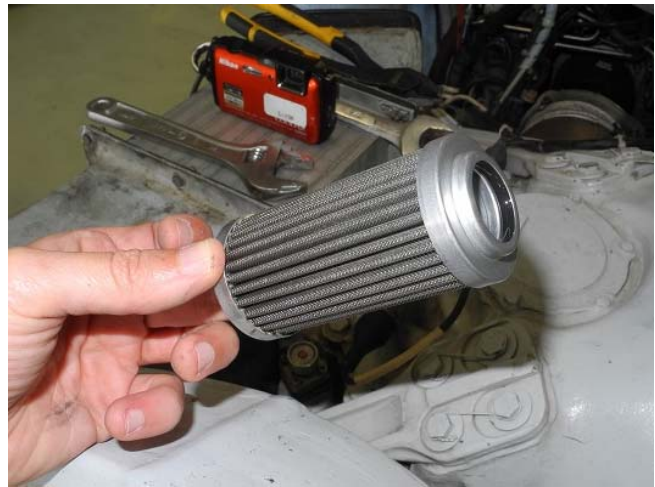
Figure 10. No. 2 engine fuel filter.
