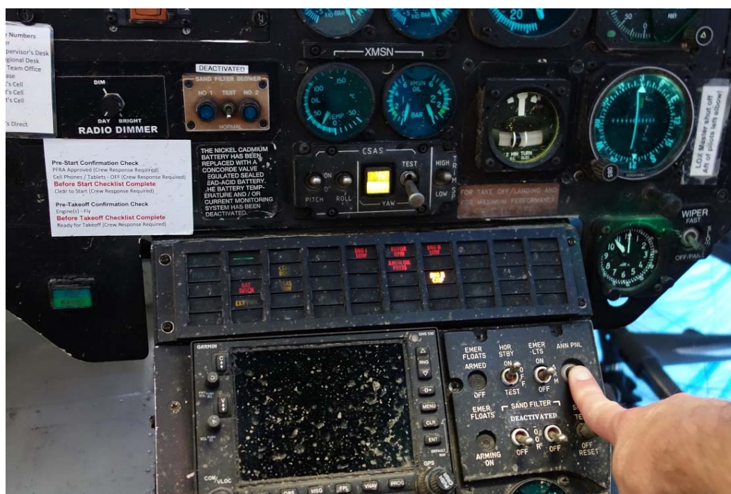
Figure 6. The advisory, caution, and warning annunciator panel with the dimming function turned on and the annunciator panel test button depressed. (courtesy of Air Methods)
