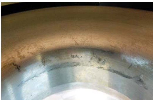
Photo #5 – Compressor housing rub and wheel impact marks
