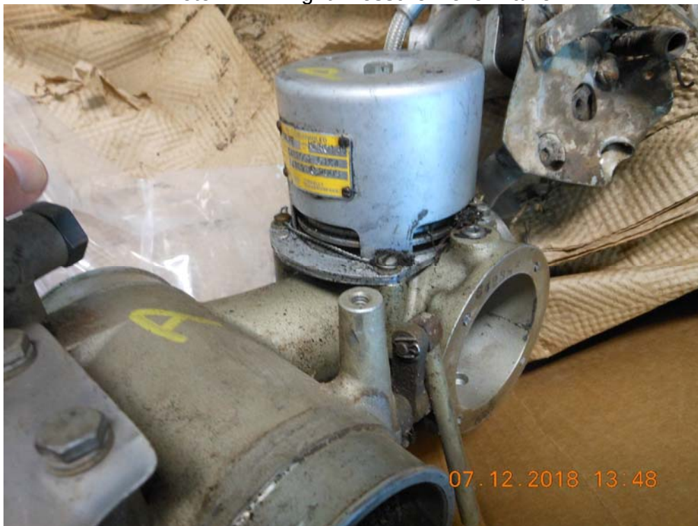
Photo #14 – Right Pressure Relief Valve
