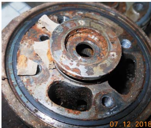
Photo #7 – Thrust bearing/collar condition Left Right (note silt deposits on left)
