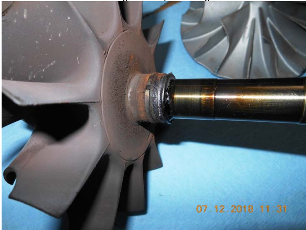
Photo #11 – Right shaft/piston ring condition
