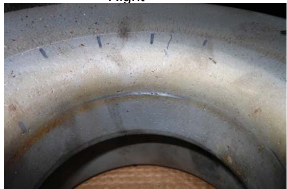
Photo #5 – Compressor housing rub and wheel impact marks
