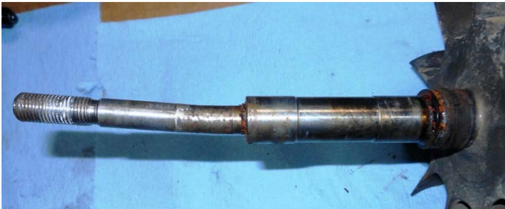
Photo #10 – Left shaft bent
