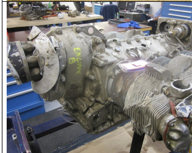
The engine was place on a stand, and readied for disassembly.
