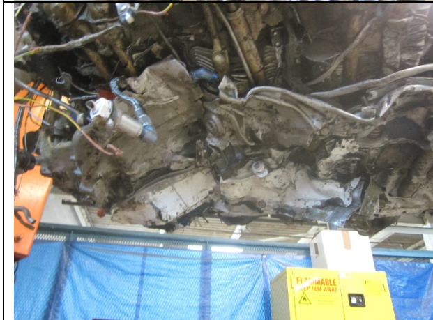
Heavy impact damage is noted to the bottom of the engine.
