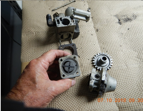
Fuel pump; the drive shaft, "shear pin" was broken.
