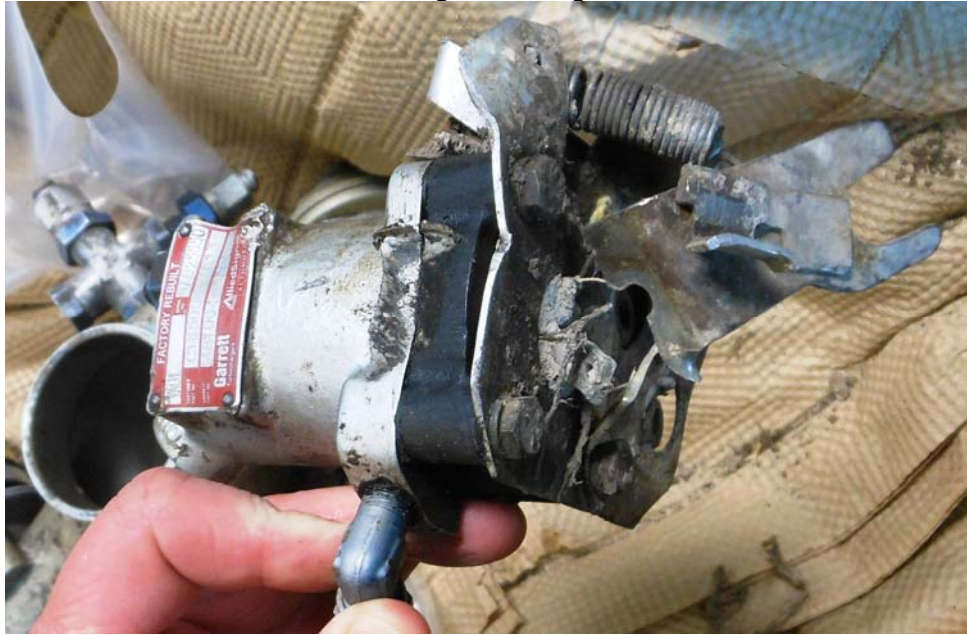
Photo #13 – Right wastegate actuator
