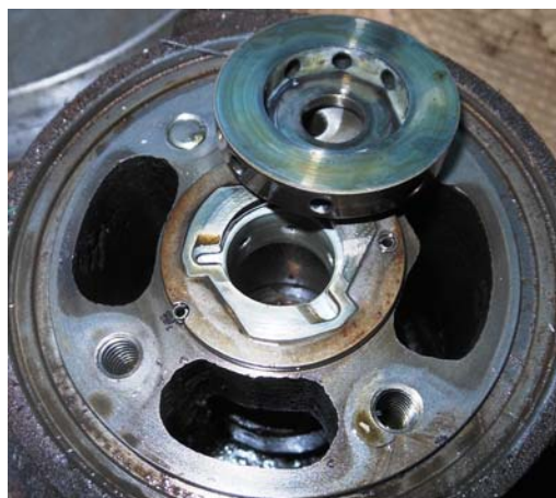
Photo #7 – Thrust bearing/collar condition Left Right (note silt deposits on left)
