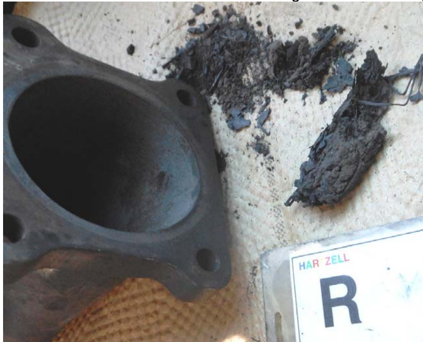
Photo #12 – Charred/burnt debris from right turbine housing
