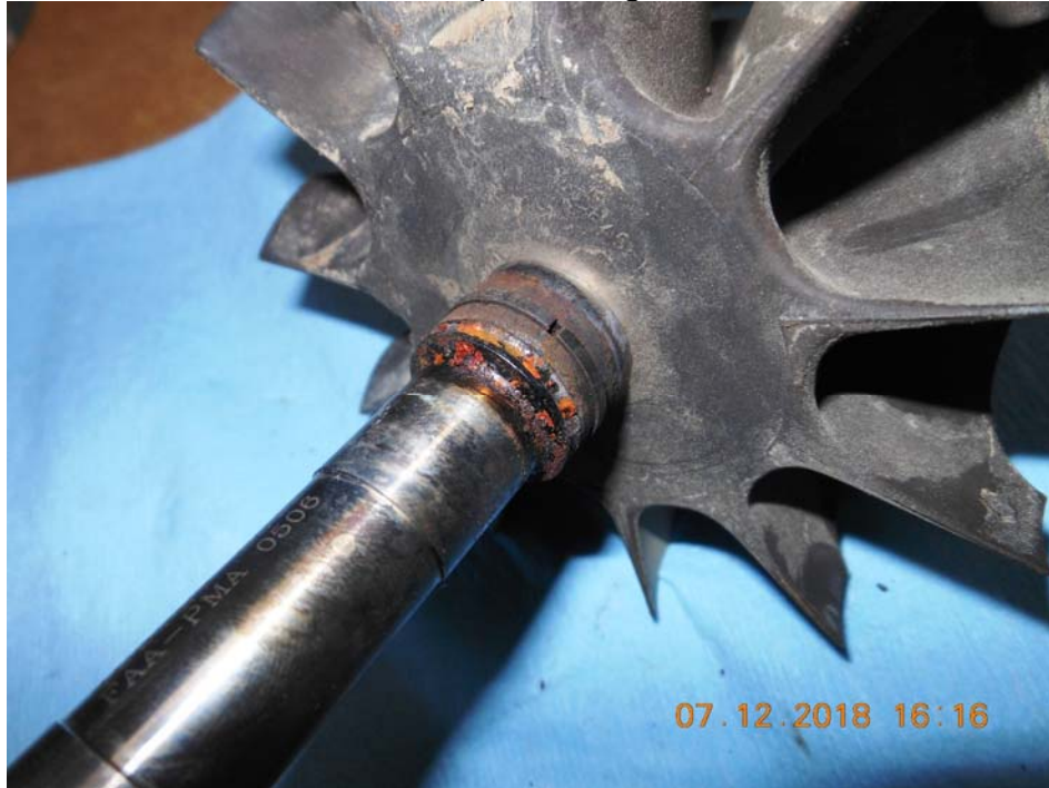
Photo #9 – Left shaft, piston ring and turbine wheel
