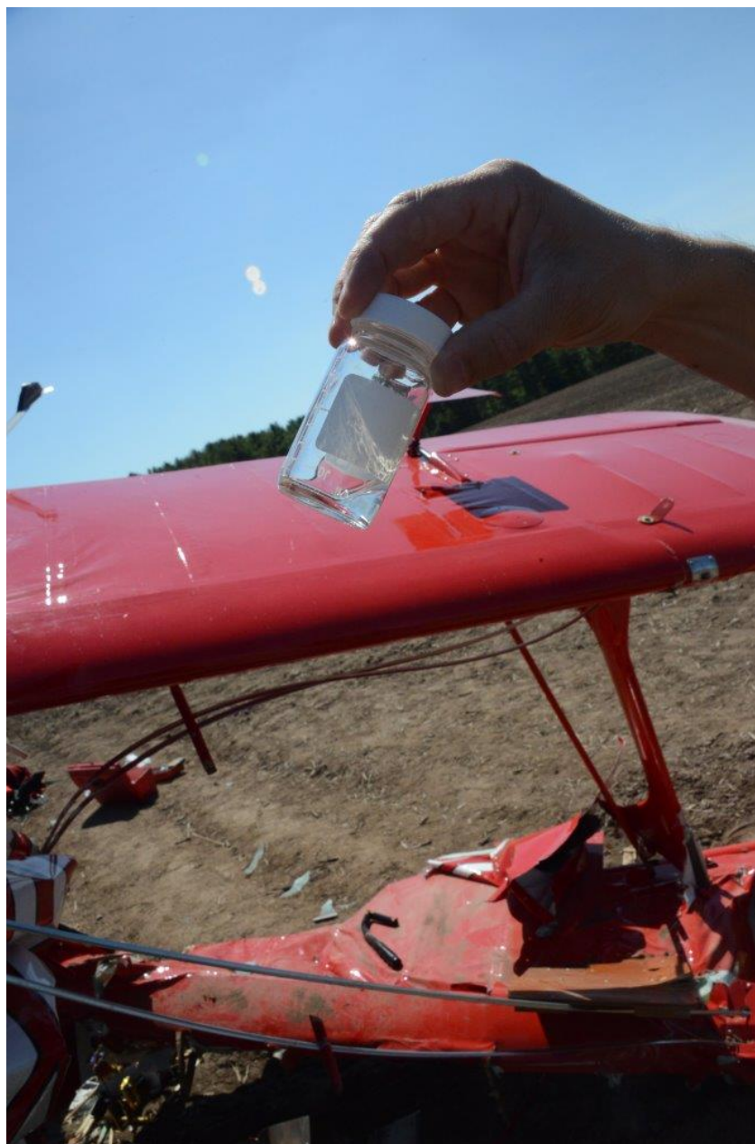
Photo 15 - View of recovered liquid from the fuel system.
