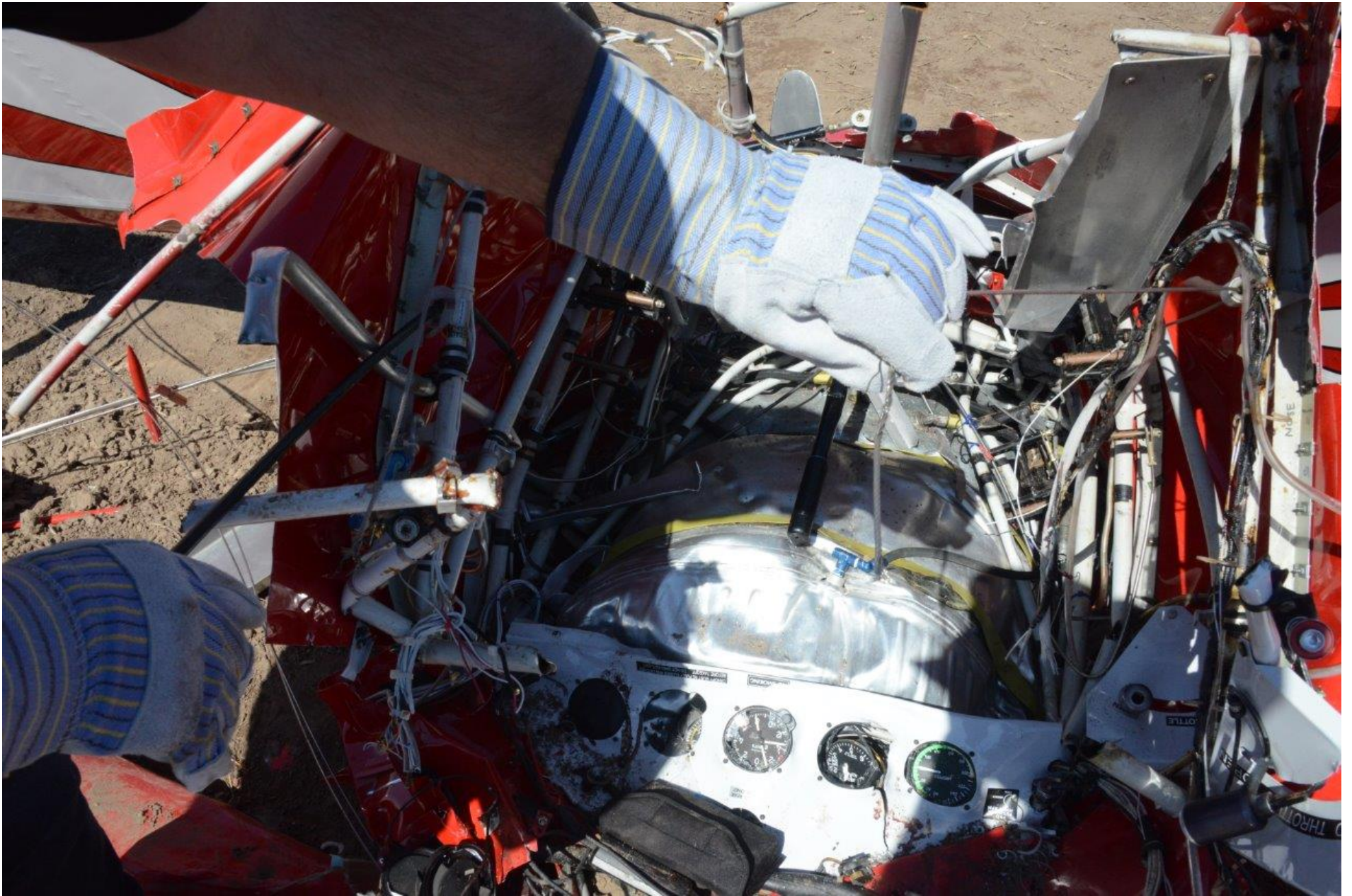
Photo 9 - View of separations in the flight control cables.
