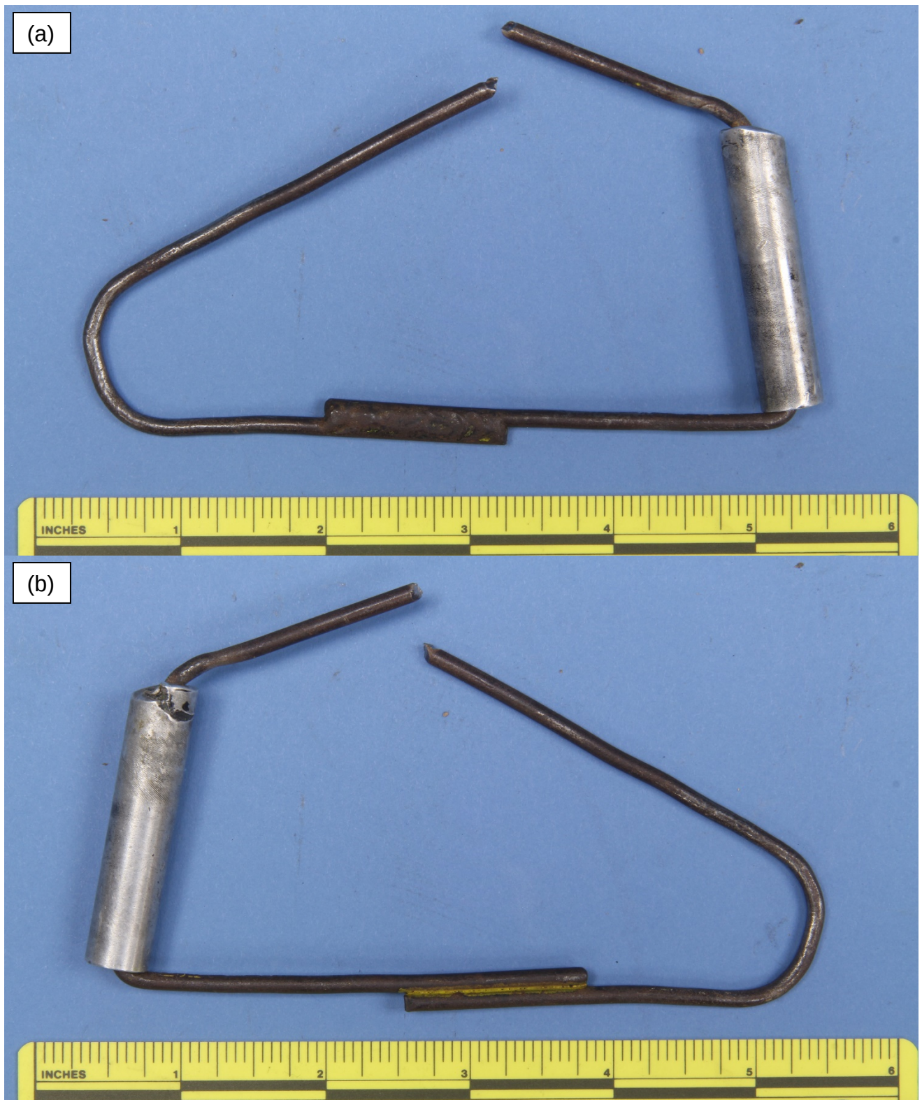
Figure 2 – The exemplar right side wire bracket as received viewed from (a) the obverse and (b) the reverse side. The upper bent portion had been cut prior to receipt.
