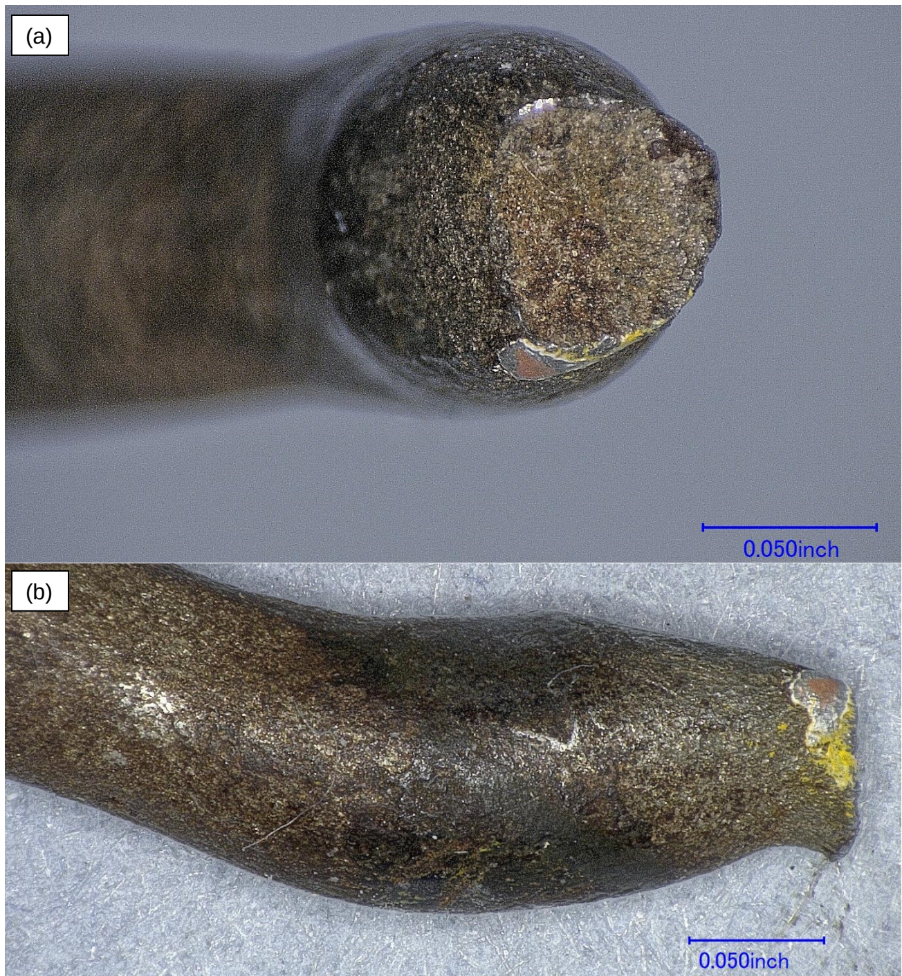
Figure 5 – The flat side fracture (lower fracture in Figure 1) viewed (a) end on, showing two visually distinct regions and (b) from the side.
