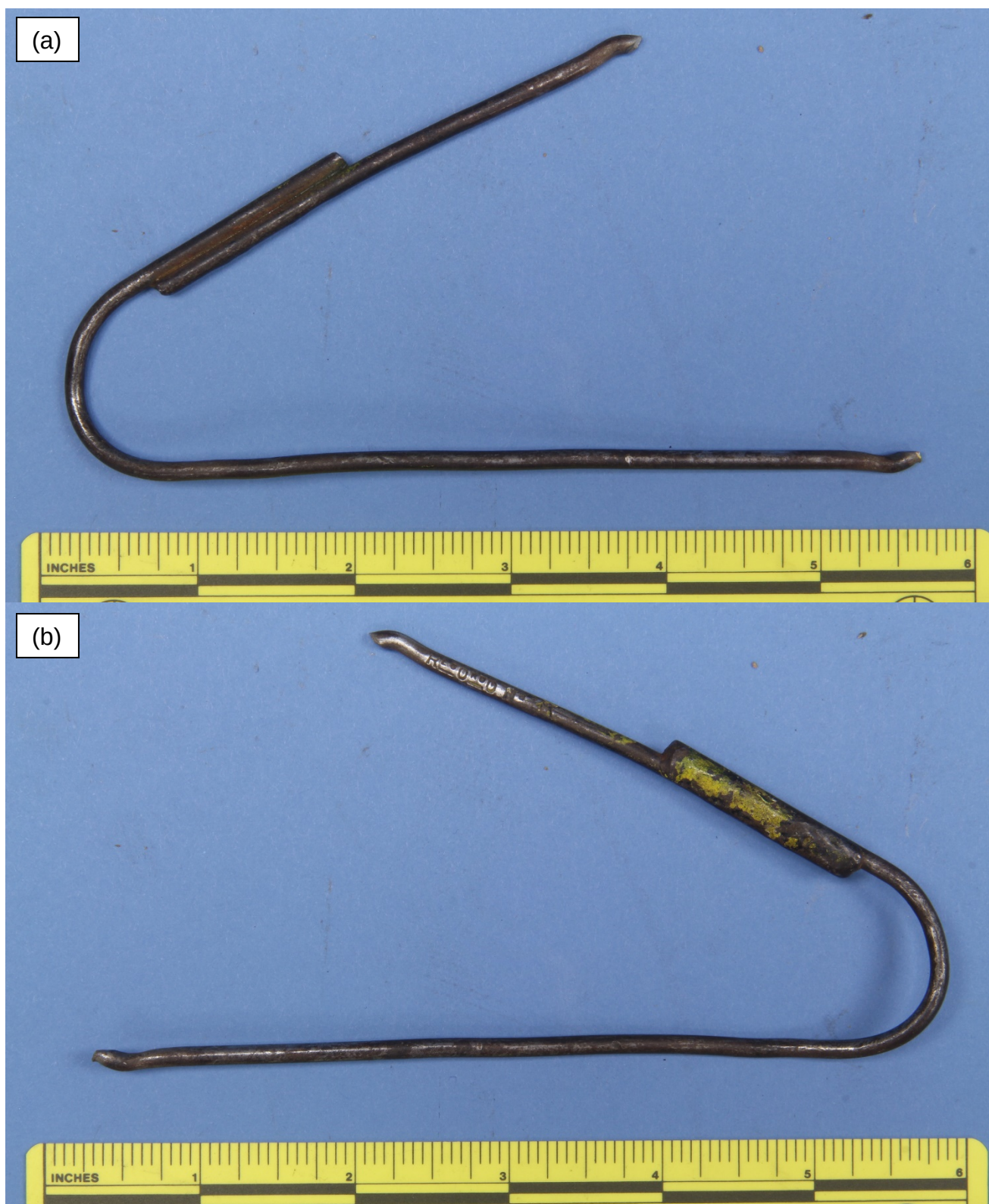
Figure 1 – The fractured wire bracket, viewed from (a) the observe and (b) the reverse side. The bracket had fractured in two places, labeled “flat side” fracture (lower) and “bent side” fracture (upper).
