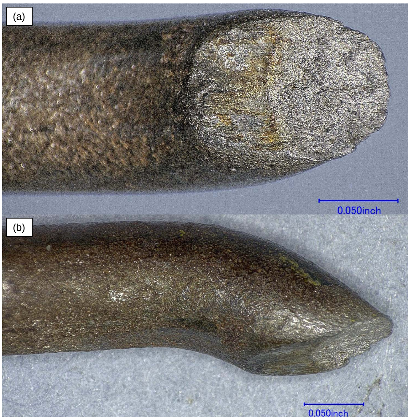
Figure 4 – The bent side fracture (upper fracture in Figure 1) viewed (a) end on, showing two visually distinct regions and (b) from the side.
