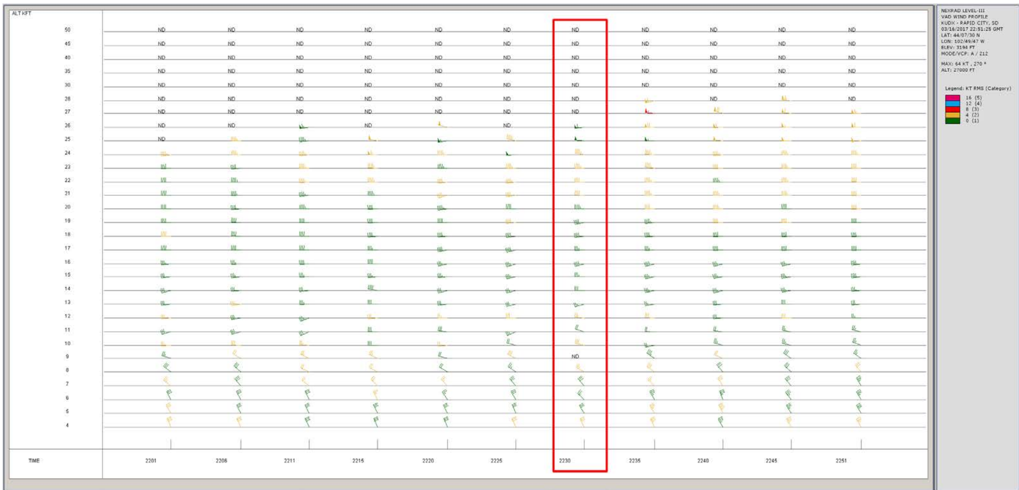
KUDX VAD wind profile for the times surrounding the accident time with the time closest to the accident time surrounded by the red box. Time is in UTC and heights are in 1,000's of feet above msl.
