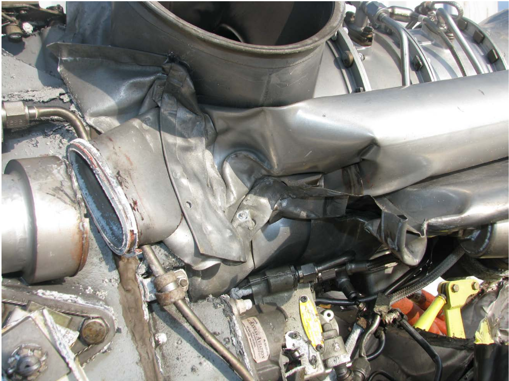
Photo 6 – Main rotor blade strike on the left side of the engine.
