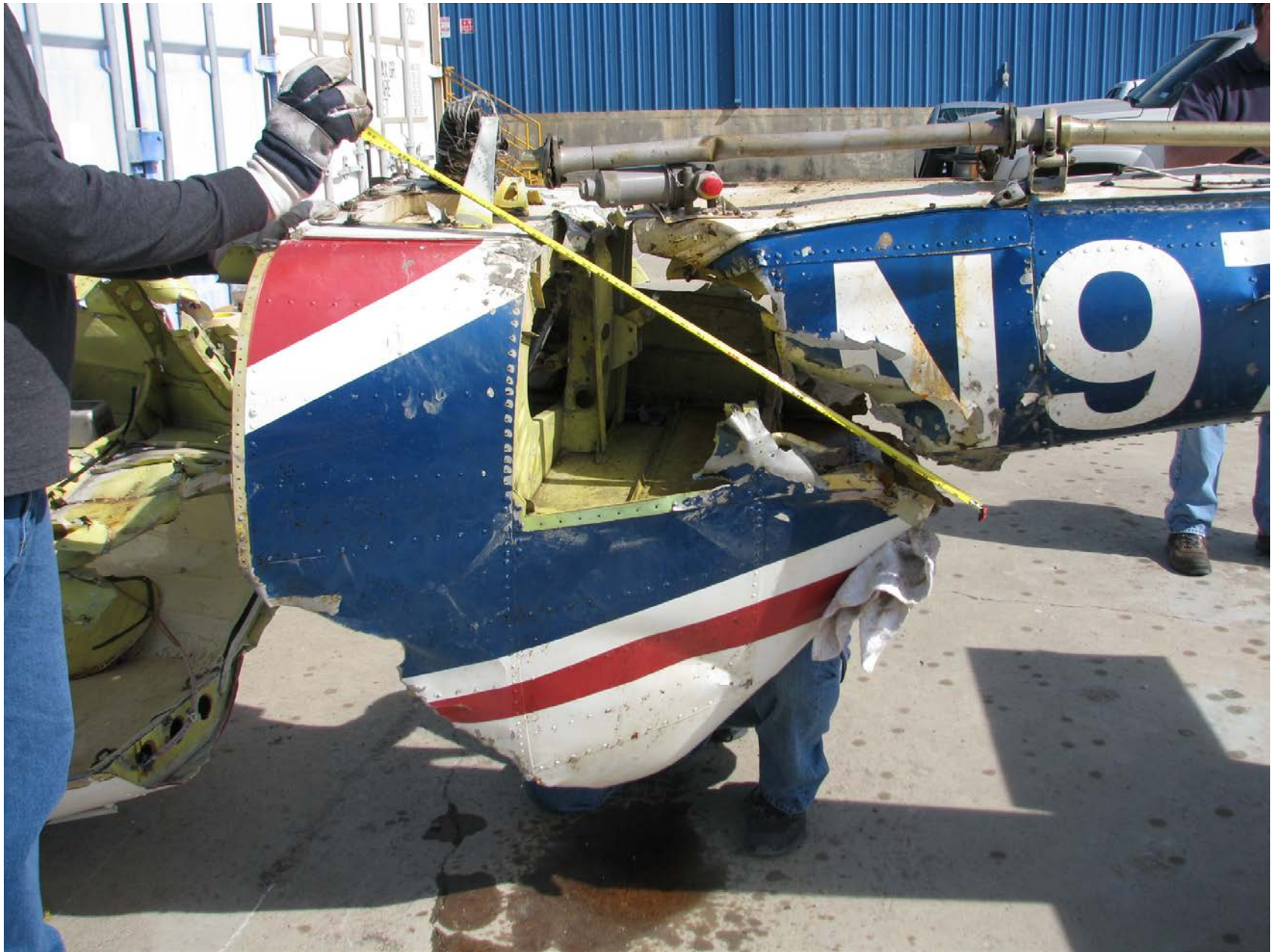
Photo 5 – Measuring the angle of a main rotor blade strike at the aft baggage compartment-tail boom.
