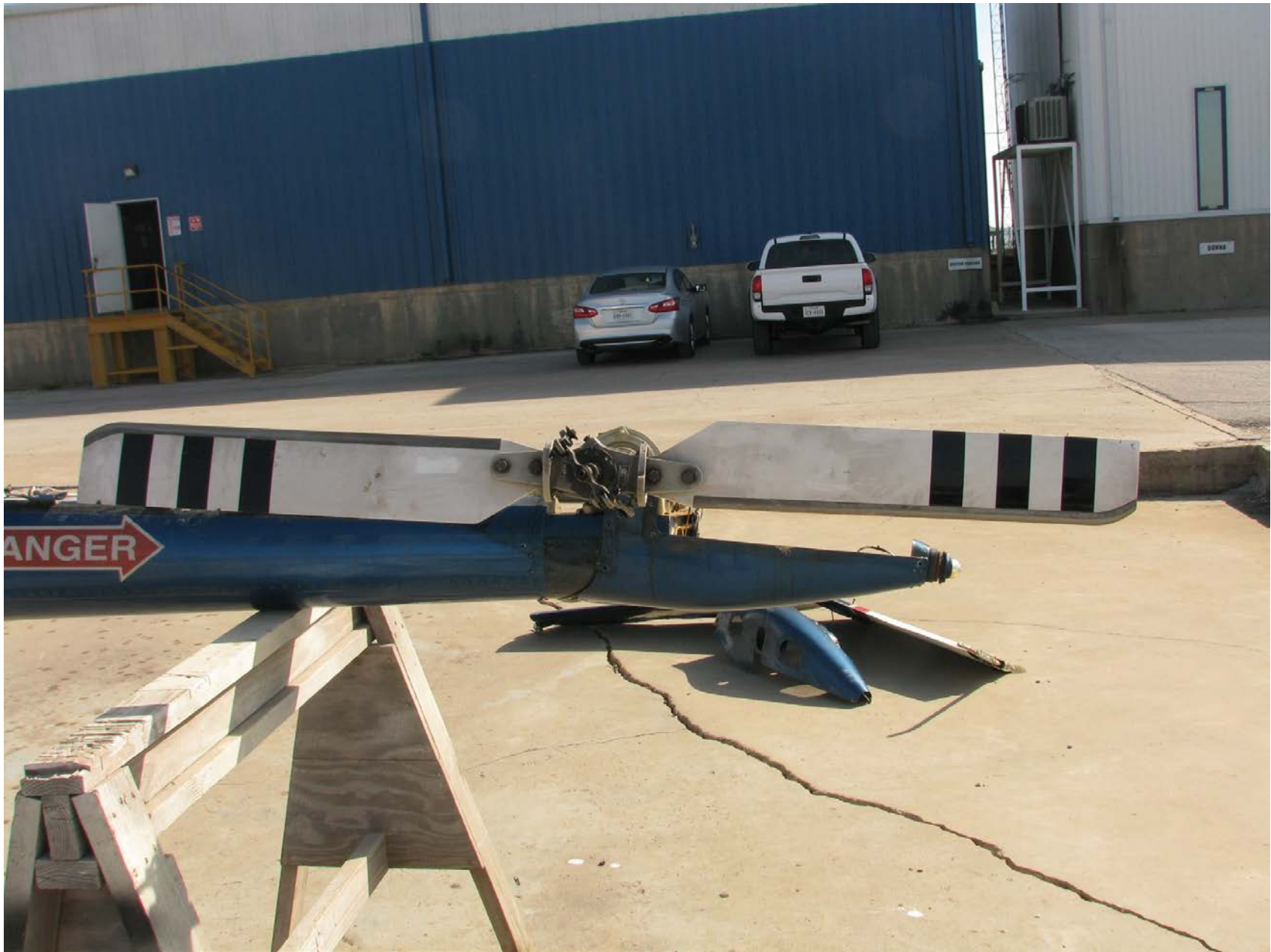
Photo 7 – Aft tail boom, tail rotor hub, and tail rotor blades were undamaged.
