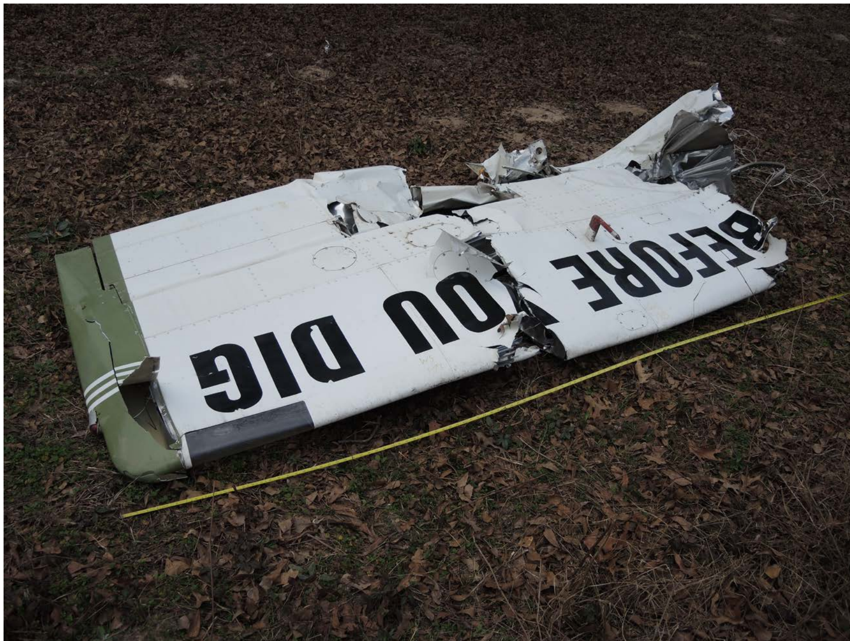
Photo 7 – Underside of Separated Left Wing
