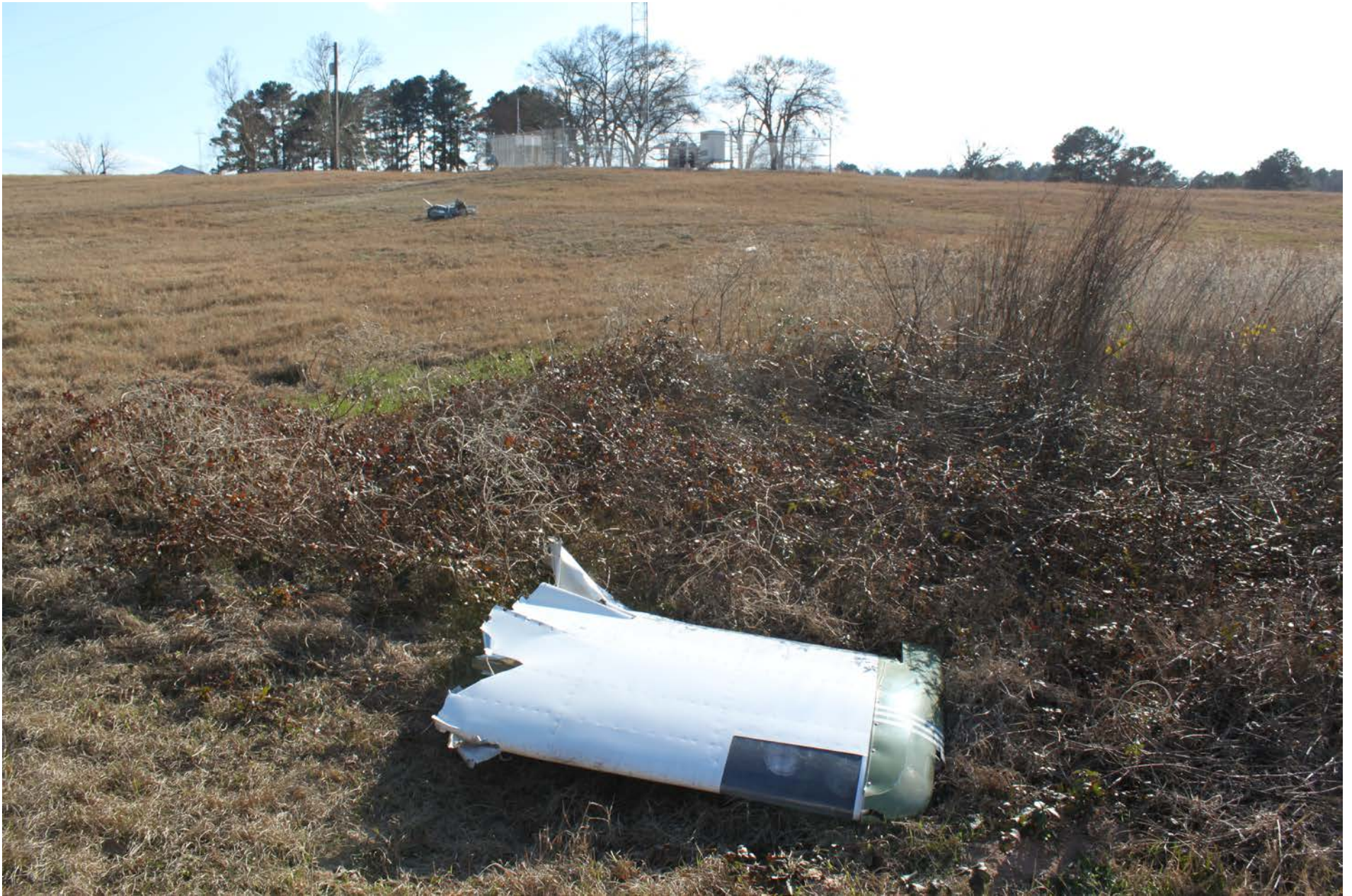
Photo 5 – Section of Separated Left Wing
