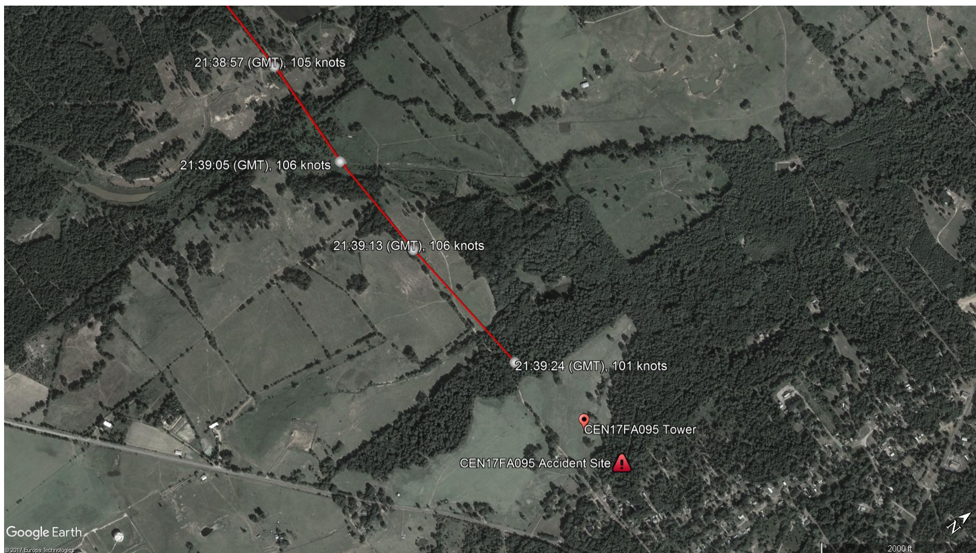
Figure 4. Detail view of the end of the recorded session, including locations for the cellular tower and the accident wreckage
