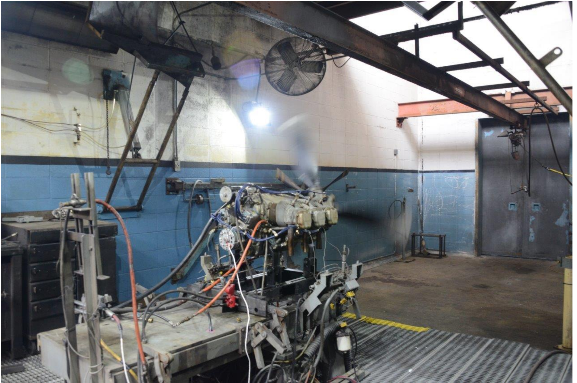
Photo 20 - View of the accident engine operational during an engine run.
