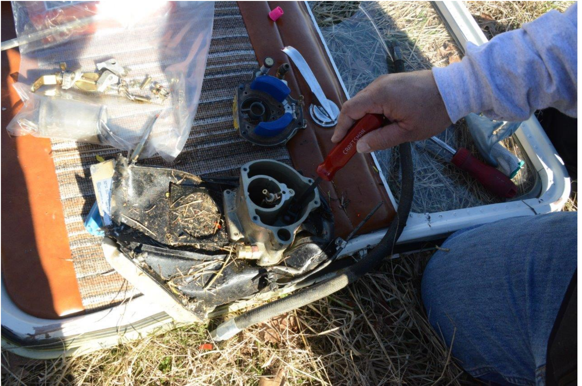
Photo 15 - View of testing for water in the liquid observed in the carburetor bowl.
