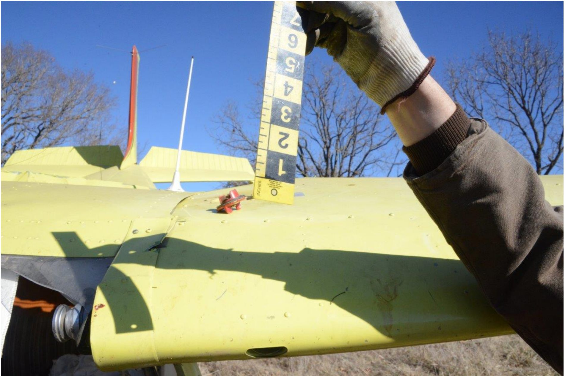
Photo 13 - Fuel level measured in the left wing.
