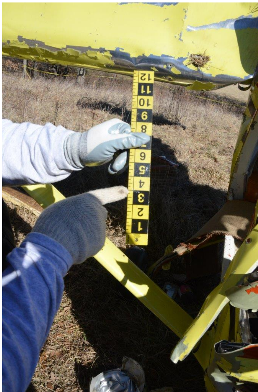
Photo 12 - Fuel level measured in the right wing.
