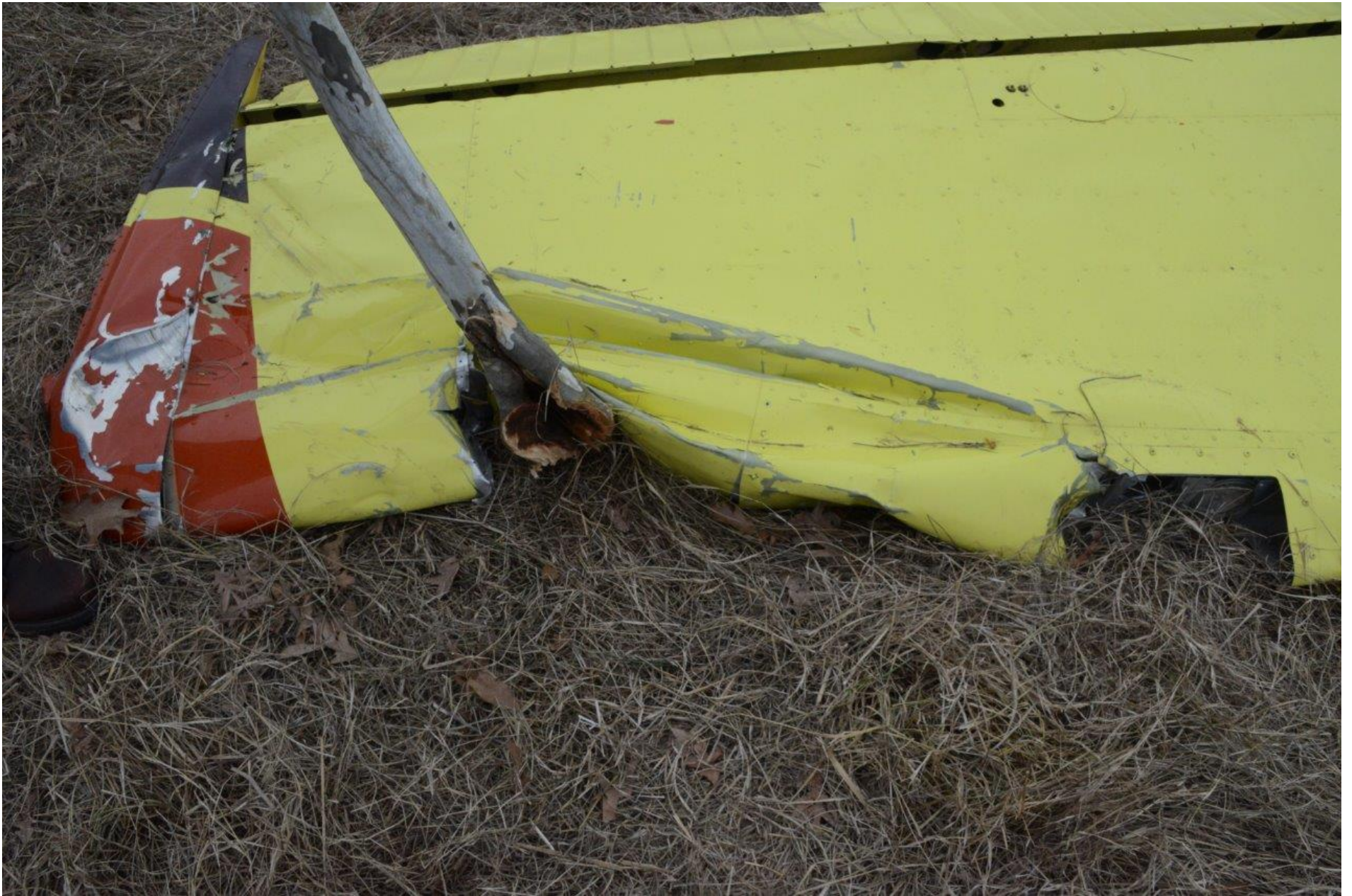
Photo 10 - View of a broken tree limb placed within the semicircular depression on the leading edge of the left wing.
