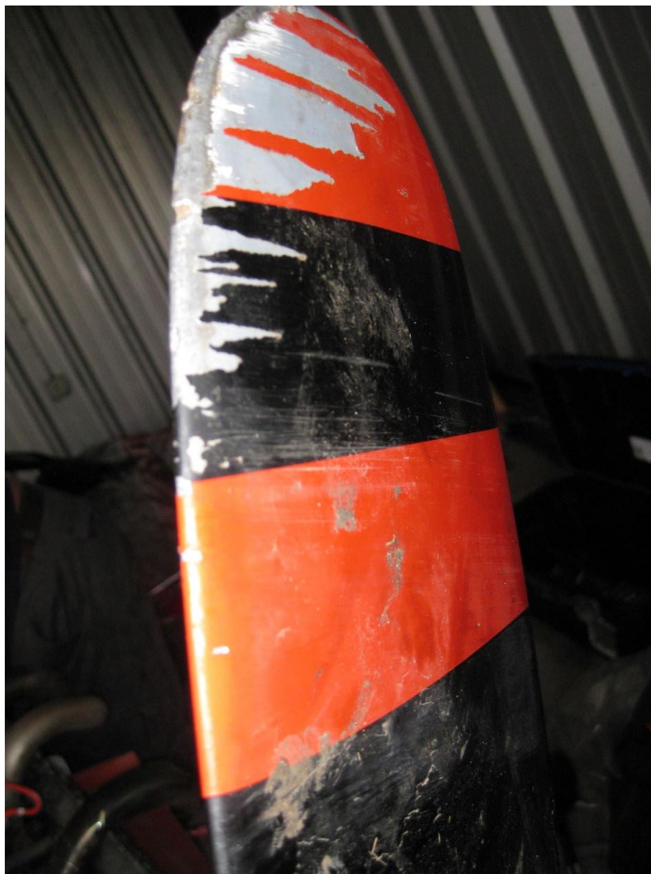
Photo 13 – View of some blade tip damage
