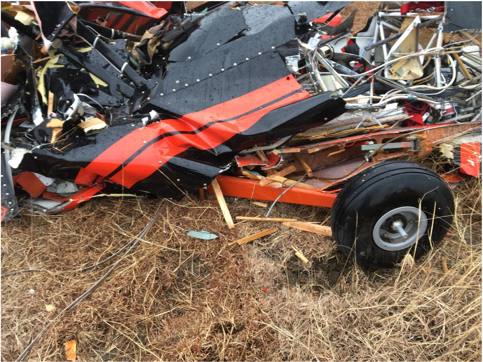
Photo 9 – View of the left main gear collapsed to the rear
