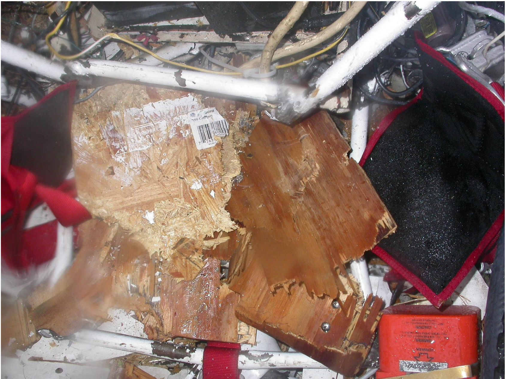
Photo 11 – View of the fractured plywood floorboards under the rear pilot's seat
