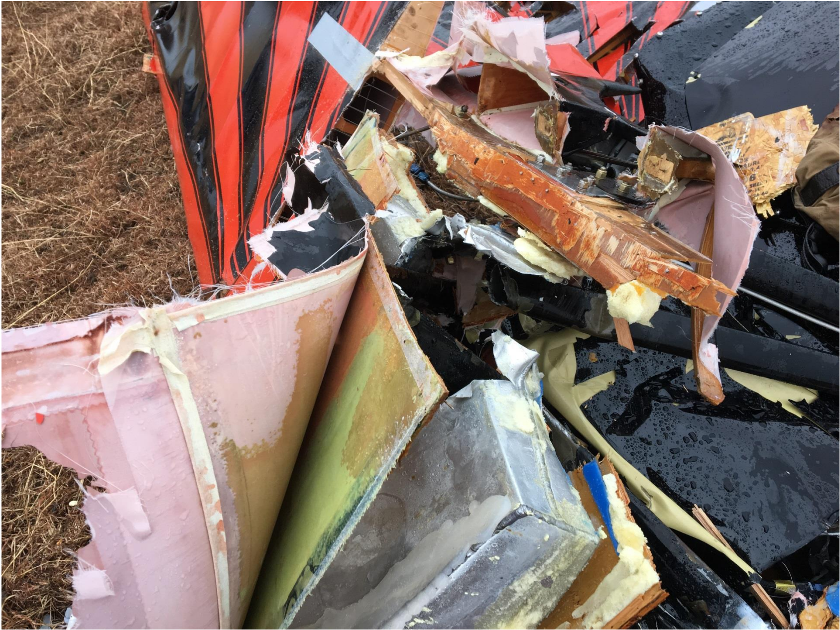
Photo 6 – View of the rear wing spar separated from the middle wing section
