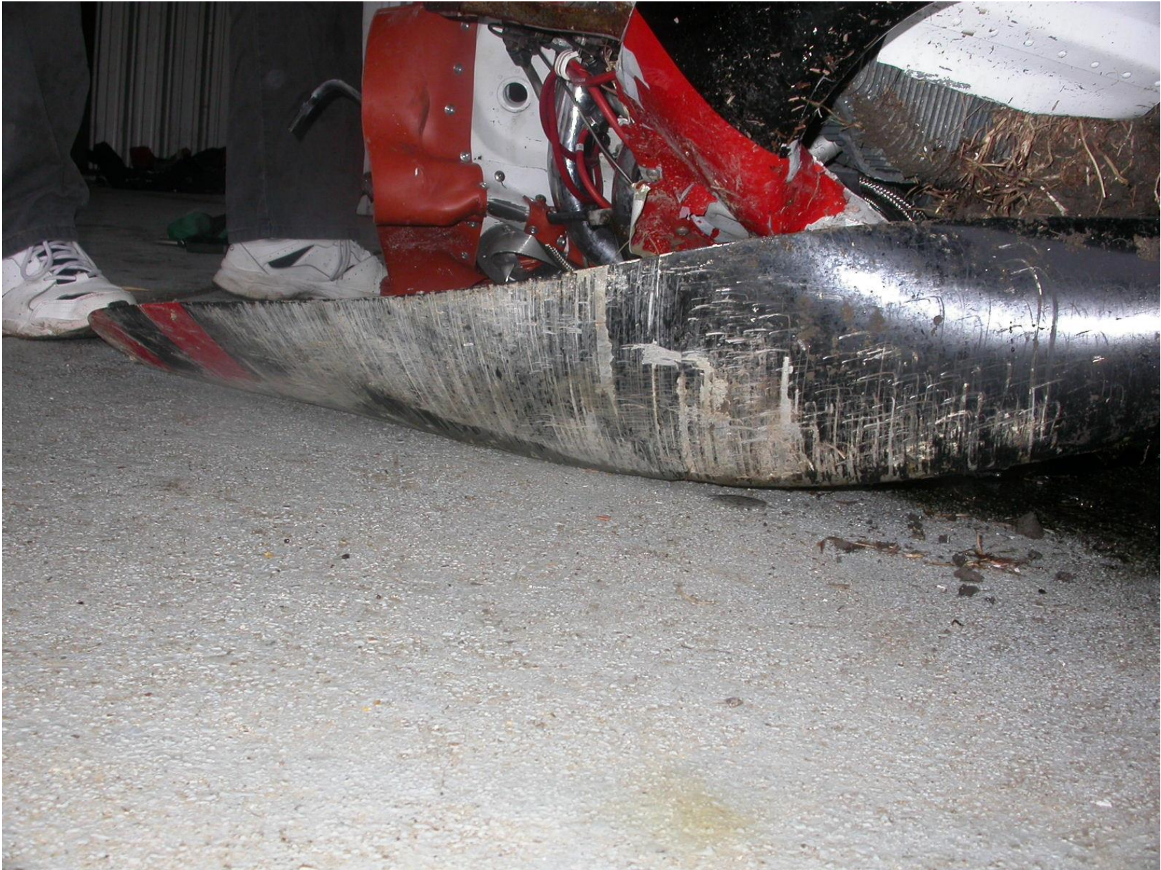
Photo 14 – View of the damage to the other blade
