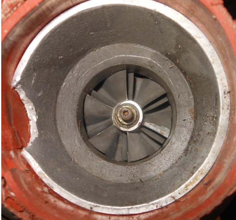
Photo #16 (Left Turbocharger Compressor Inlet)
