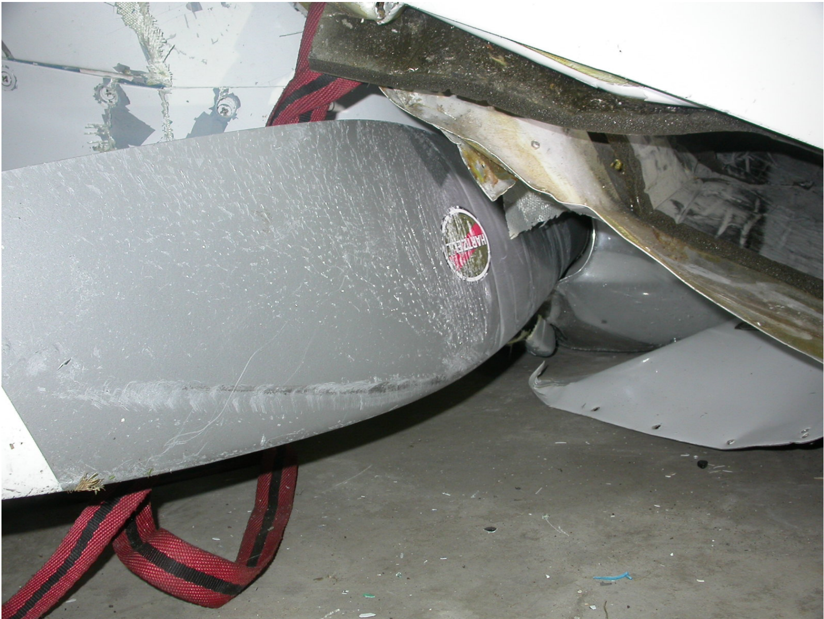
Photo 11 – View of propeller blade with scuff mark on the chamber side of the blade
