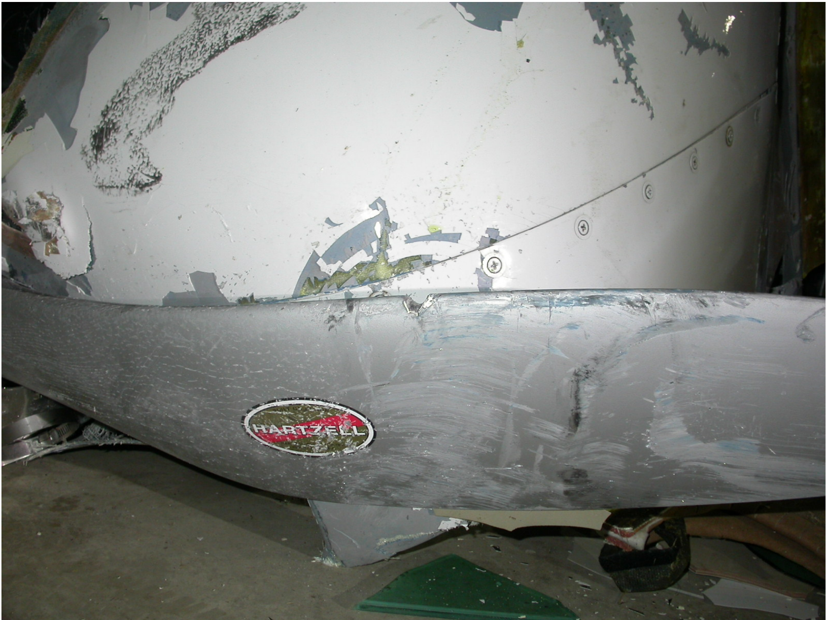
Photo 10 – View of propeller blade with a gouge in the leading edge
