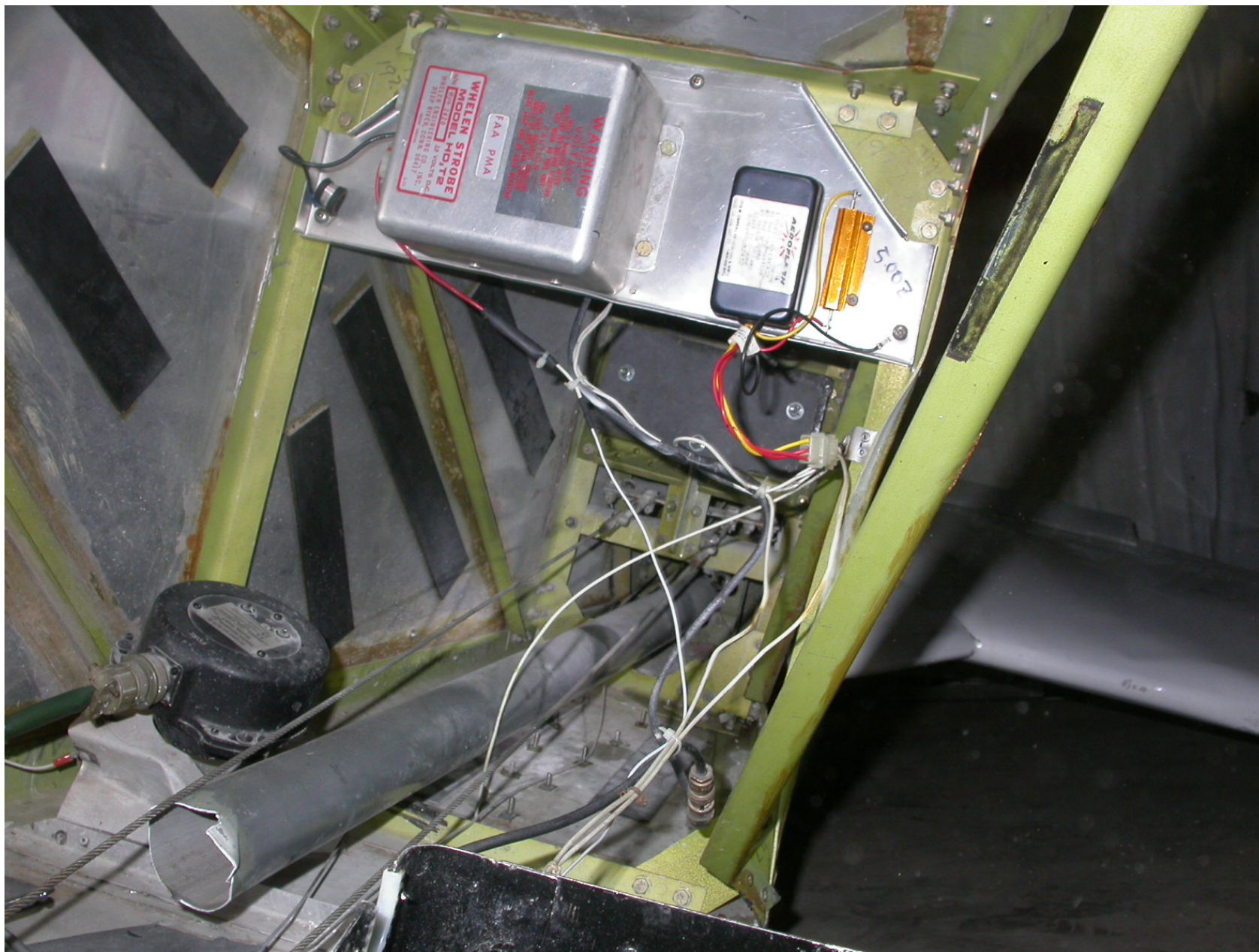
Photo 13 – View of rudder cable and elevator control tube
