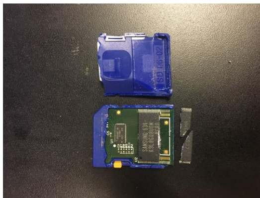
Figure 2. Photo of damaged SD card.
