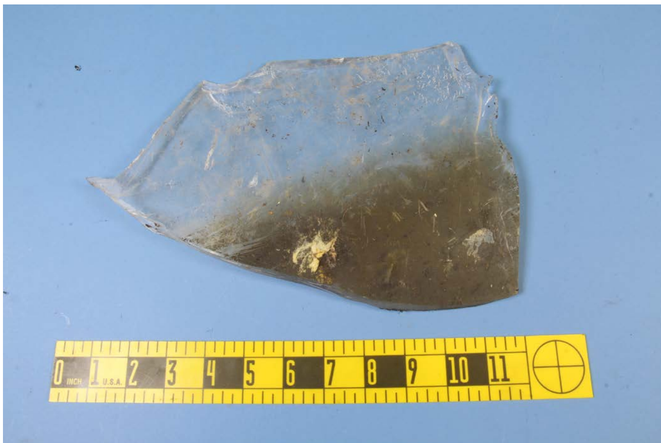
Figure 3: Portion of windshield with soot staining.
