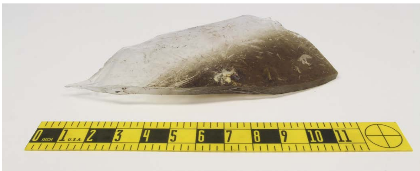
Figure 4: Clean fracture surface adjacent to soot stained exterior surface.
