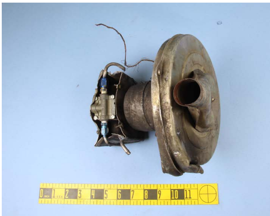
Figure 5: Combustion air blower.
