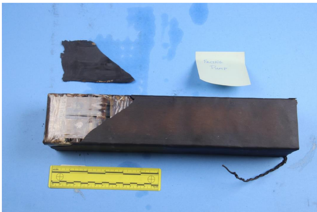
Figure 12: Cells visible within battery pack.
