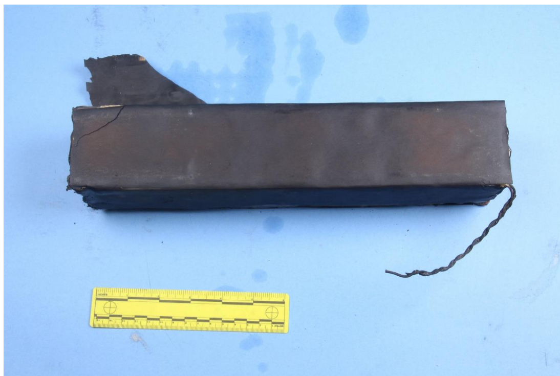
Figure 11: Battery pack with insulating paper.
