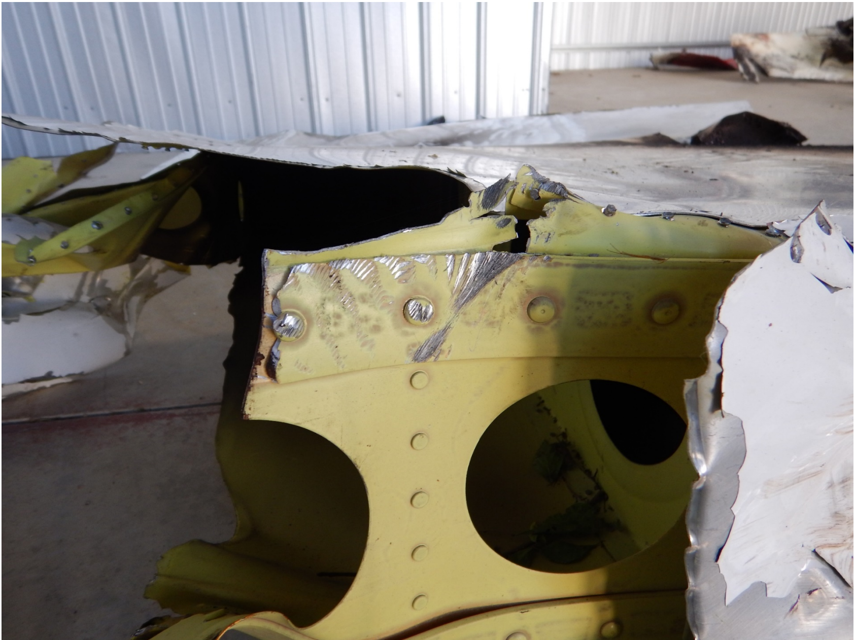
Photo 13 – Outboard Section Right Wing Spar
