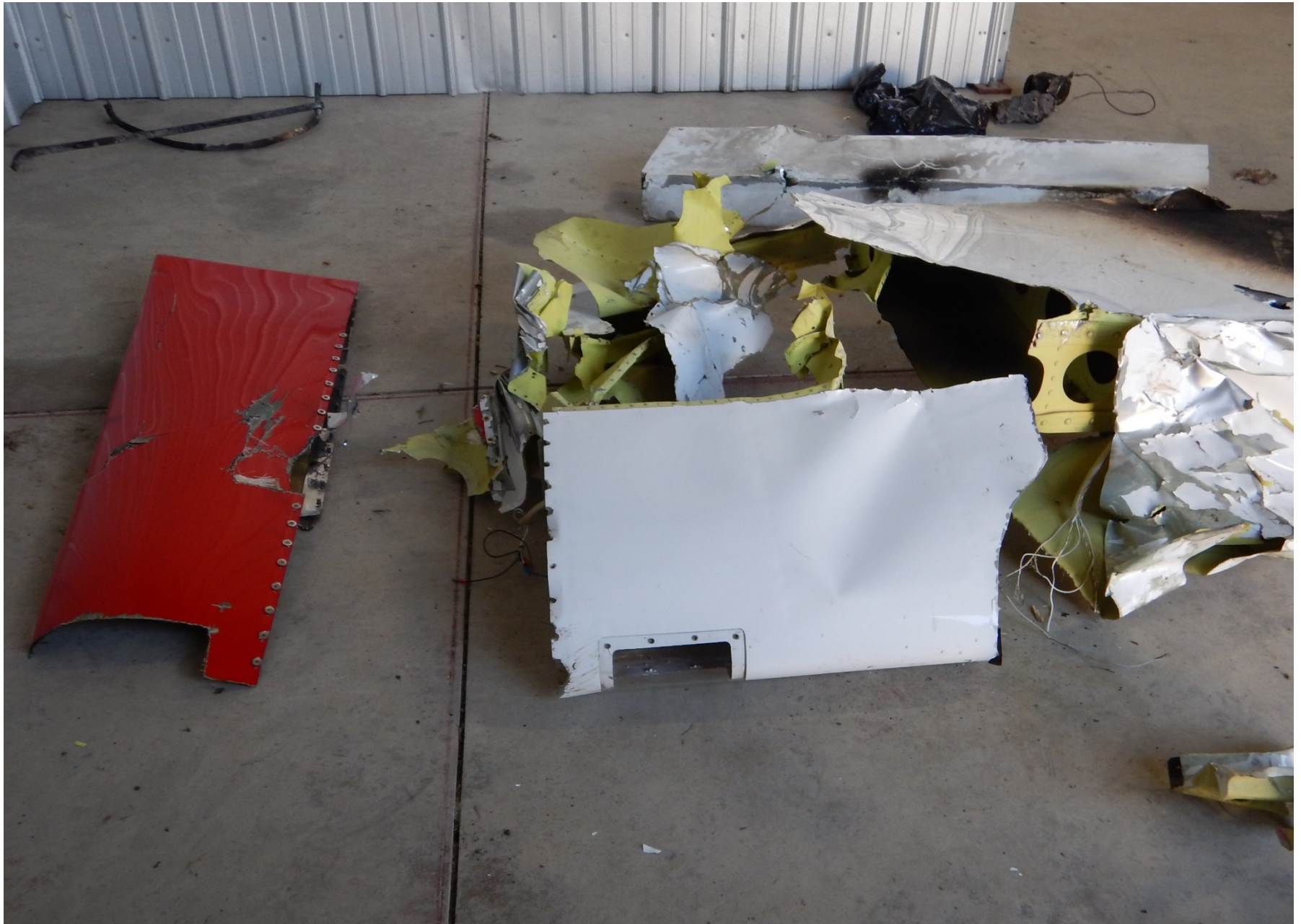
Photo 10 – Outboard Section of Right Wing
