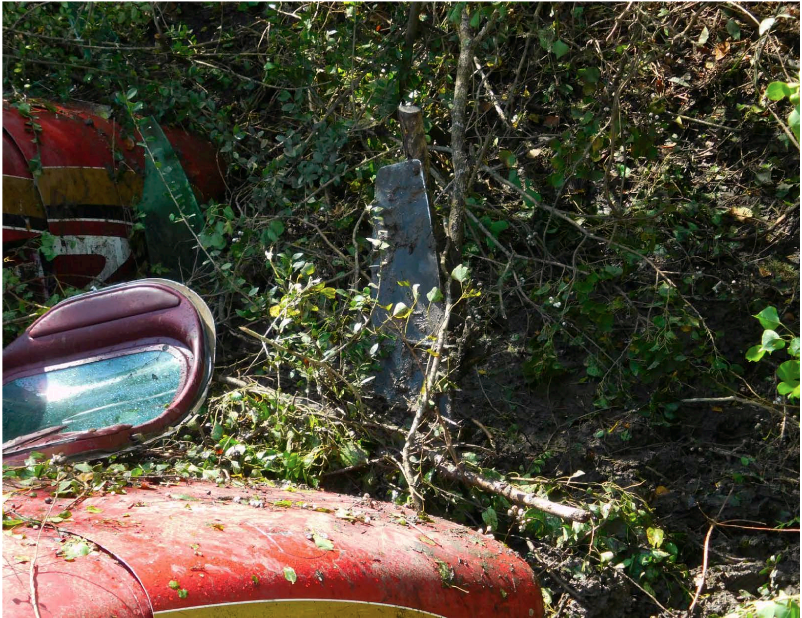
Photo 7 – Left engine and propeller.
