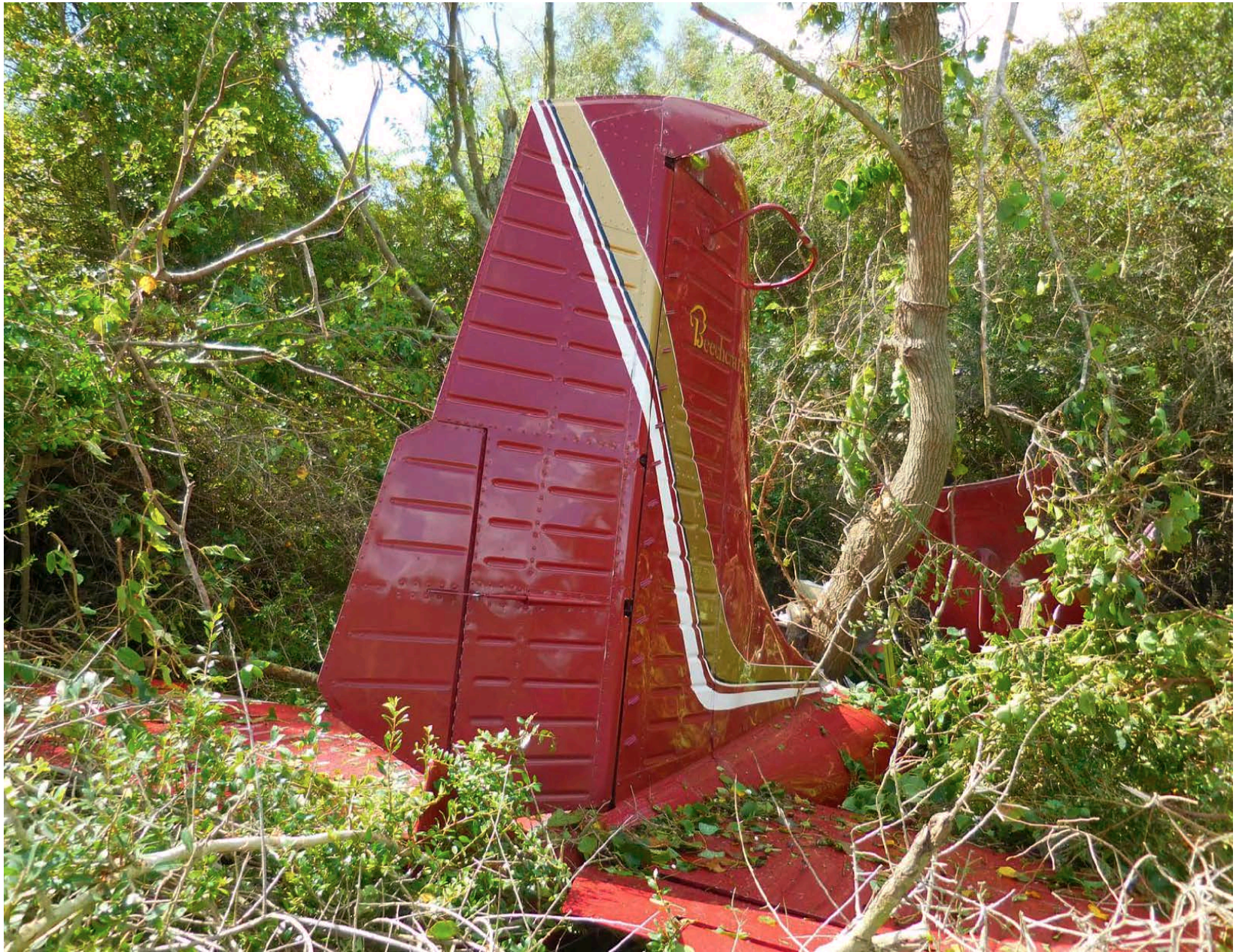
Photo 5 – The empennage. Note left deflection of the rudder.
