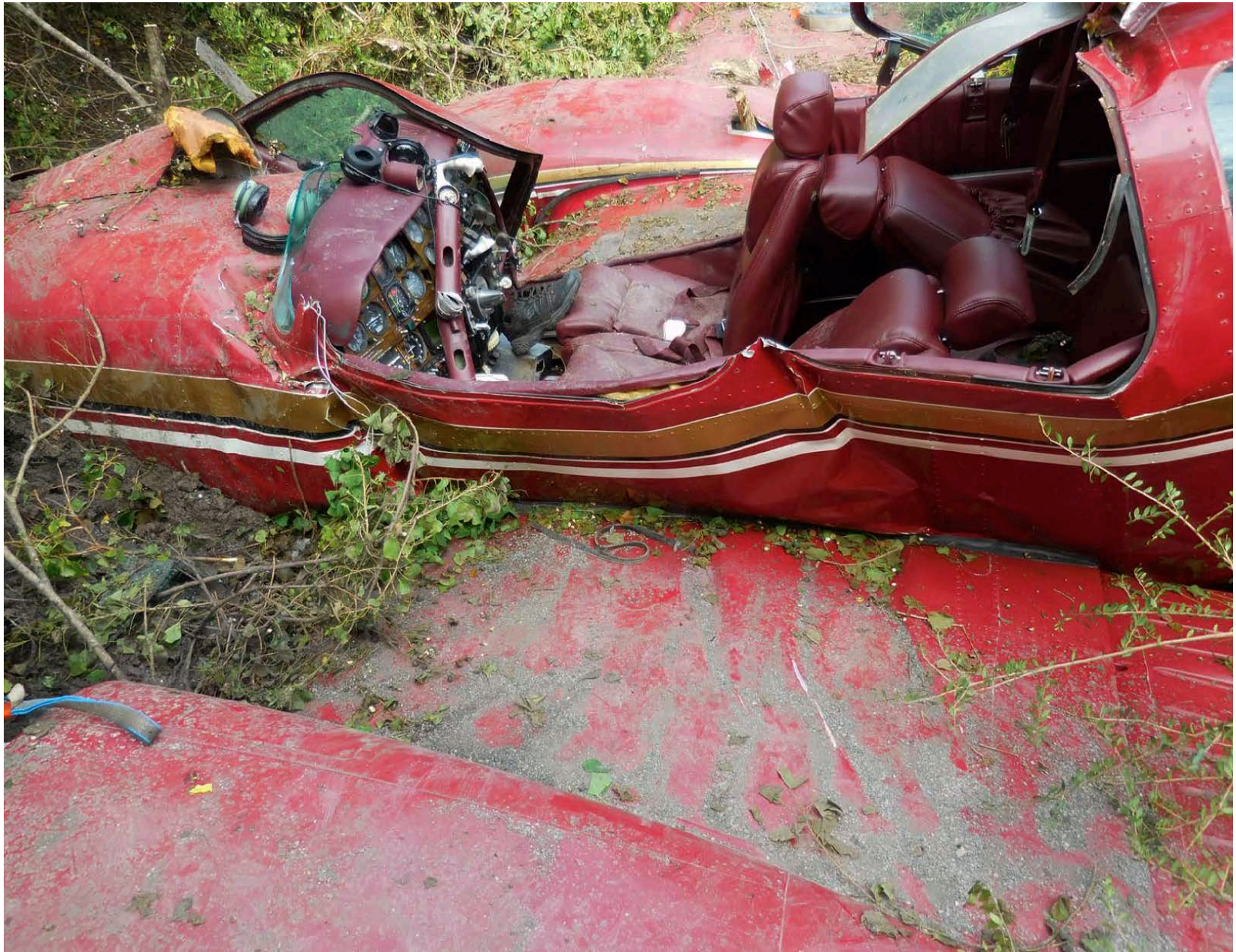
Photo 6 – Left side of fuselage. Note creases at instrument panel and pilot's seat. Top to bottom, left to right.
