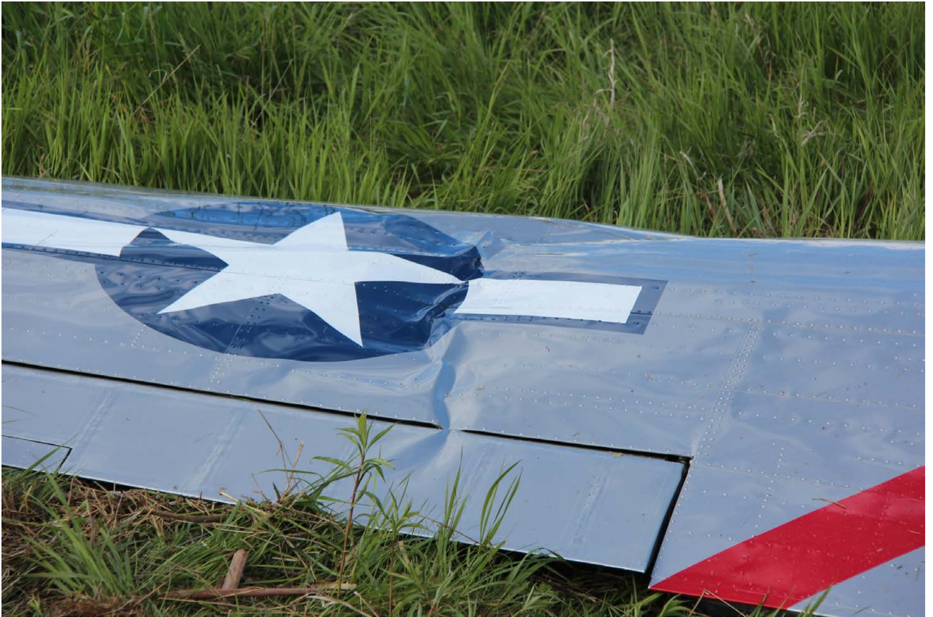
Photo 3 - Close-up of damage to left wing.
