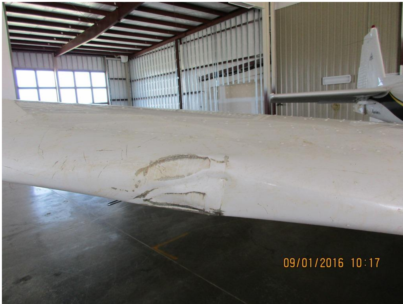
Photo 1 – Damage to the left wing (FAA photo)
