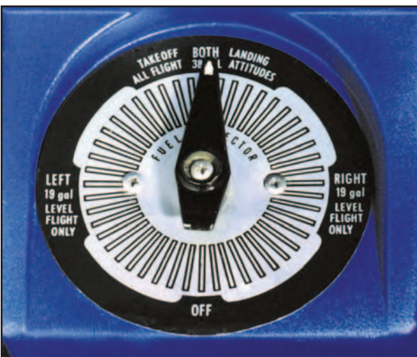
Figure 5-16. Fuel selector valve.
