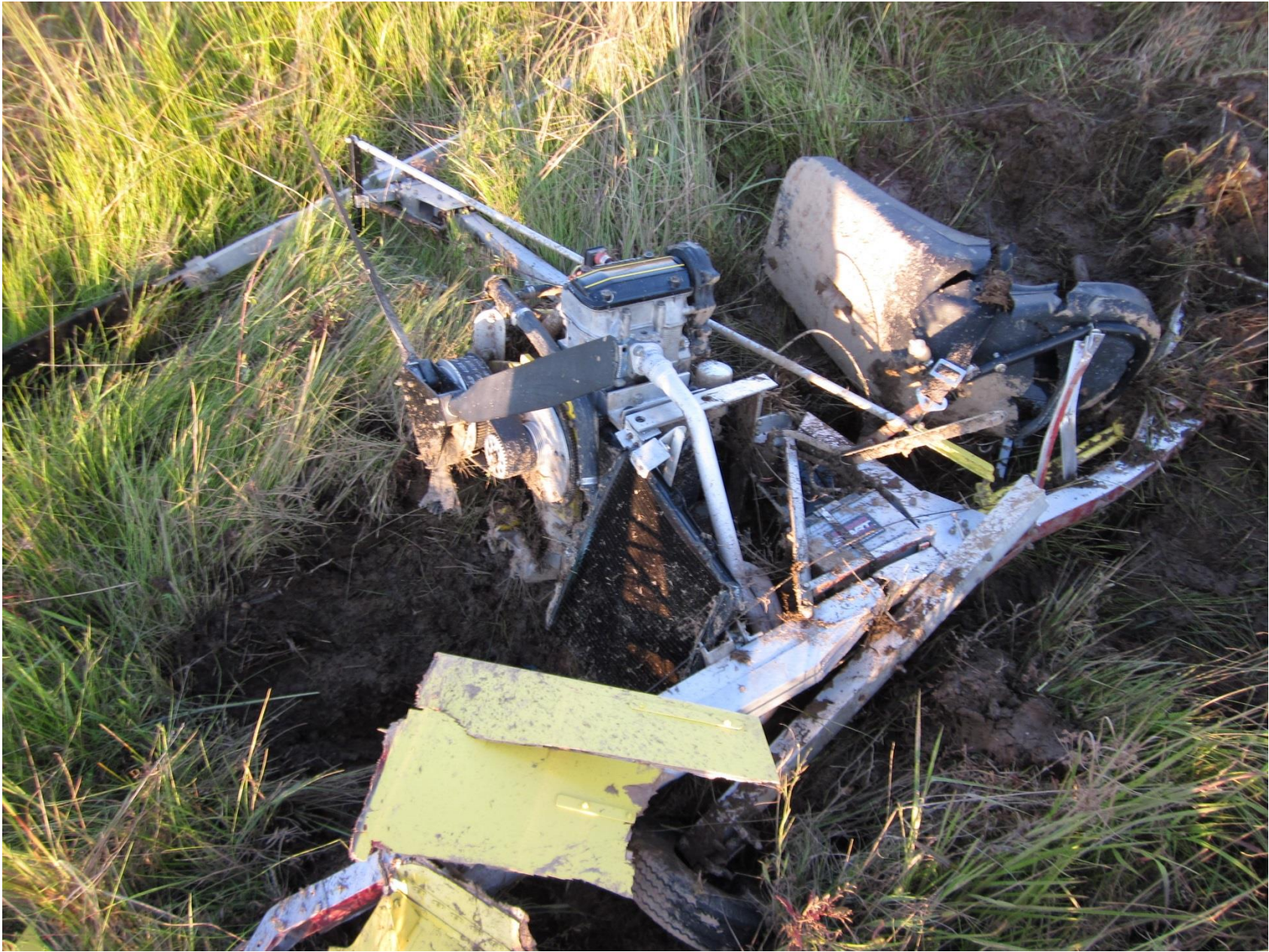
Photo 1 – The unregistered gyroplane. Note absence of ground scars, only impact crater, consistent with no forward velocity
