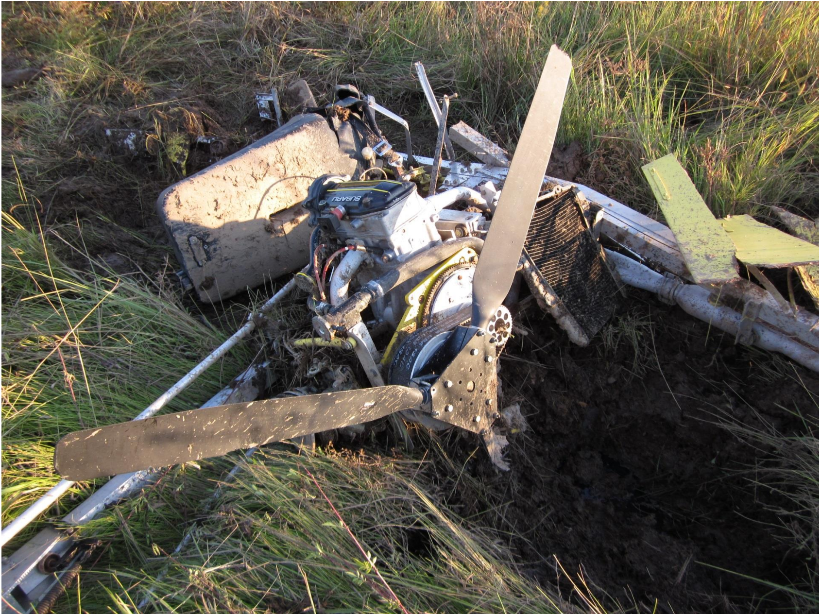
Photo 2 - Rear view of gyroplane, showing Subaru engine and pusher-type propeller.
