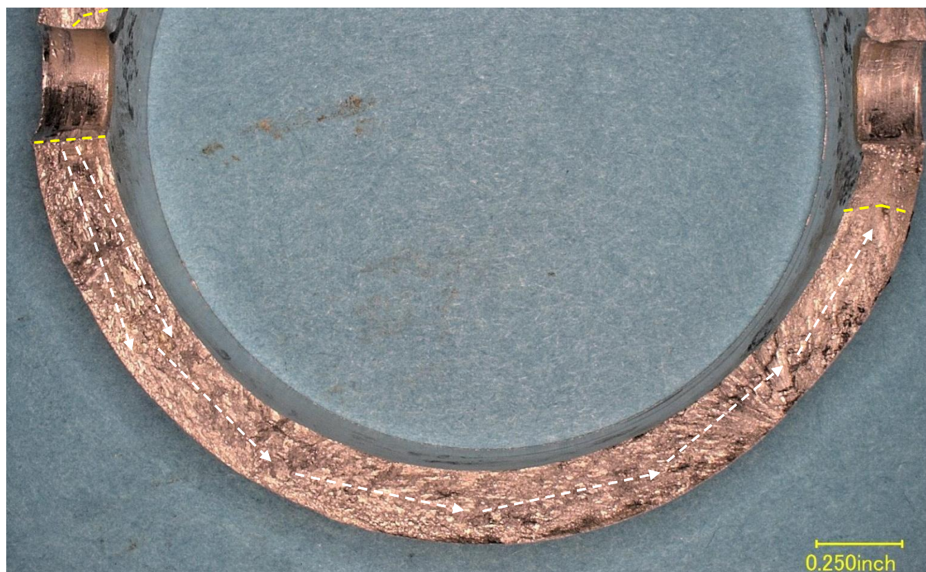
Figure 6 – Closer view of the flat portion of the outboard fracture surface of the cuff (from Figure 5), after disassembly and cleaning. The progressive portions of the fracture surface are outlined and the crack direction is annotated.
