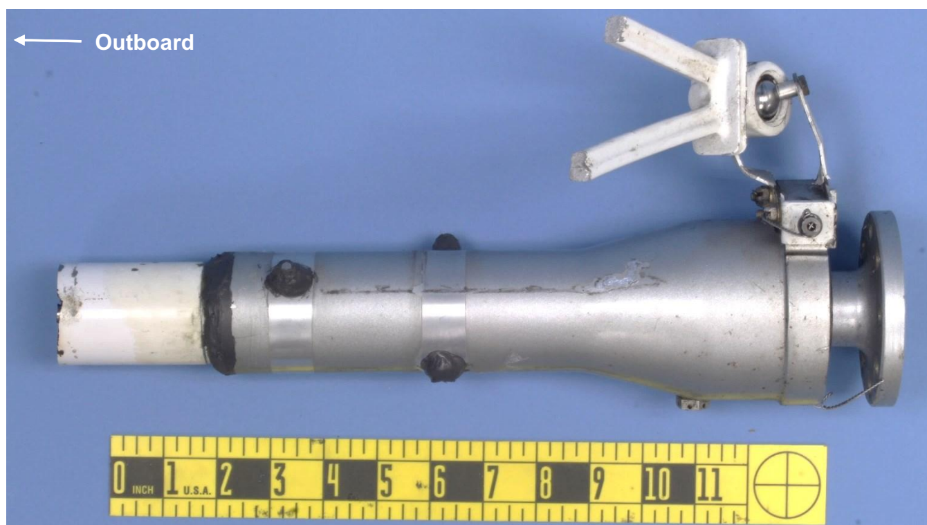
Figure 2 – The section of the intact control rotor cuff, opposite the fractured one in Figure 1, as received.
