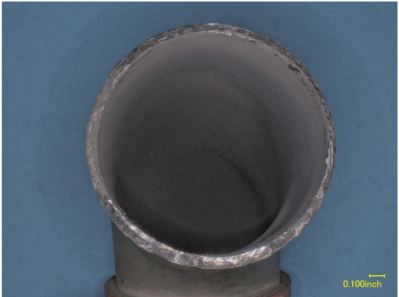
Figure 4 – Closer view of the tube side fracture surface.
