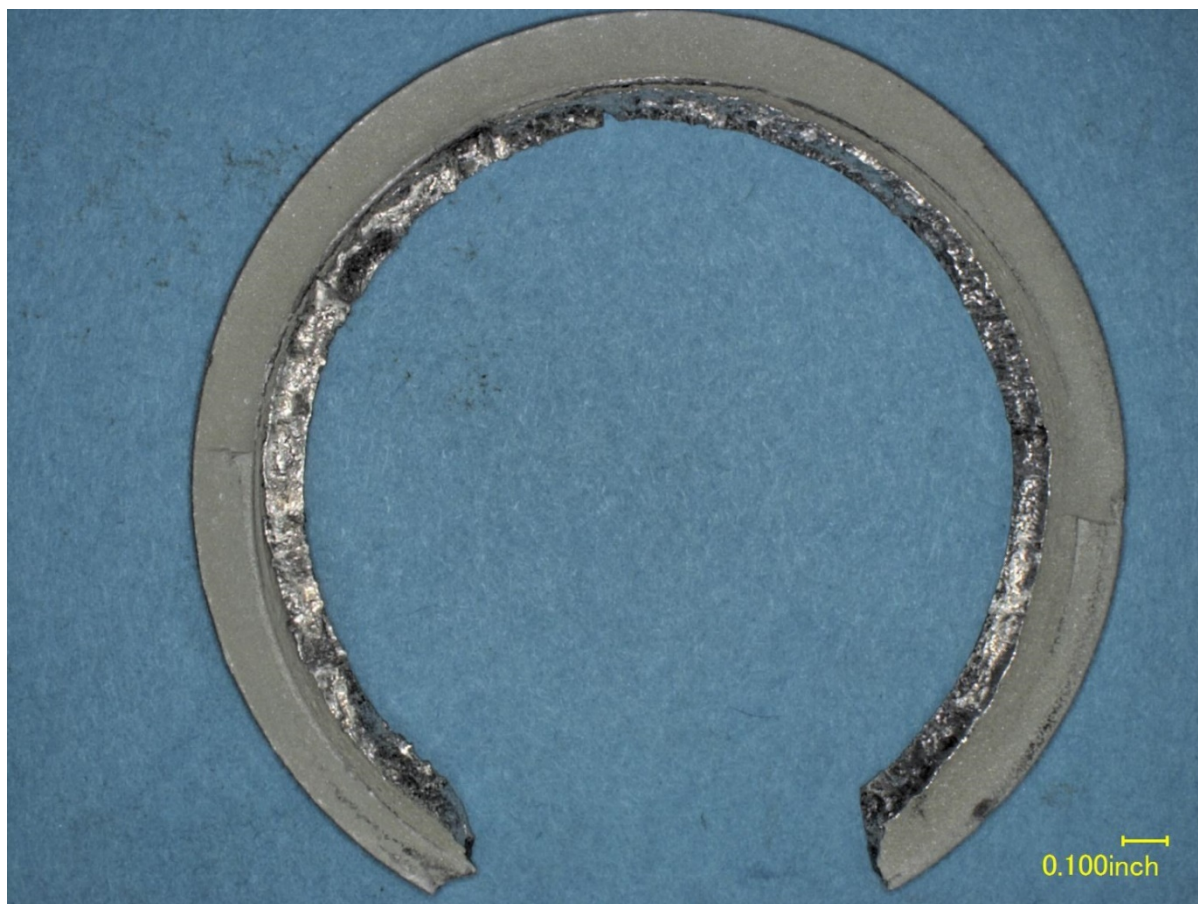
Figure 6 – The fracture surface of the fractured tube flange.
