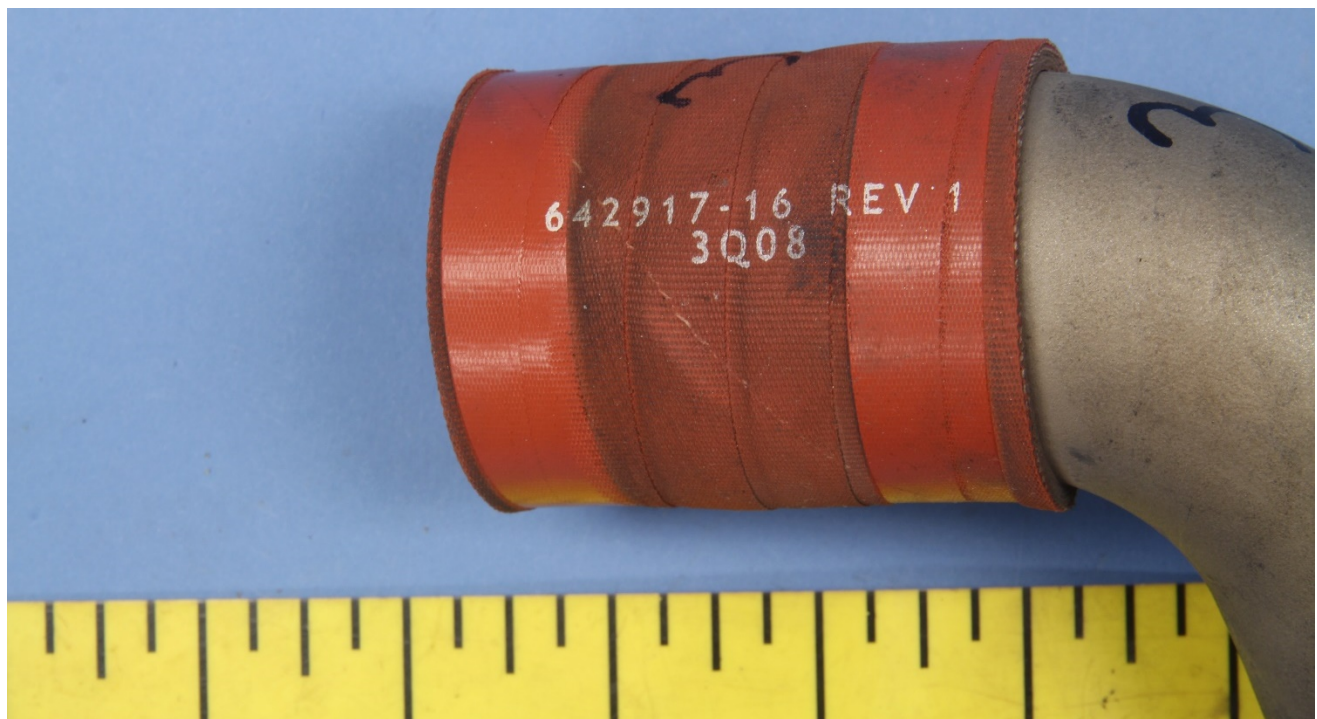
Figure 2 – Markings on the orange rubber connector on the opposite side of the induction tube.
