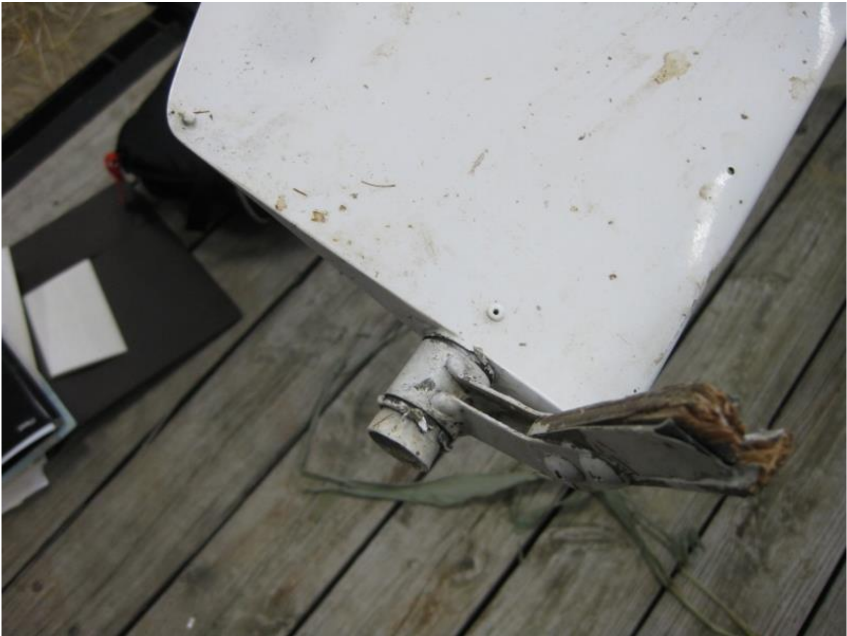
Photo 18 – View of the broken outboard left wing flaperon attach point
