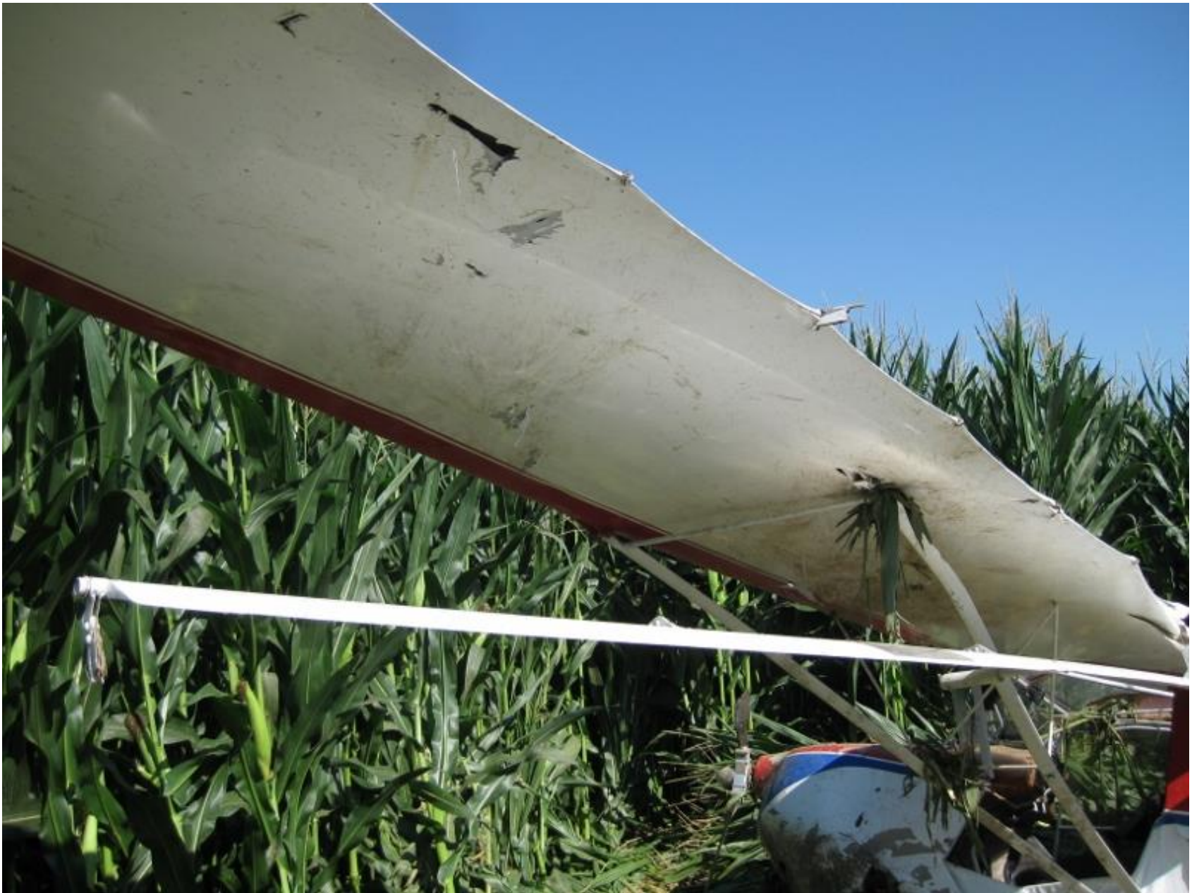
Photo 4 – View of the left wing and broken flaperon attach points
