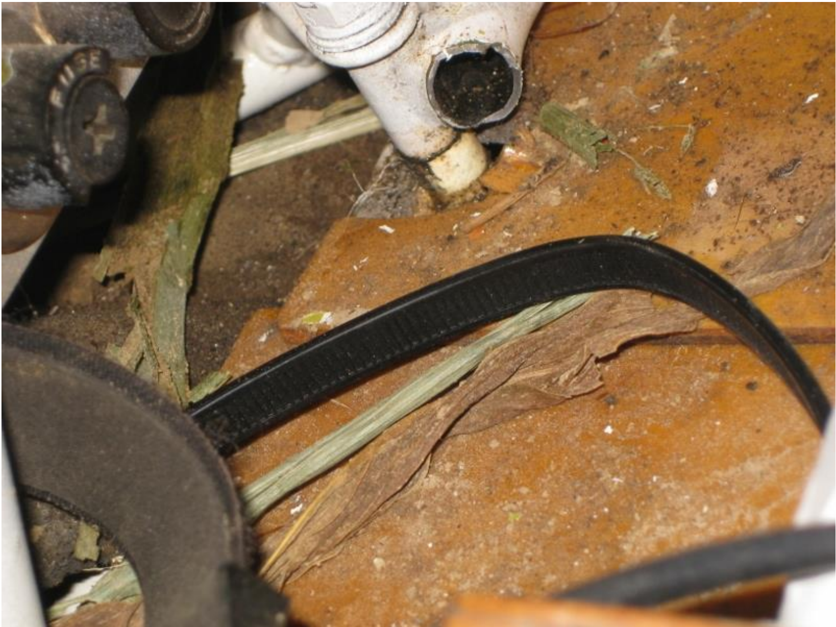
Photo 14 – View of the fractured flaperon control tube
