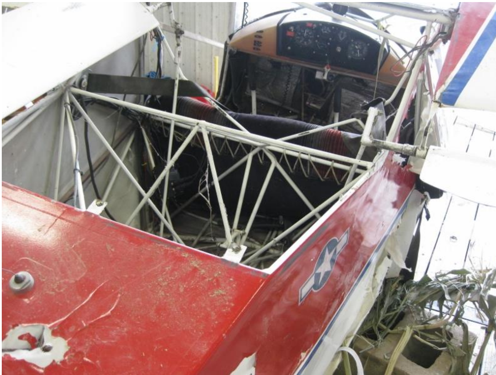
Photo 16 – View of the control tube attachment to the left flaperon
