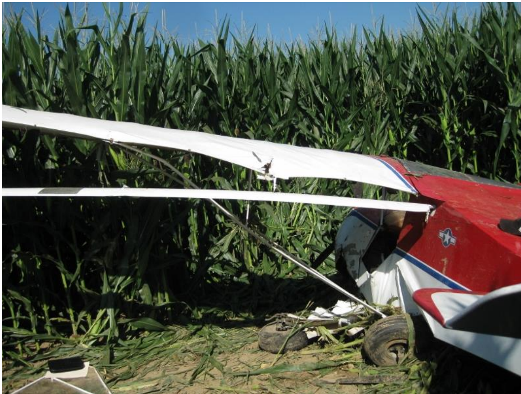
Photo 5 – View of the left wing and broken flaperon
