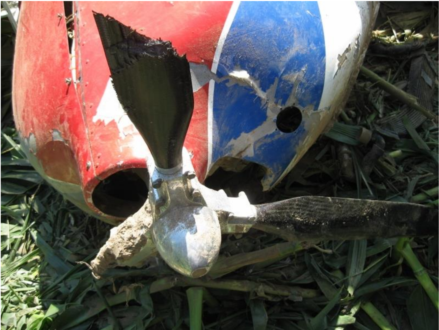
Photo 9 – View of the broken propeller blades at the accident site
