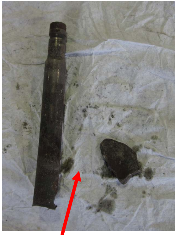
These pieces were found in the left side muffler
