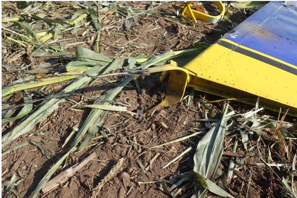
Deformation of the rudder control horn
