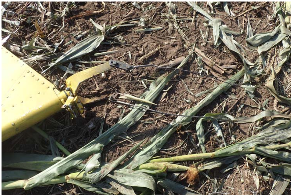
Rudder horn with separated cables
