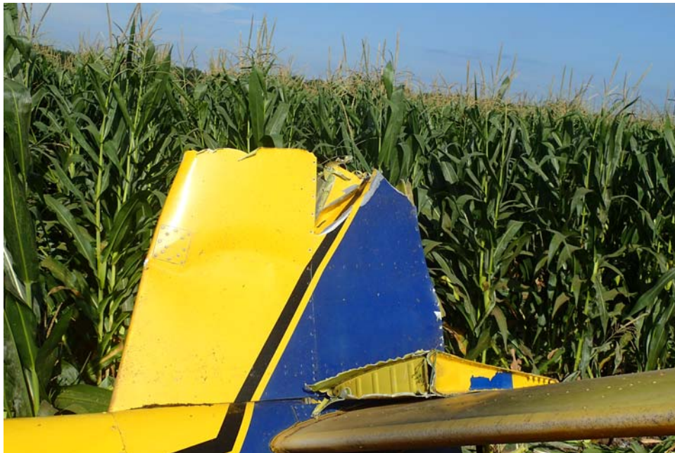
Damage to the vertical fin
