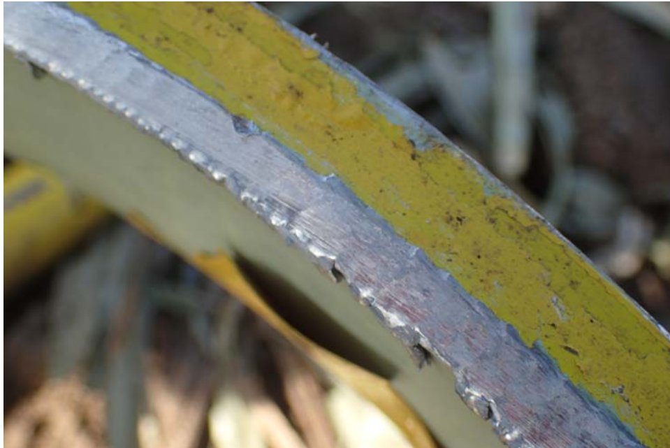
Detail of the bar showing chamfered edge
