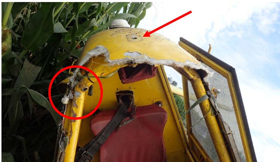
Detail of canopy damage, wire contact damage (red circle), and missing antenna (red arrow)
