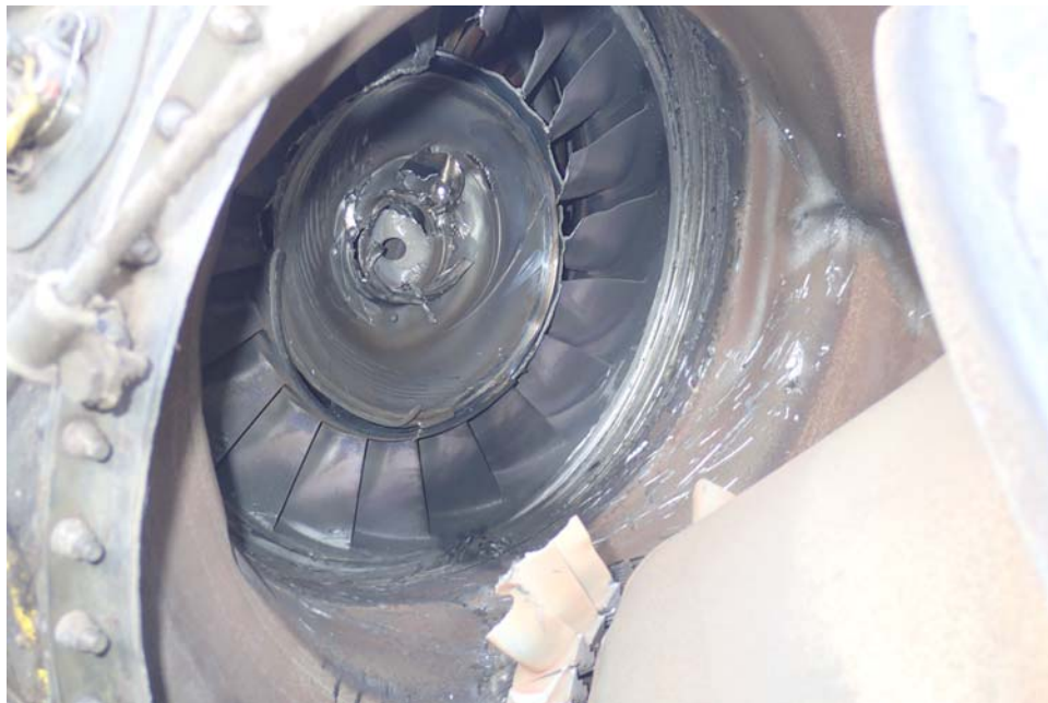
Detail of Engine Interior (looking aft through the separation at the "C" flange)
