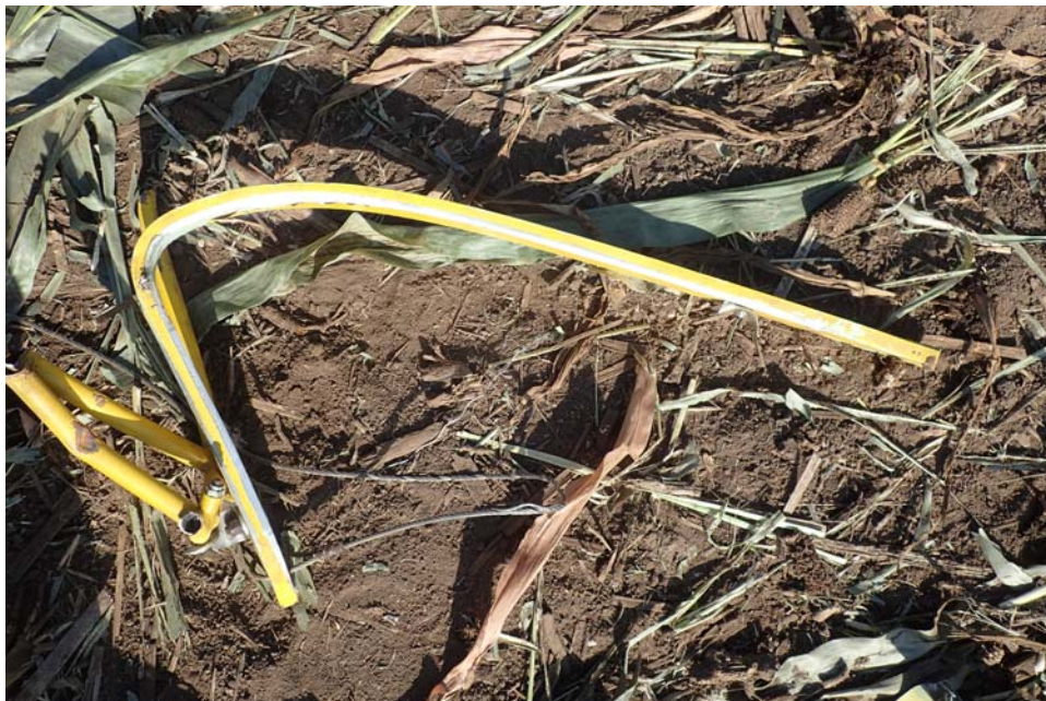
Aluminum bar as found (overturn structure and cable attached)
