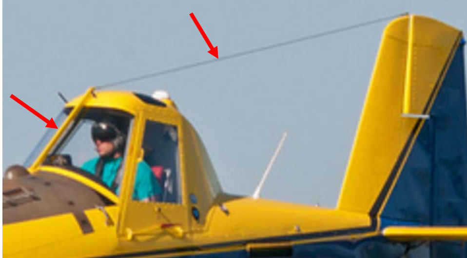
Typical AT-402 showing aluminum bar and deflector cable
