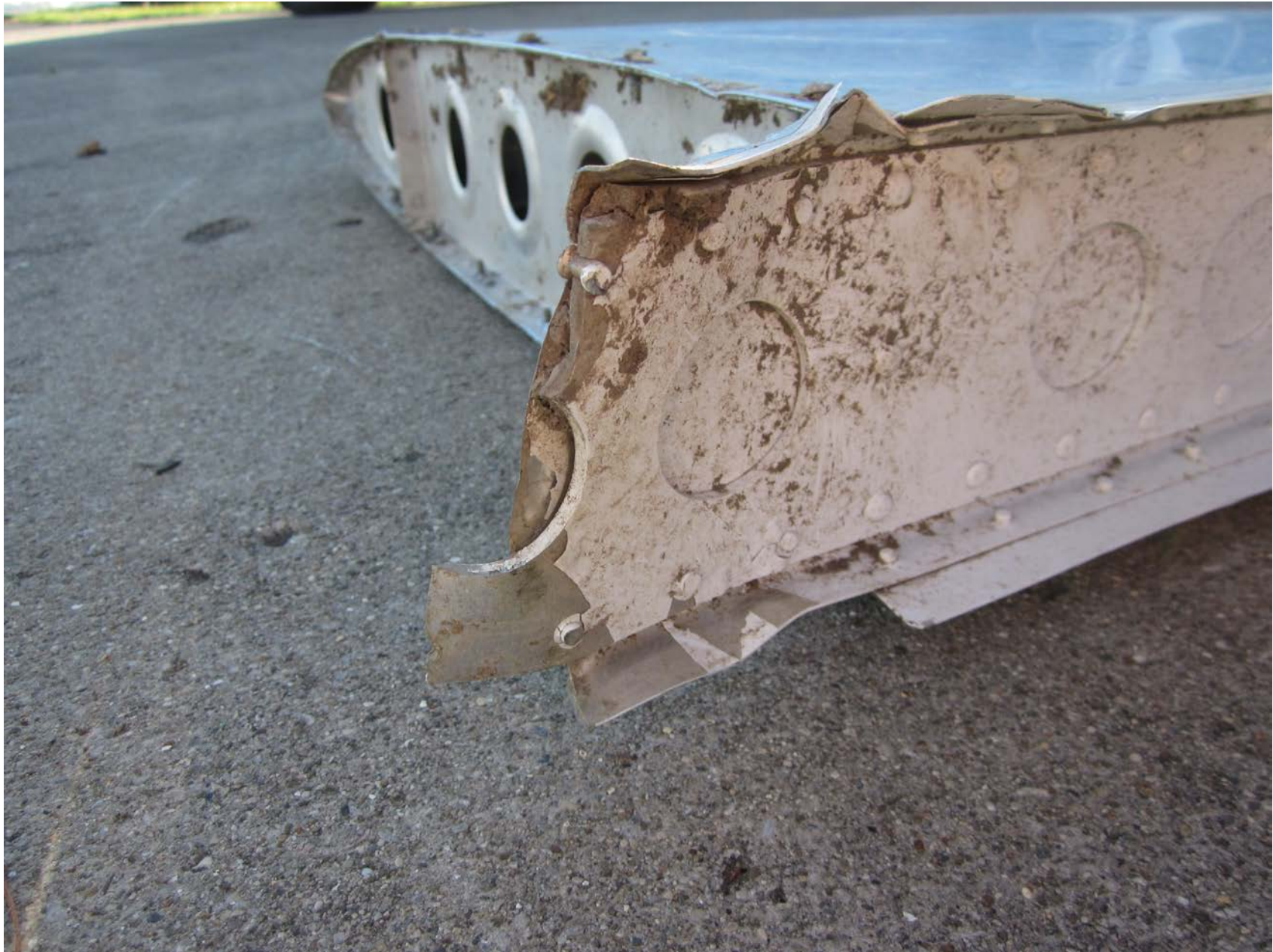
Photo 5 – Vertical stabilizer spar
