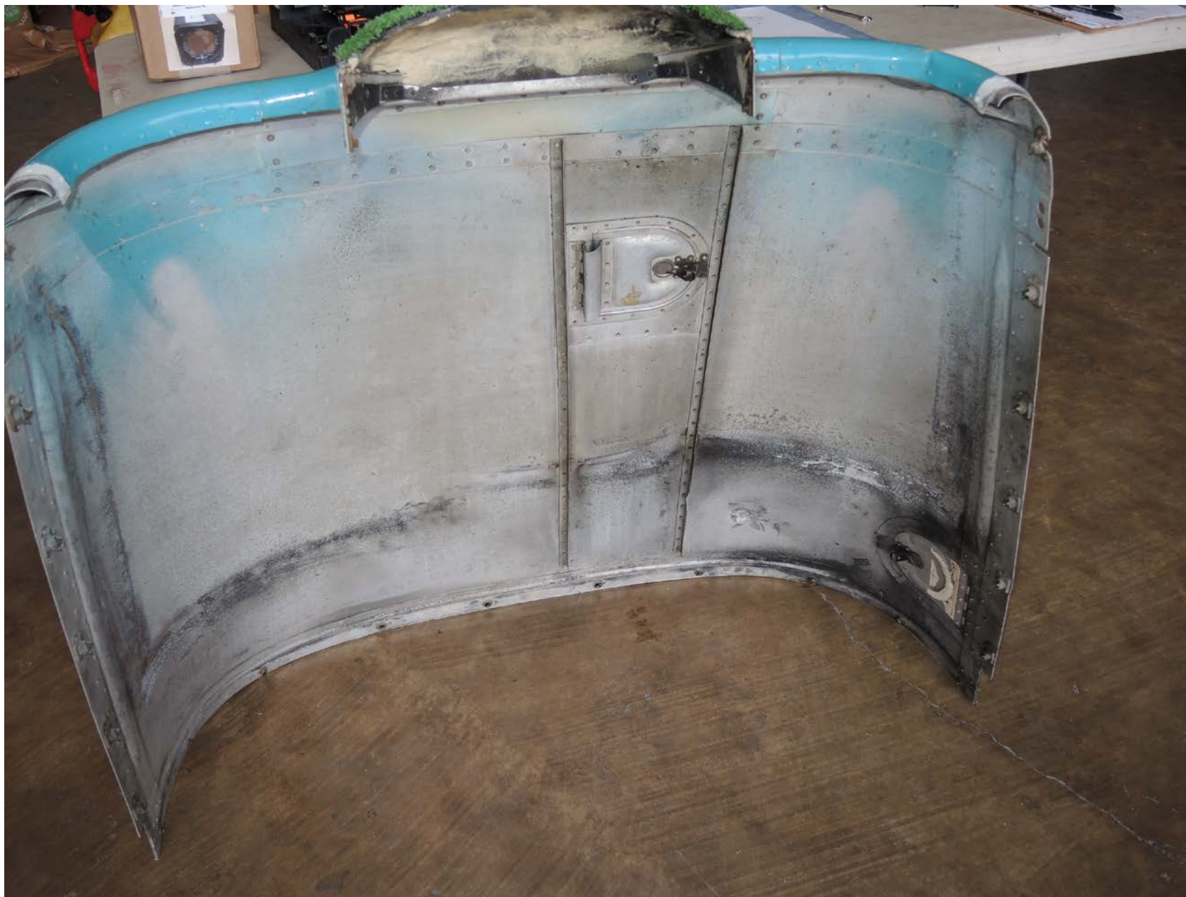
Photo 5 – Inside of top engine cowling
