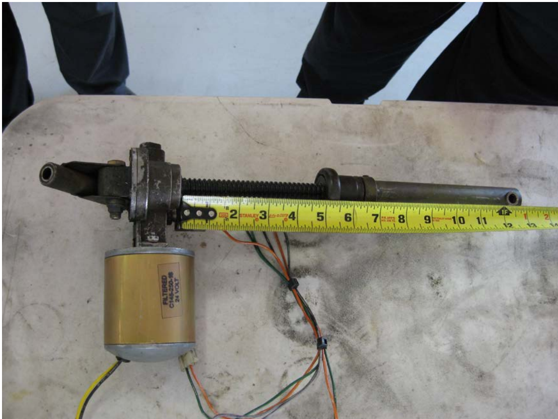
Figure 1 – The flap motor assembly as found by inspectors from the FAA FSDO (FAA photo)
