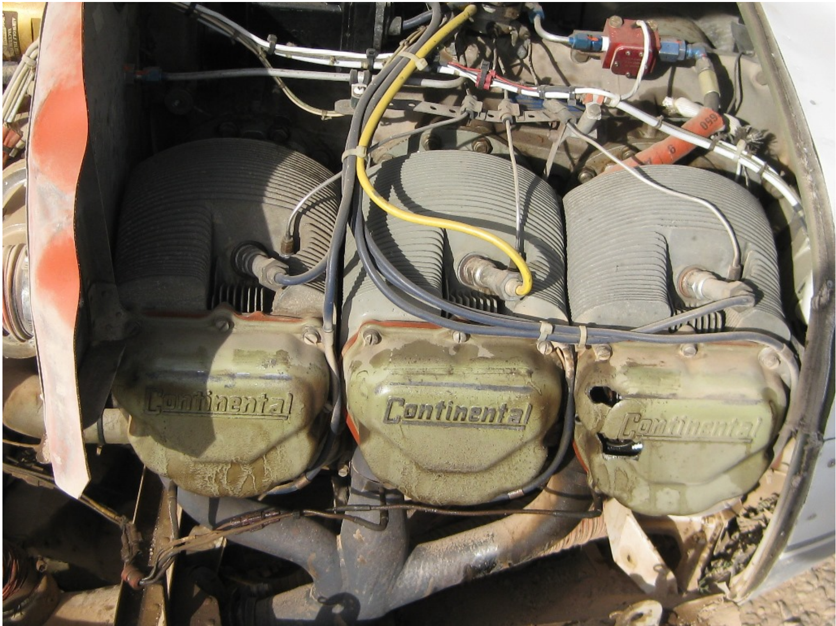
Figure 3 – Engine Cylinder No. 5 Damage
