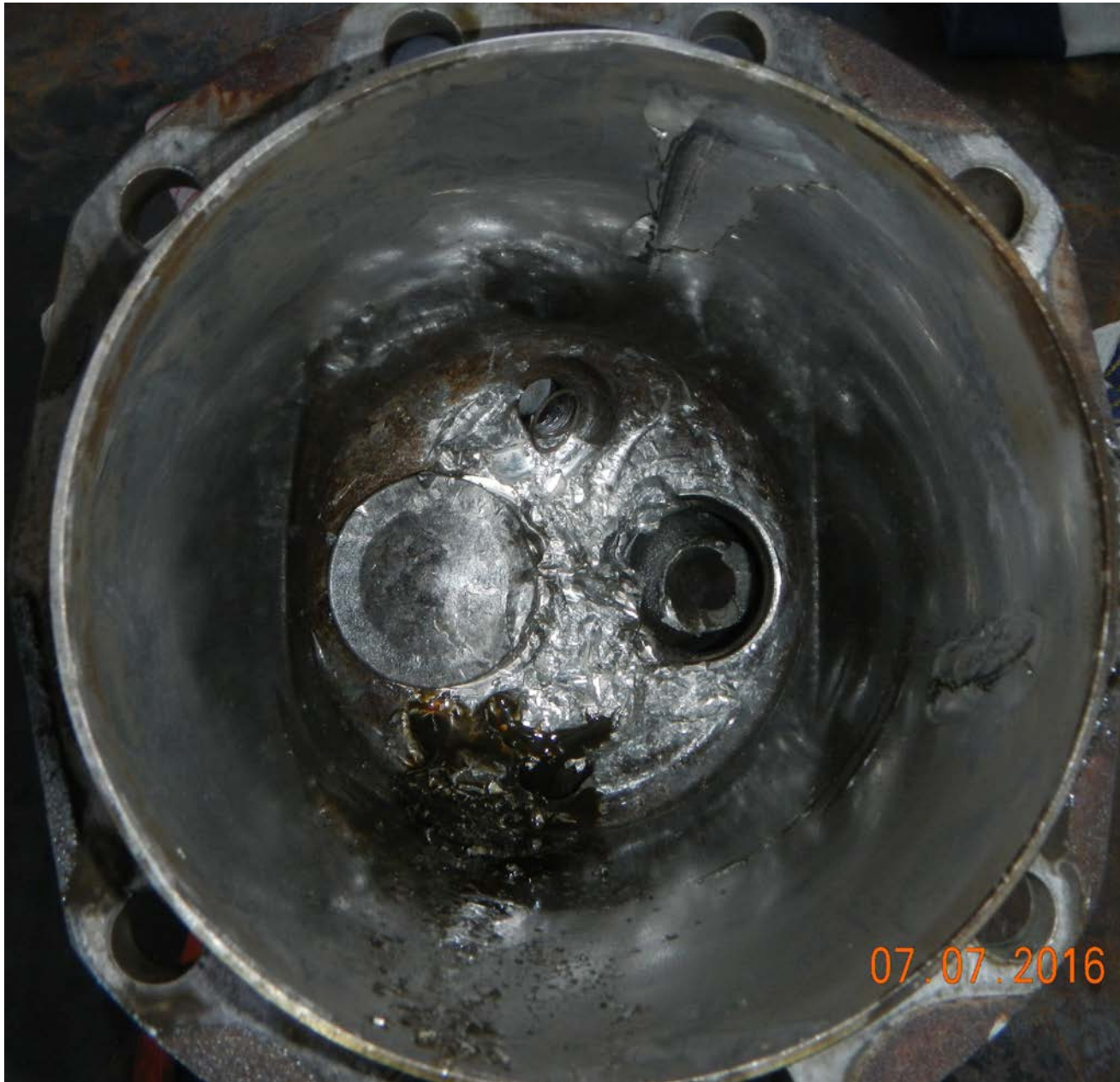
Photo 1 – No. 5 Cylinder Internal Damage
