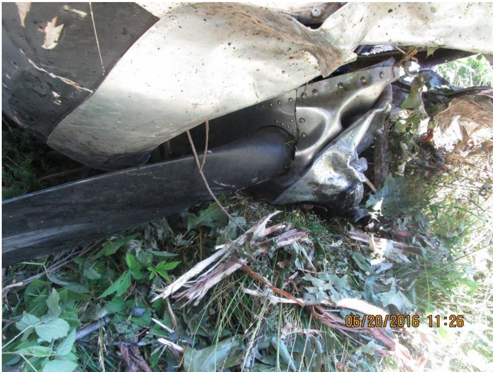
Photo 16 – View of the crushed propeller spinner and other propeller blade
