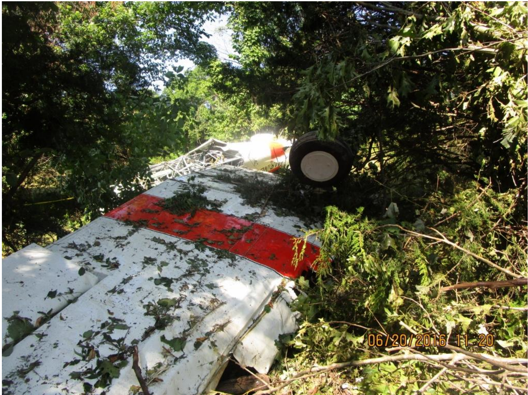
Photo 5 – View of the inverted right wing and landing gear
