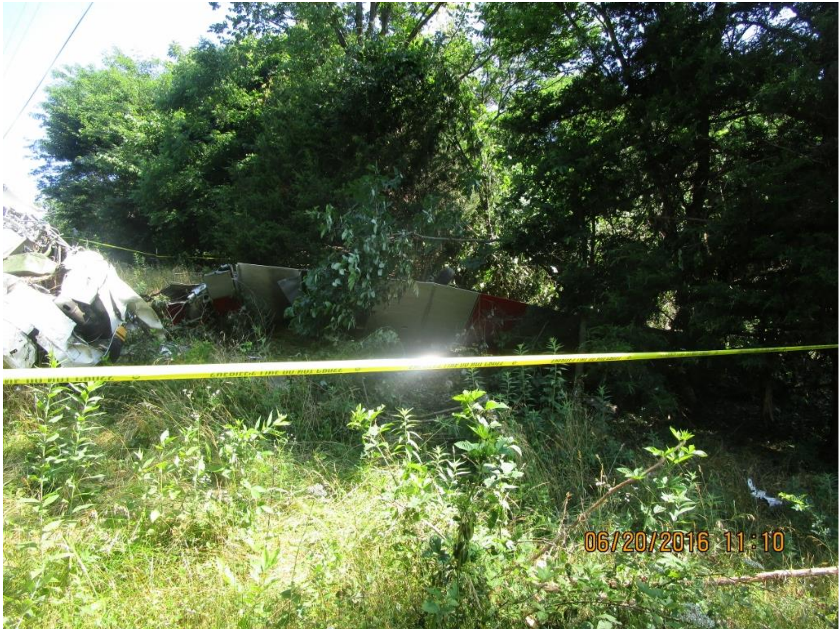
Photo 3 – View of right wing separated and lying next to the fuselage
