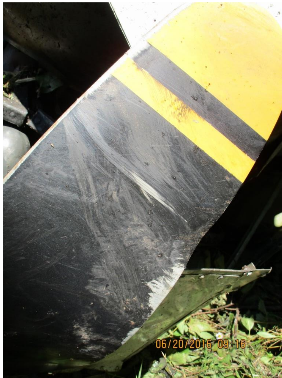
Photo 14 – View of damage to the blade tip
