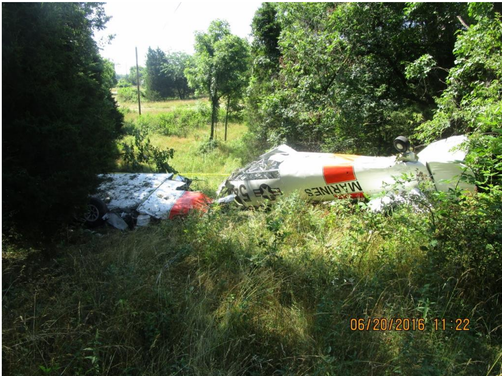
Photo 4 – View of the separated right wing and fuselage from the left rear of the aircraft
