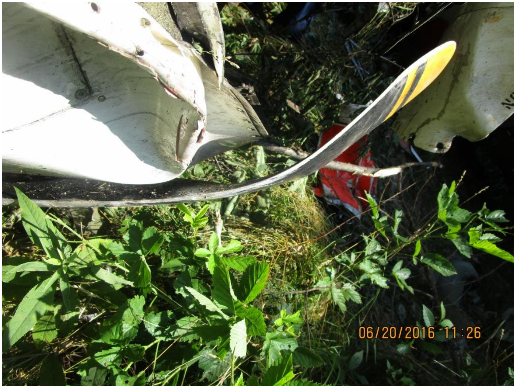
Photo 15 – View of the leading edge of the propeller blade
