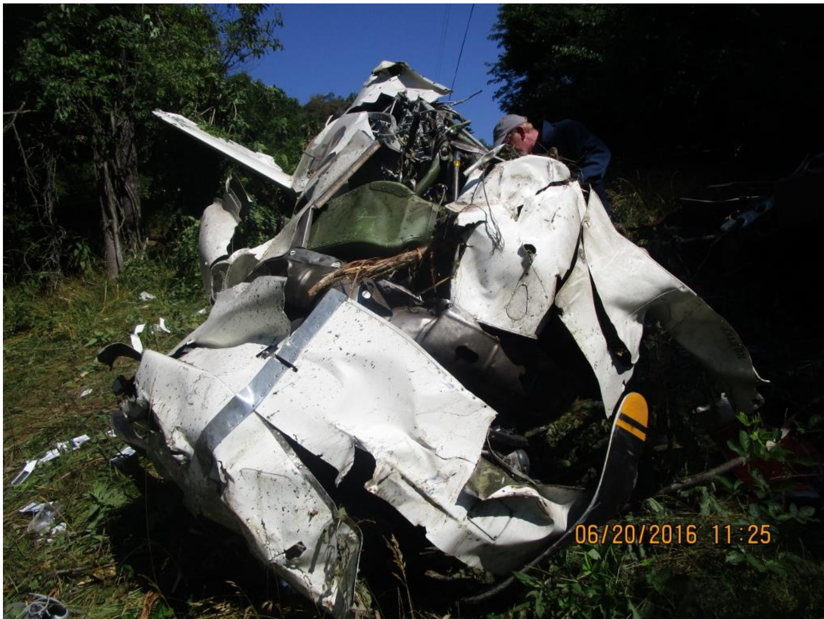
Photo 11 – View of the aircraft’s propeller and the crushed engine cowling
