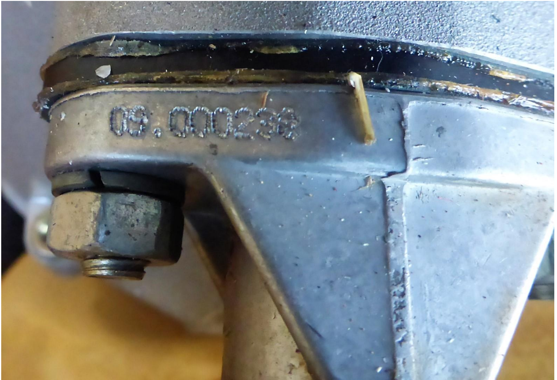
Photo 2 – The fuel pump diaphragm before removal from engine
