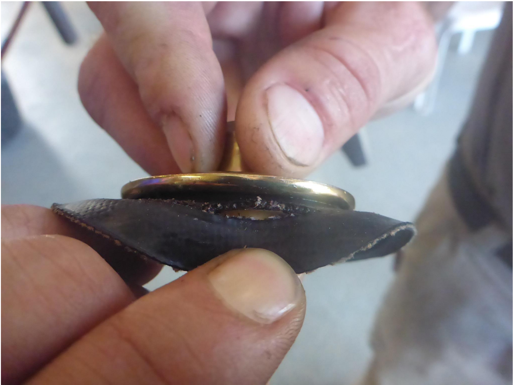
Photo 4 – Side view of hole in fuel pump diaphragm
