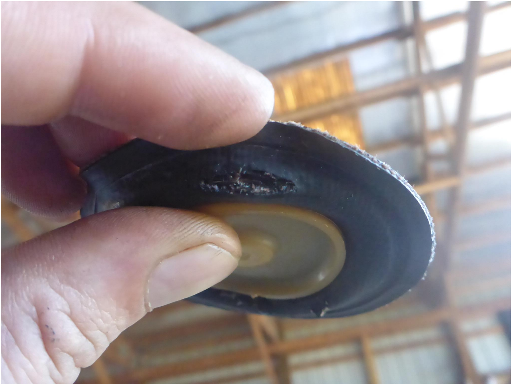
Photo 3 – Hole in fuel pump diaphragm
