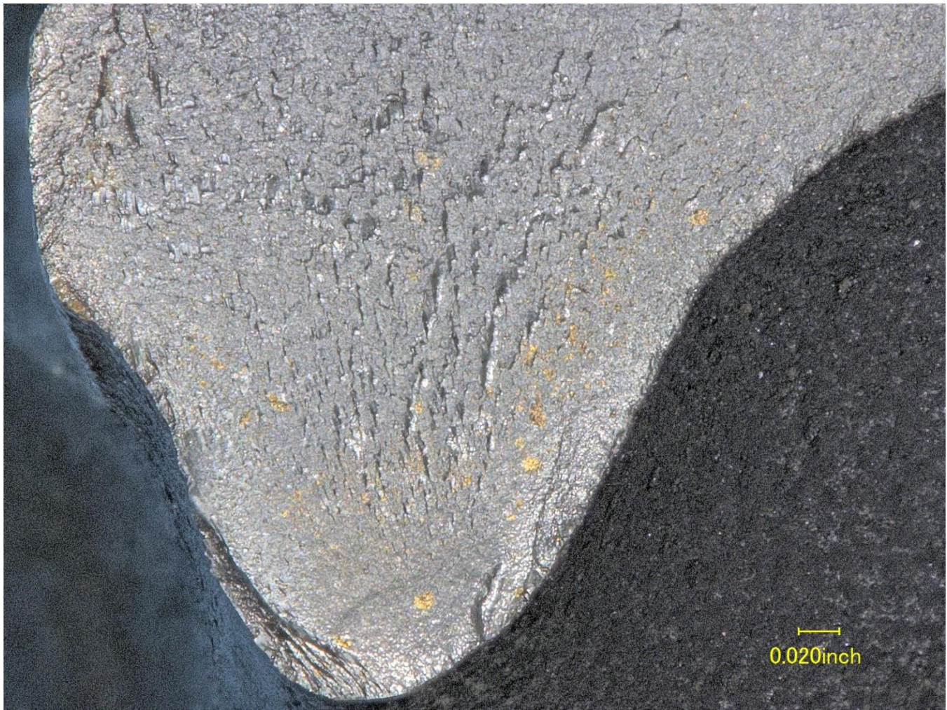
Figure 6 – Closer view of the crack initiation site of the lower left side from Figure 5.
