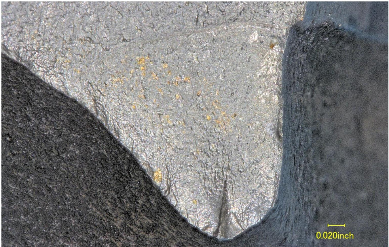
Figure 7 – Closer view of the crack initiation site on the lower right side of Figure 5. A ratchet mark was present in the figure.
