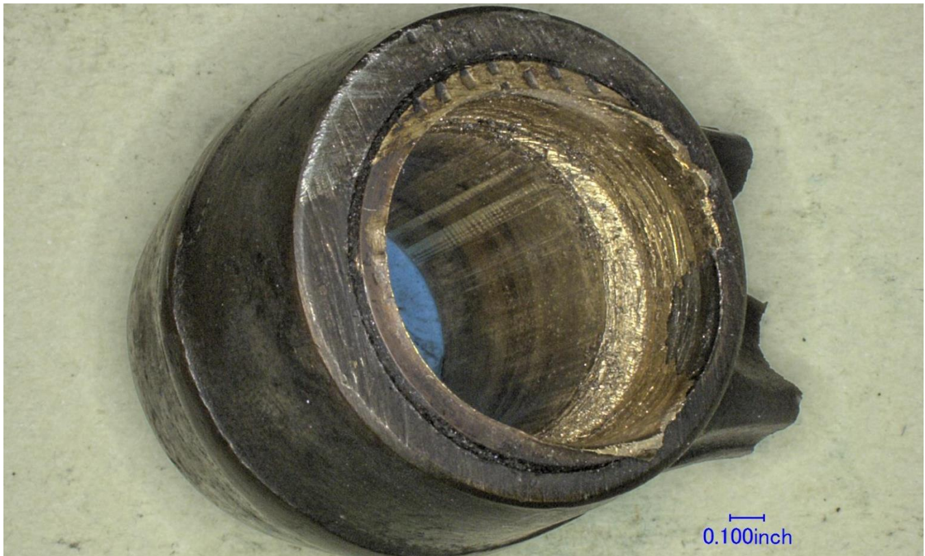
Figure 4 – Side view of the bearing of the fractured connecting rod, where the fractured pin was located.
