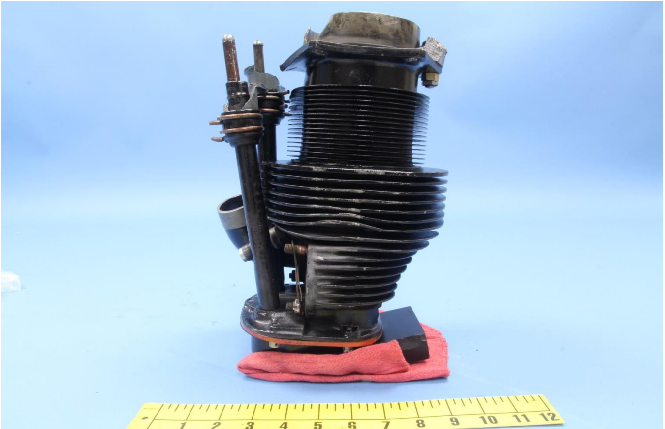
Figure 1 – The #2 cylinder, as received. The upper flange was torn and bent on the top of the figure.
