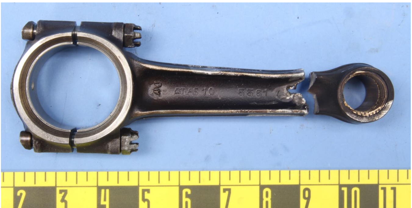
Figure 3 – The fractured halves of the connecting rod, shown after removal of the fragment from the cylinder (right).
