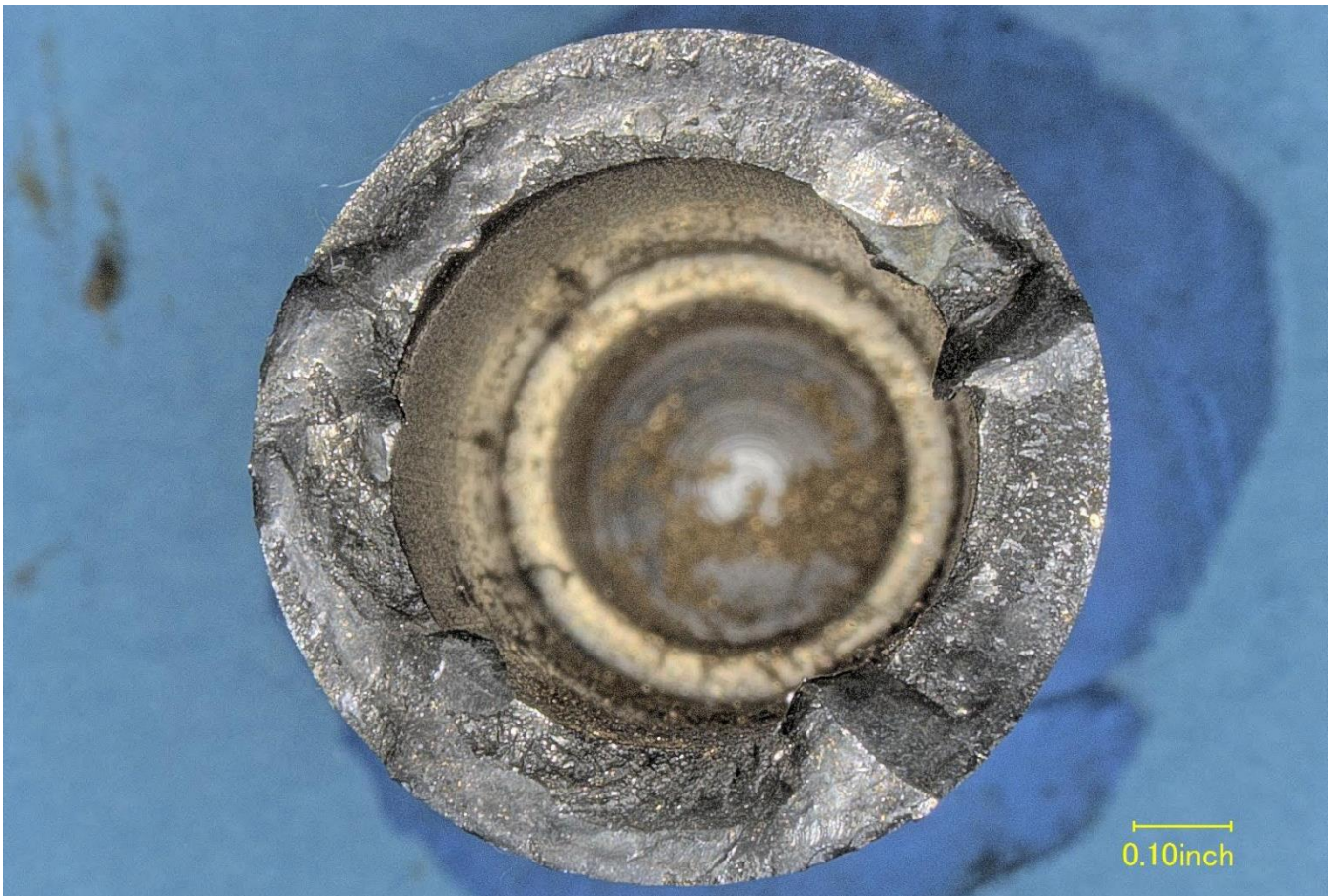
Figure 13 – The less damaged fracture surface of the pin from the connecting rod.
