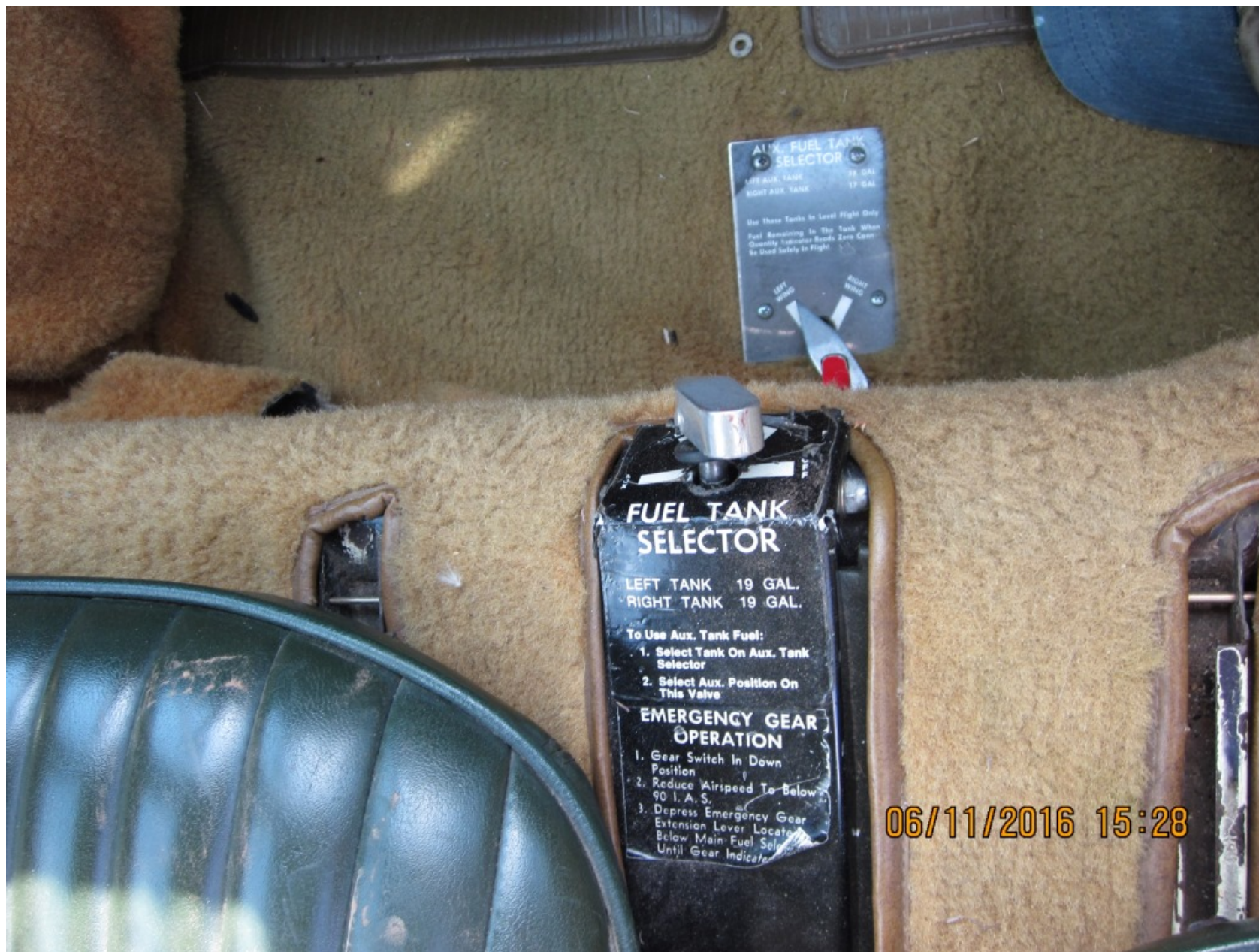
Photo 3 – Fuel Selector Valve (FAA Photo)
