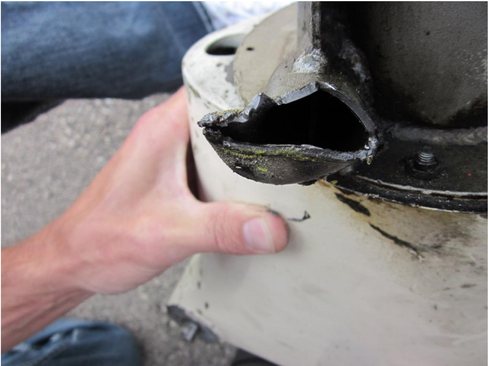
Photo 10 - View of nose gear fracture surface
