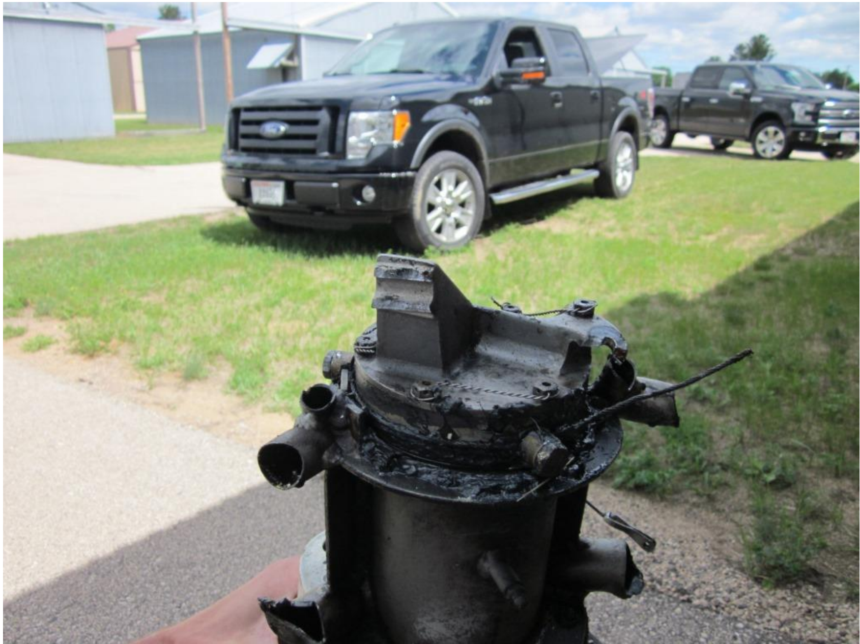
Photo 6 – View of the fracture surfaces on the top of the broken nose gear
