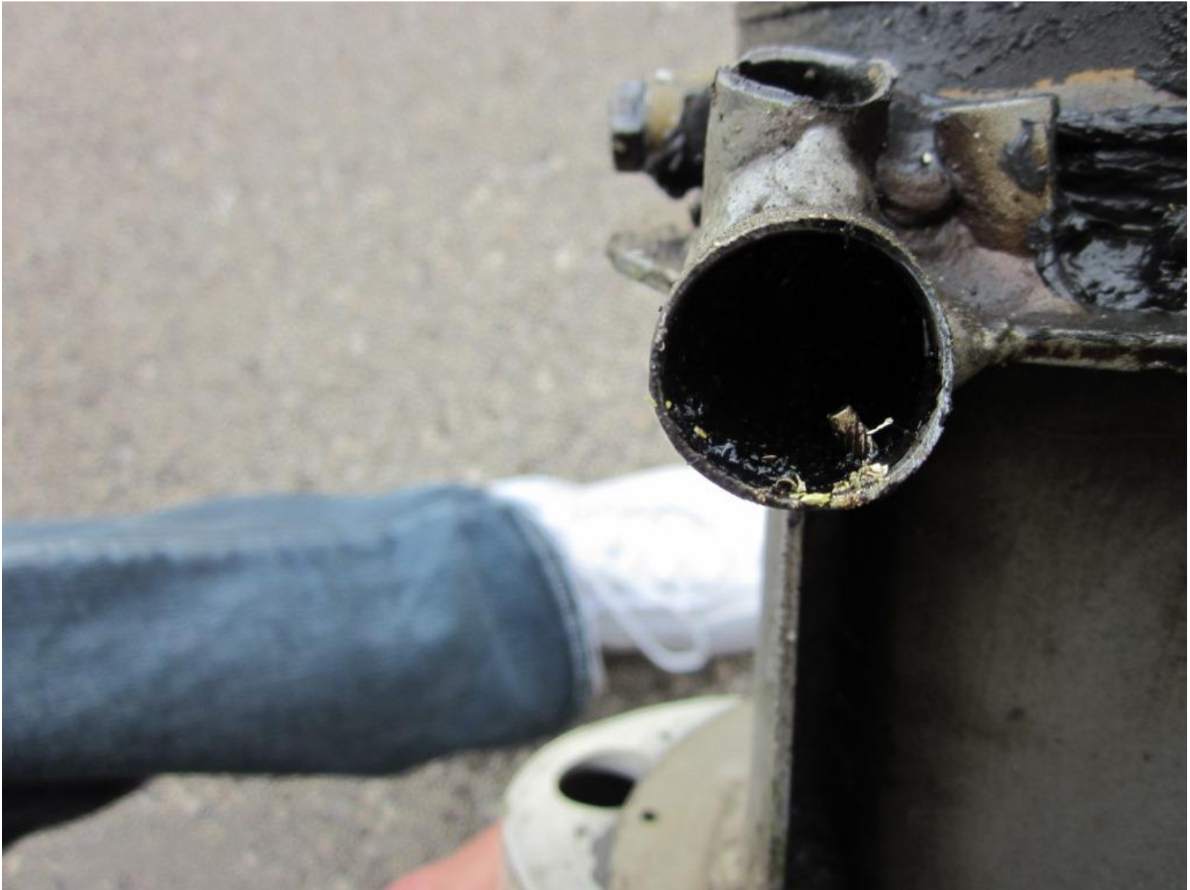
Photo 11 - View of nose gear fracture surface
