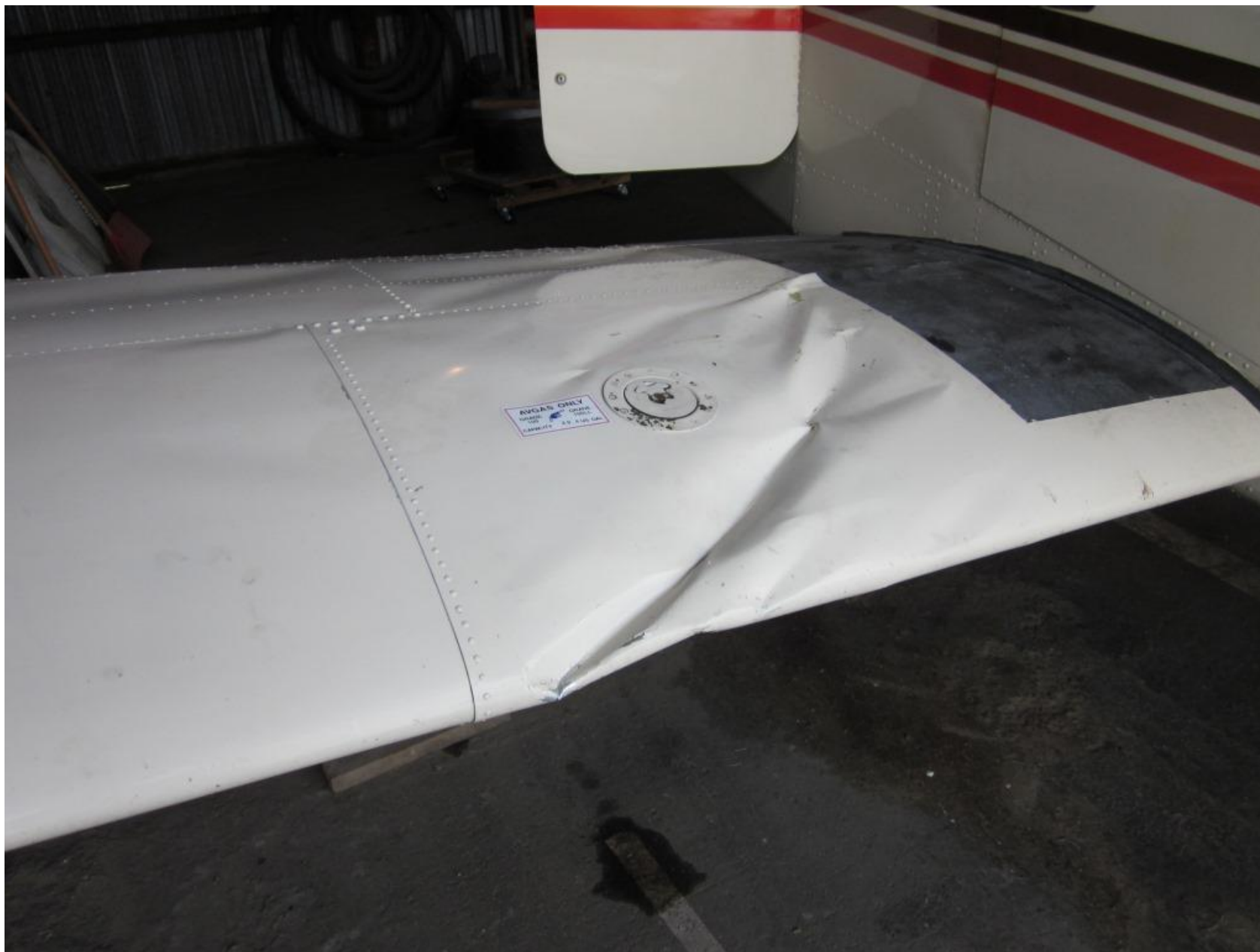
Photo 2 – View of damage to the right wing
