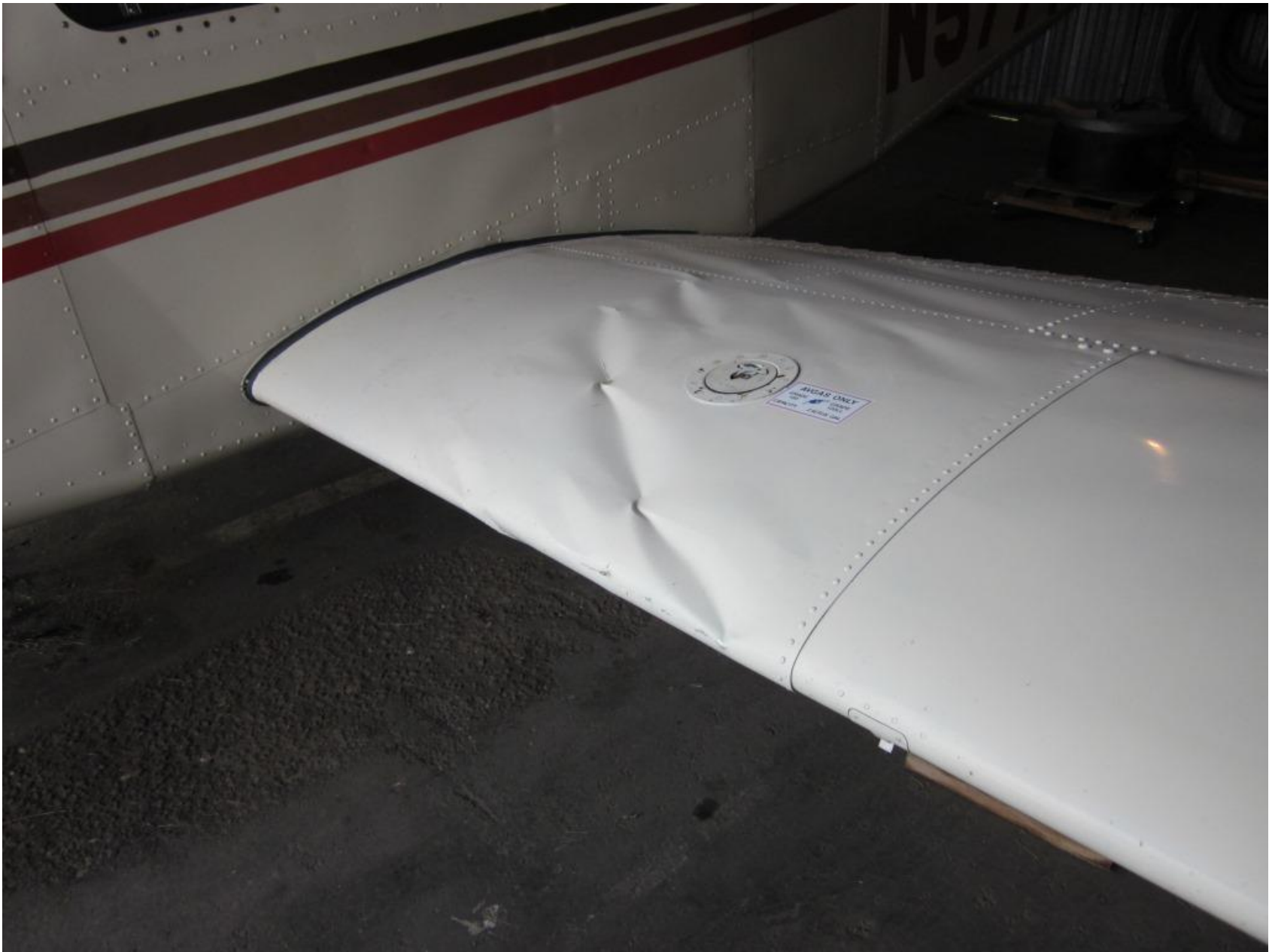
Photo 1 – View of damage to the left wing
