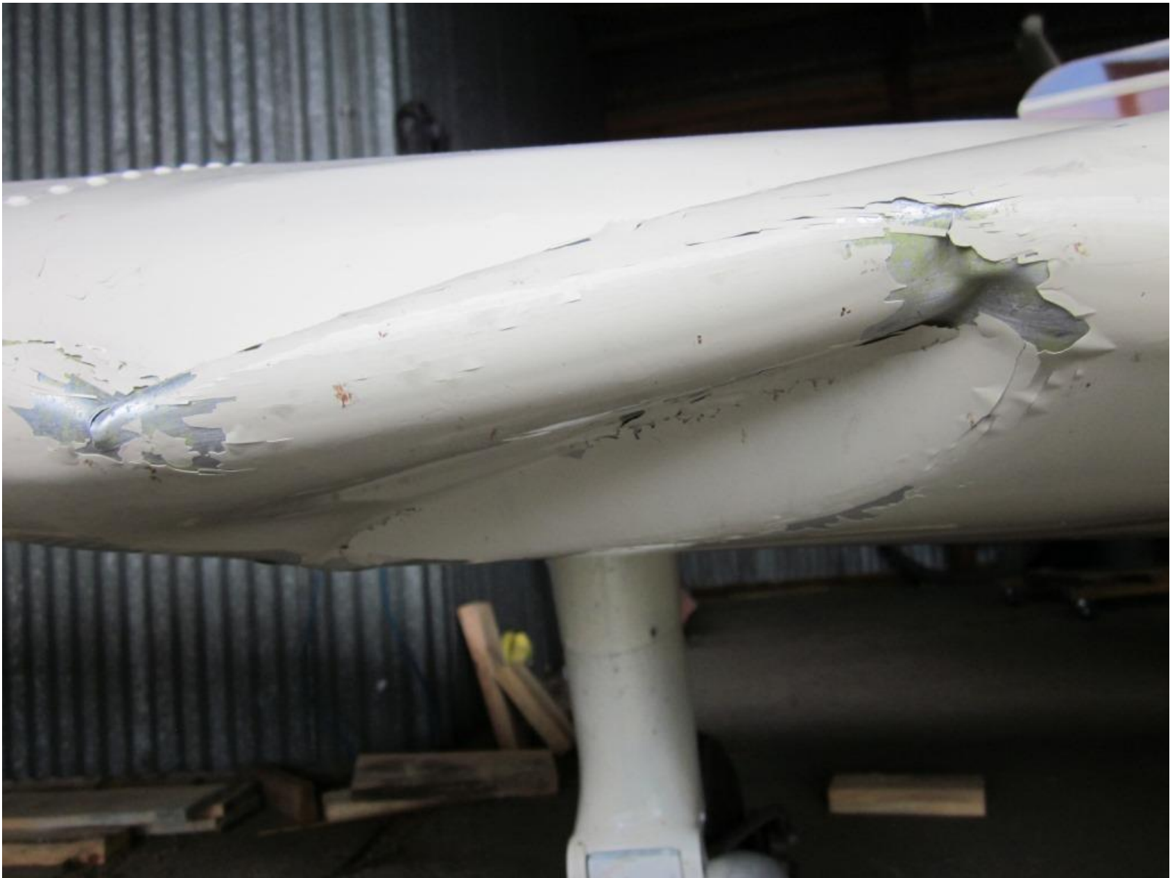
Photo 3 – Leading edge damage to the right wing
