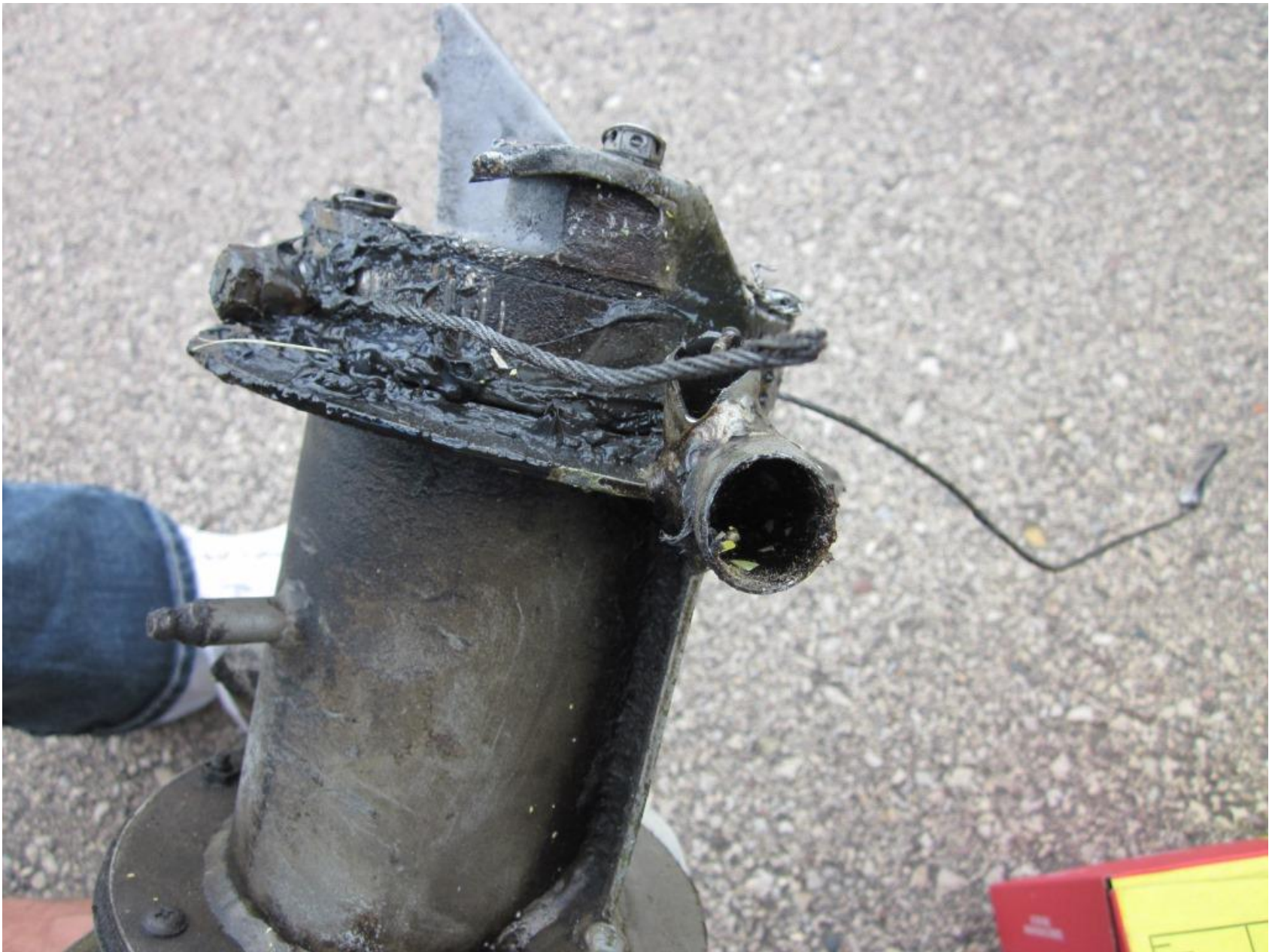
Photo 9 - View of nose gear fracture surface
