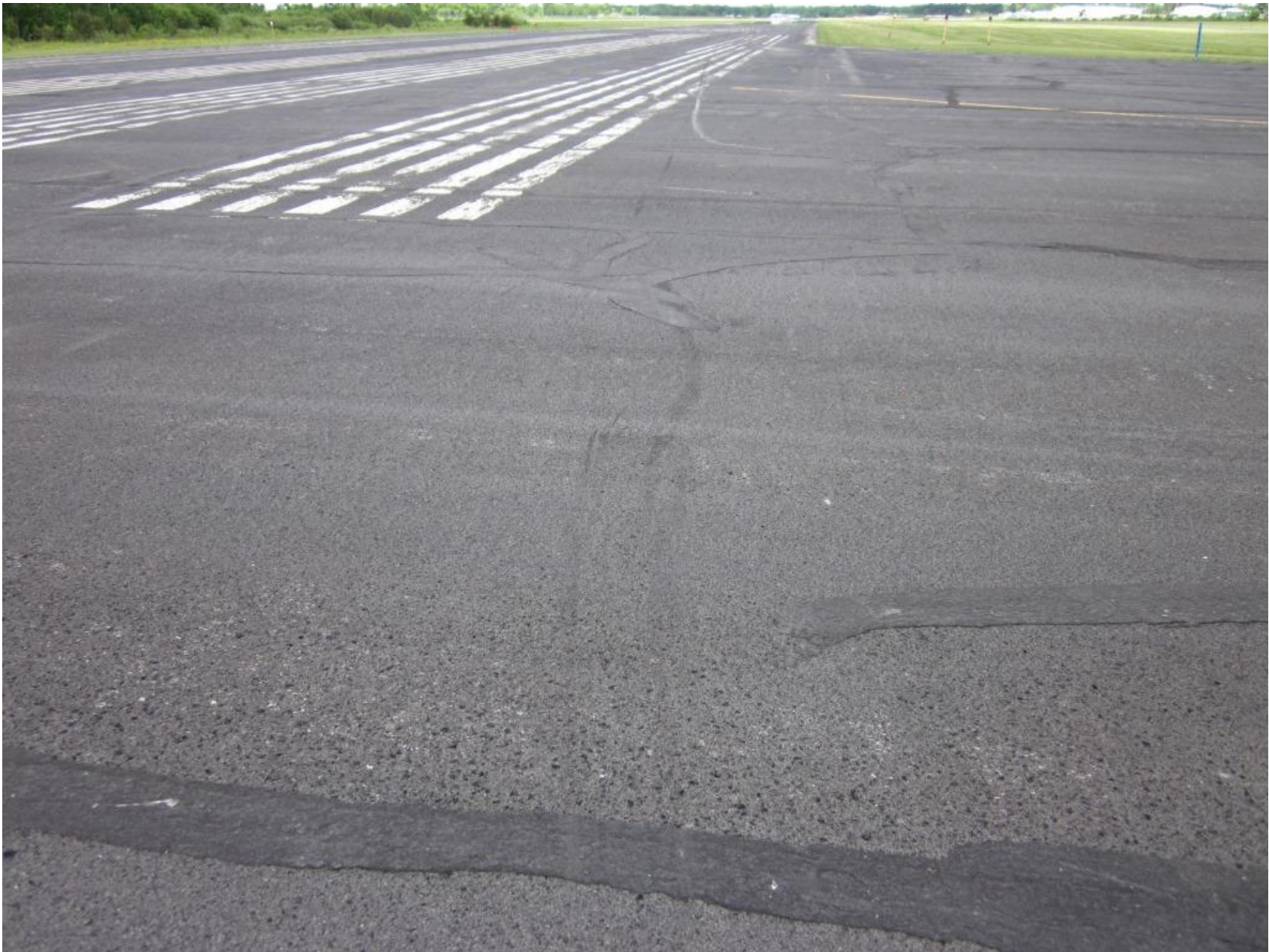
Photo 15 – View of nose gear tire marks leading to the first propeller strike
