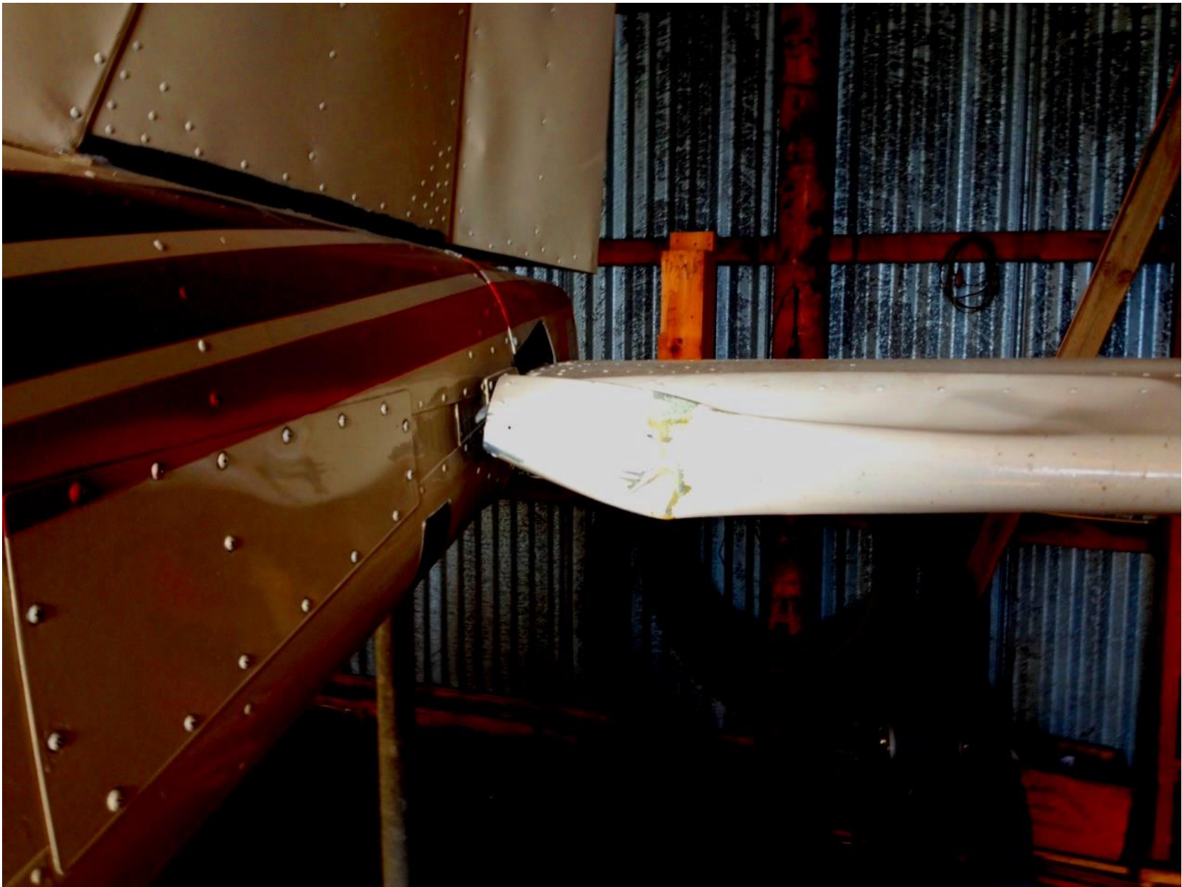
Photo 19 – View of damage to the left horizontal stabilizer
