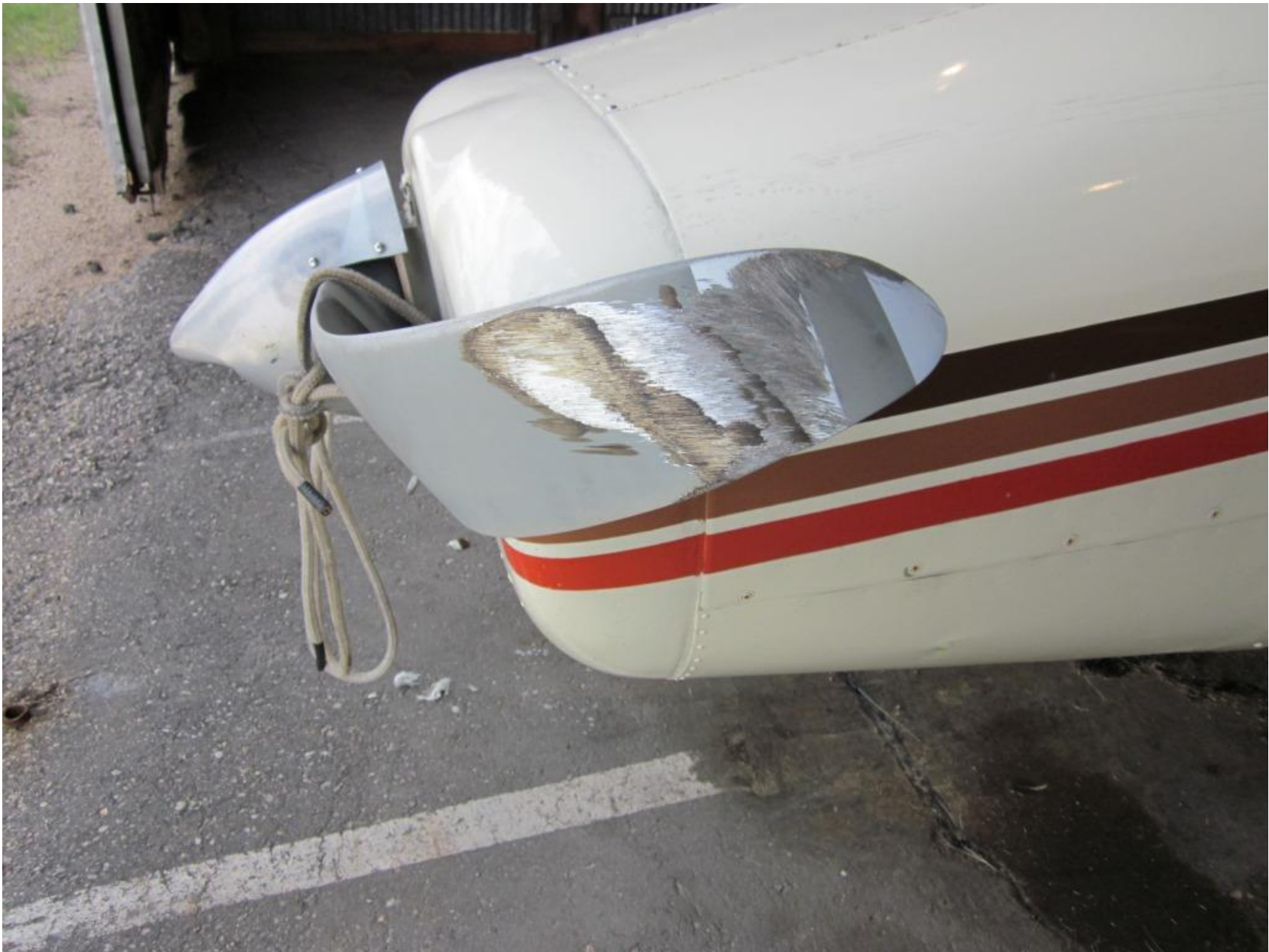
Photo 4 – Impact marks on a propeller blade
