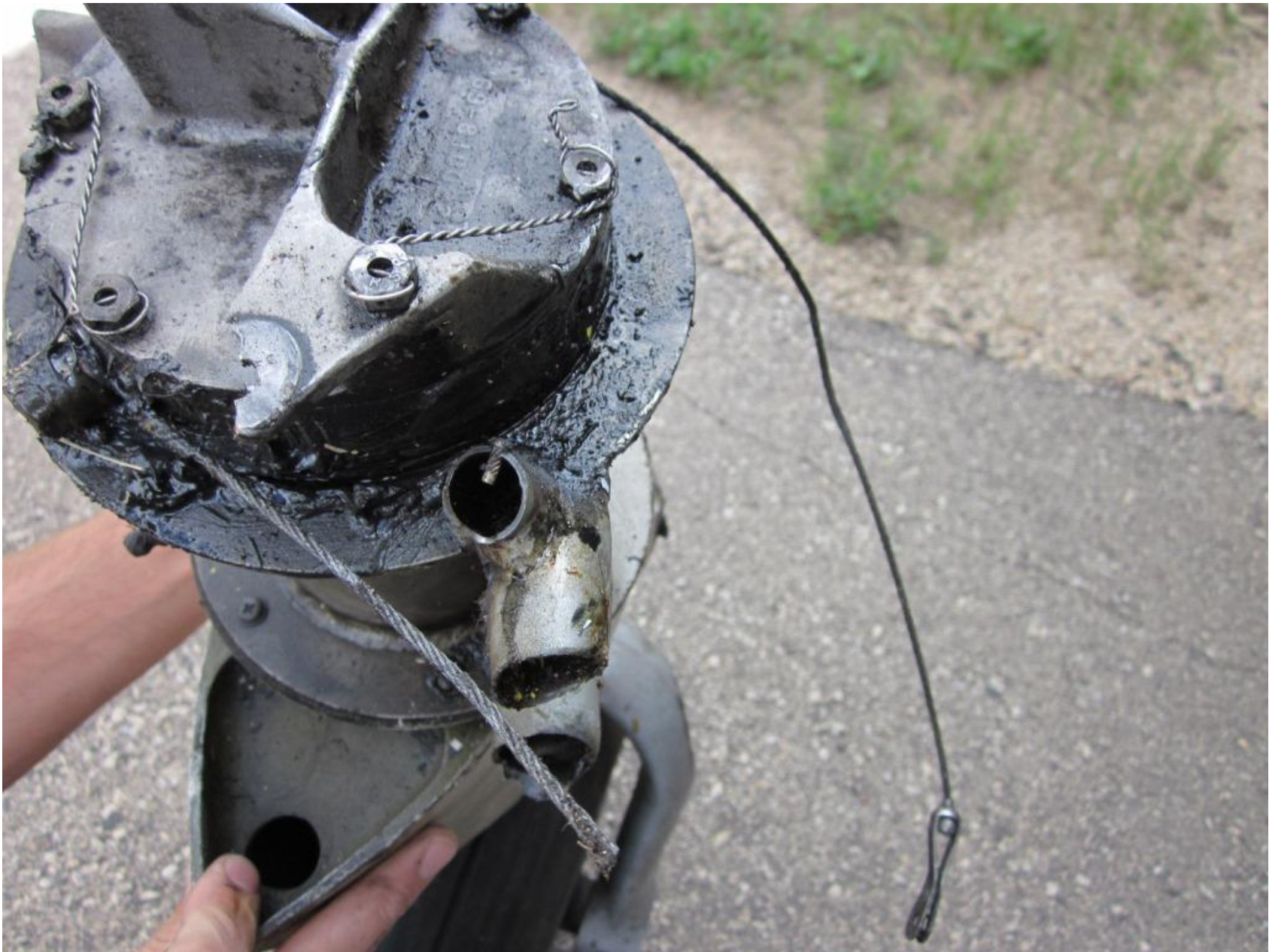
Photo 7 – View of fracture surfaces on the bottom portion of nose gear
