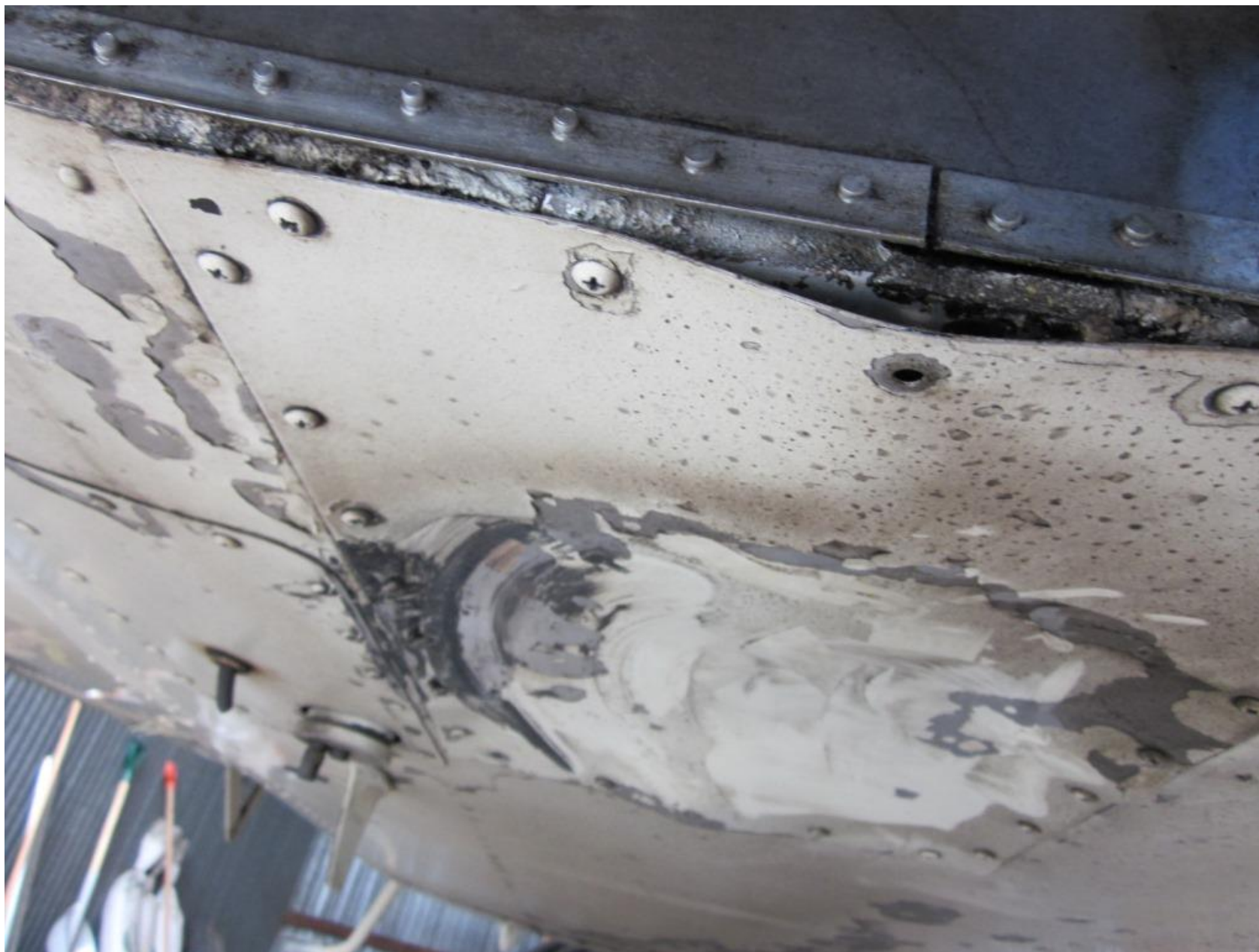
Photo 5 – Indentation of belly skins from nose wheel
