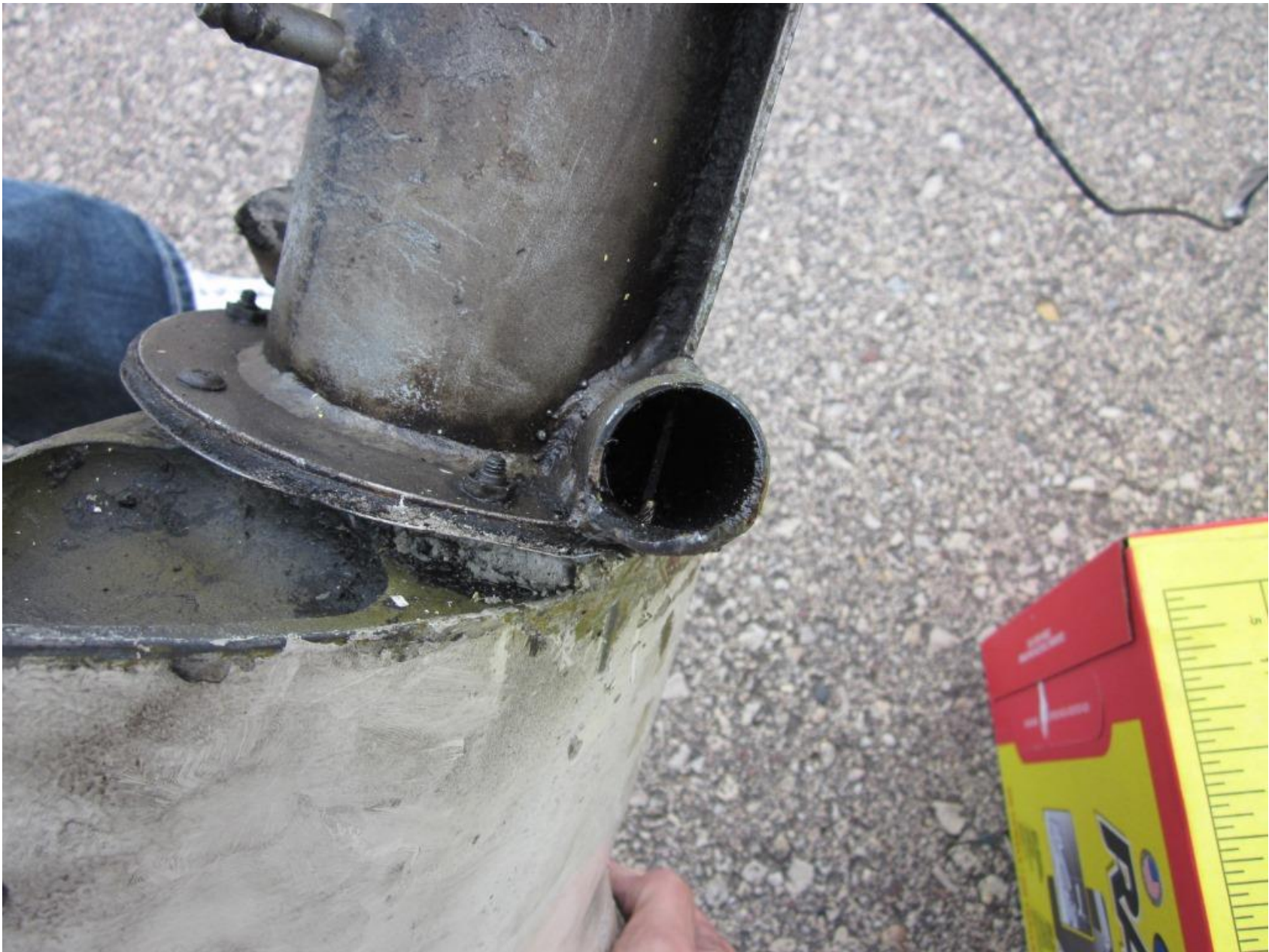
Photo 8 – View of nose gear fracture surface
