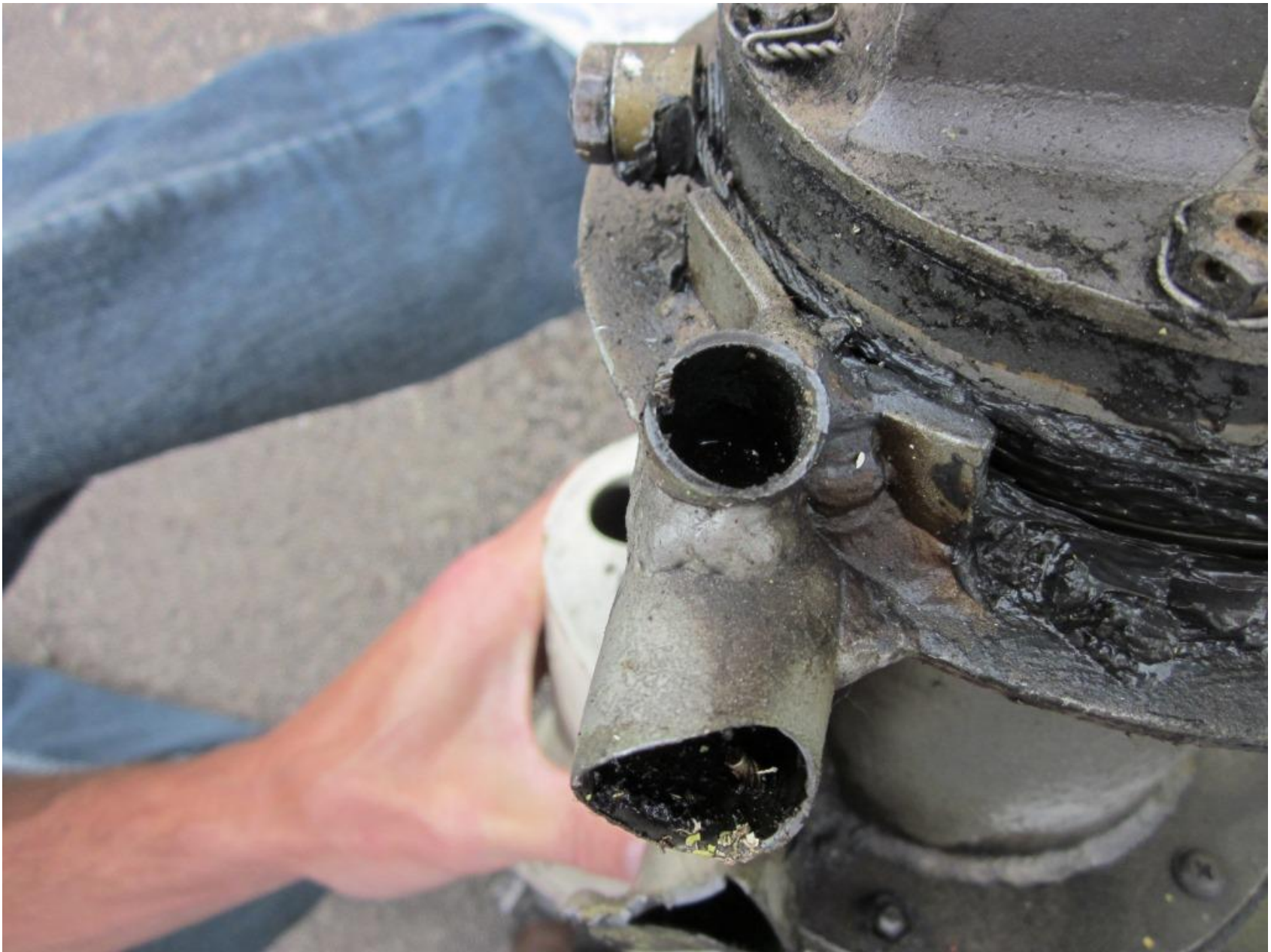
Photo 12 - View of nose gear fracture surface
