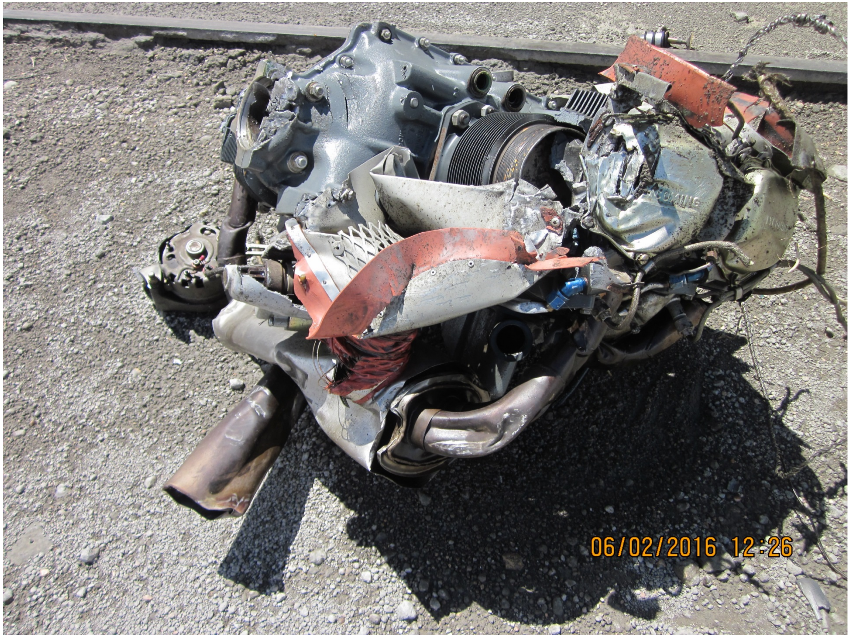
Photo 4 – The engine, separated from N5879G by impact.
