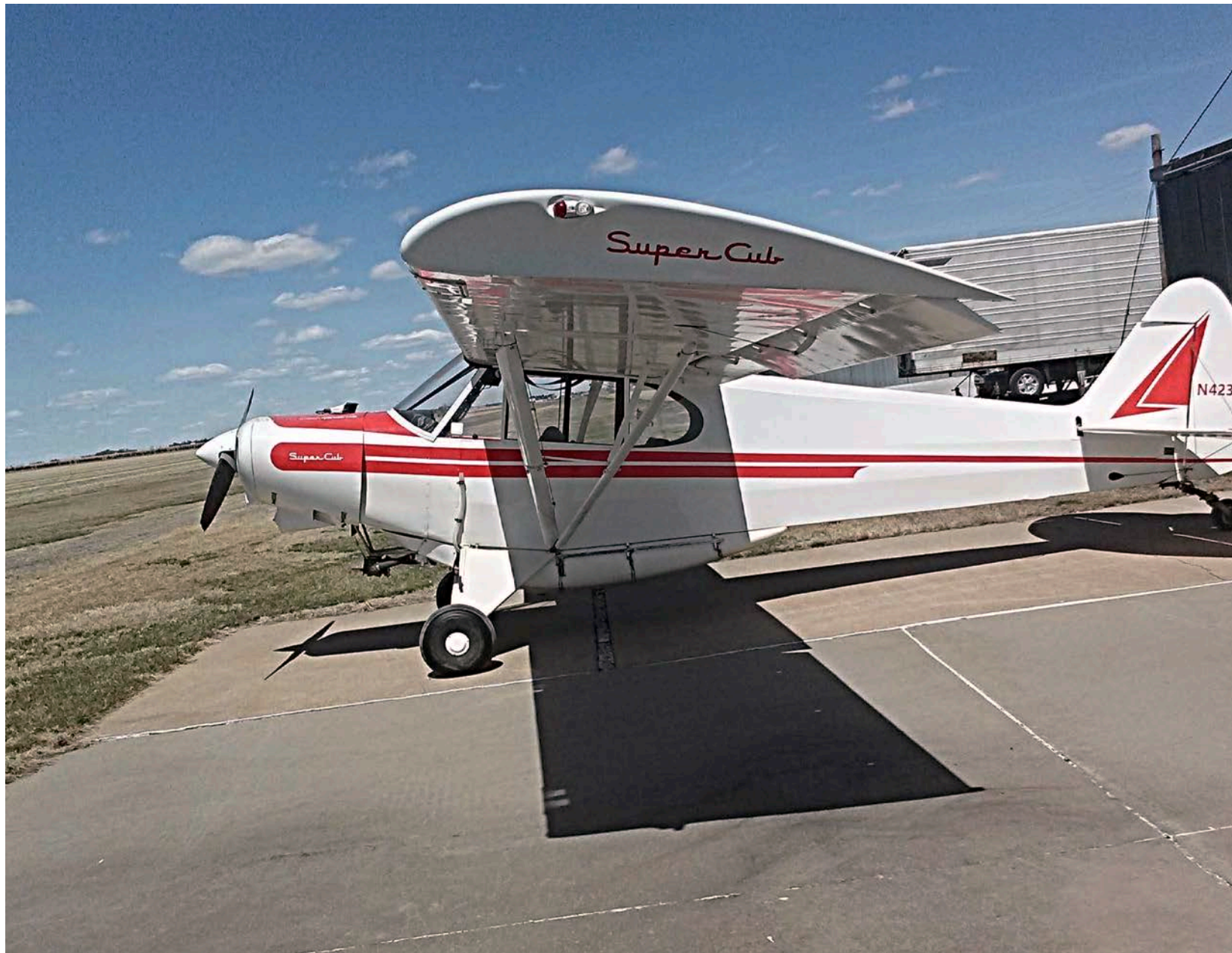
Photo 1 – Pre-accident photograph of N4234Z, showing a 90-gallon Sorensen tank on bottom of fuselage. The front of the tank is about 2 inches aft of the front of the landing gear leg.
