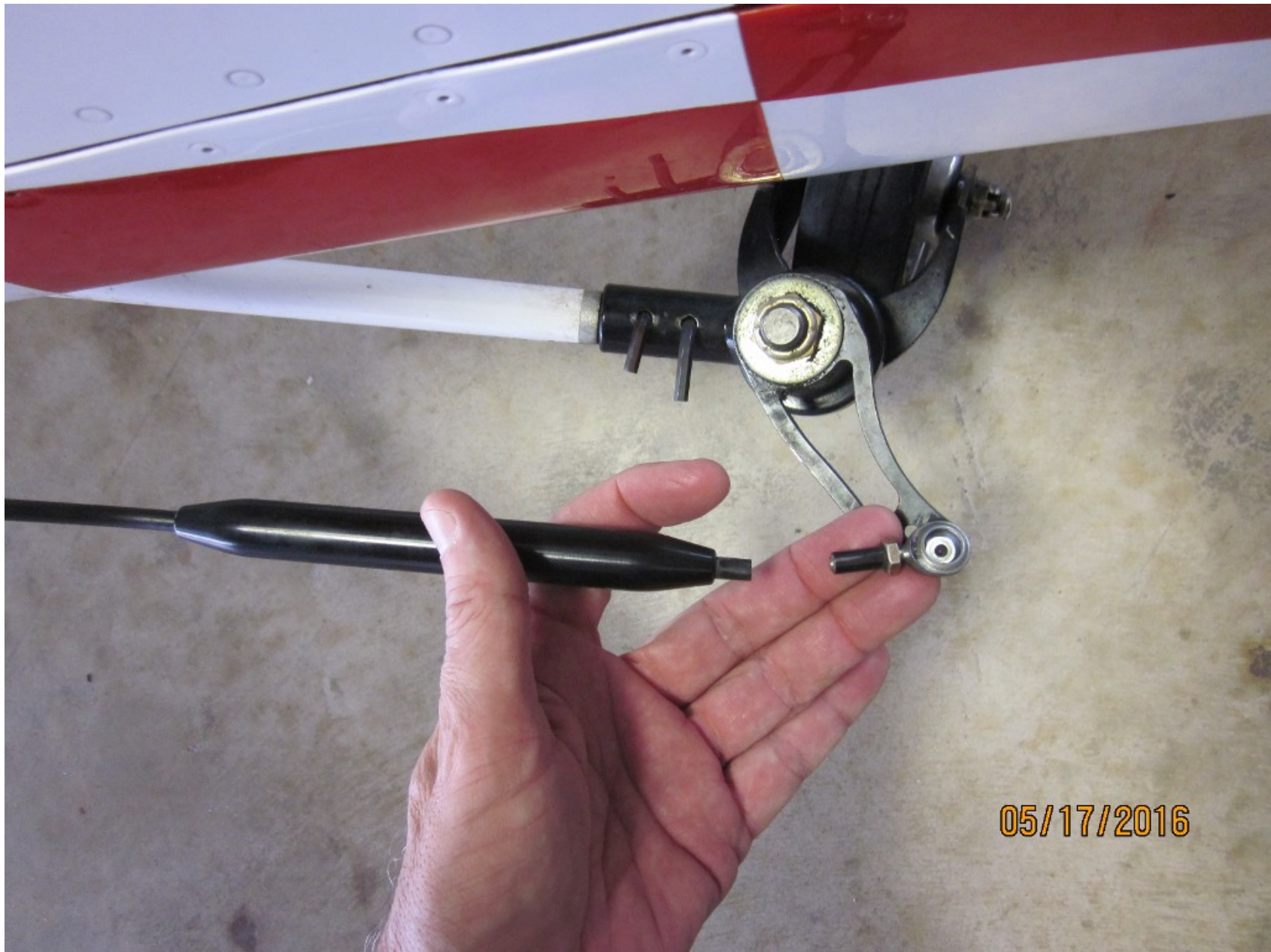
Photo 2 - Broken tailwheel link Photo courtesy of FAA
