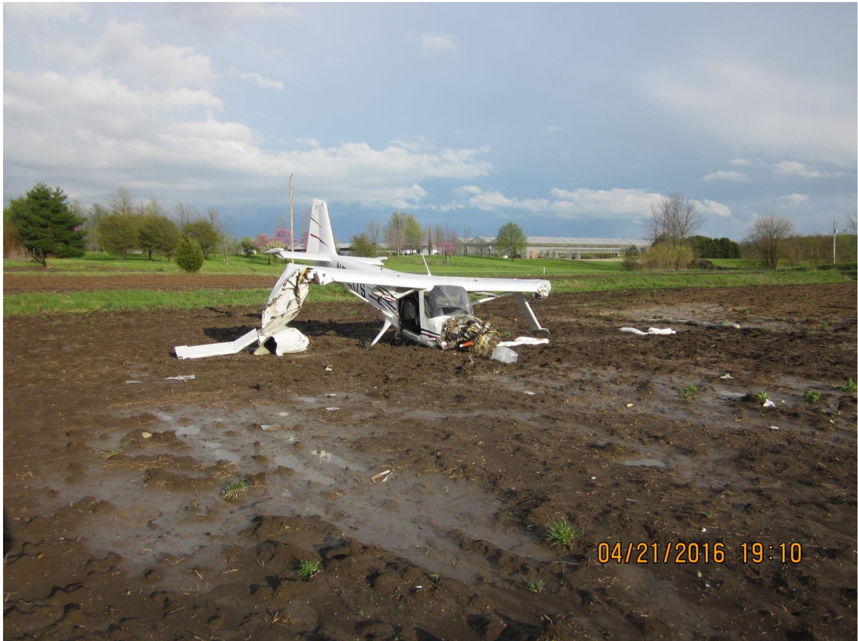
Photo 3 – View of airplane damage to nose gear, left and right wings
