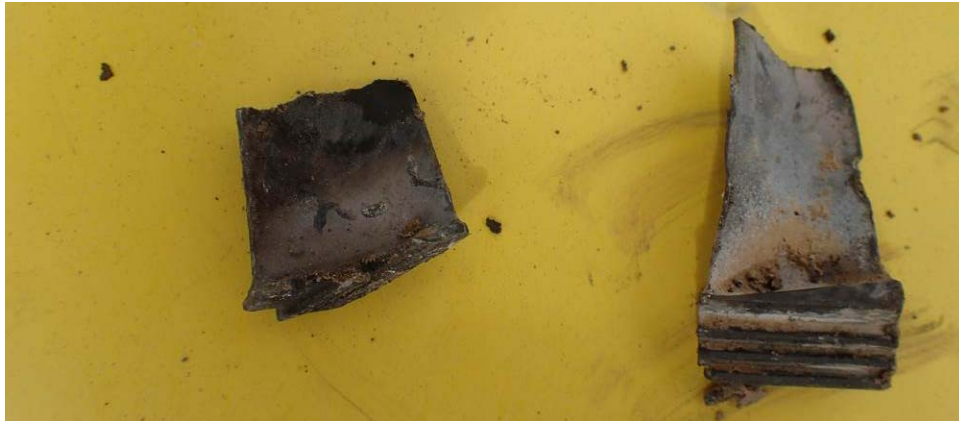
Power Turbine Blades
