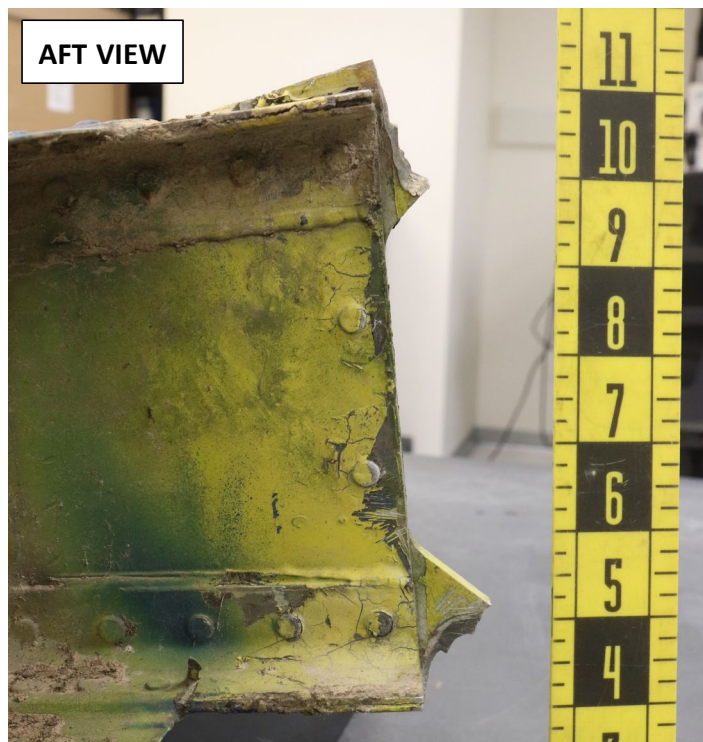
Figure 7. Macro photos of the stabilizer fin attach plate as viewed from the forward and aft directions.
