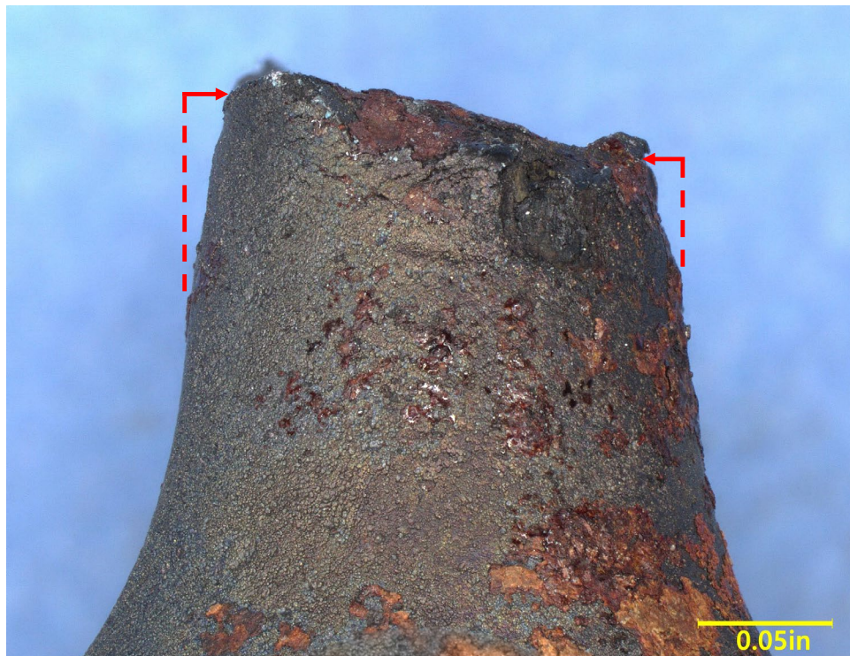
Figure 22. Digital microscope images of the fracture surface and profile of the separated deflector cable terminal end. The red dashed lines indicate the reduced diameter from necking of the terminal end.
