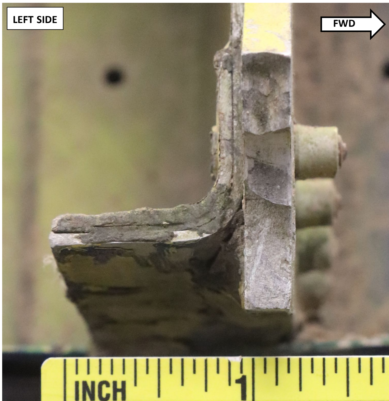
Figure 6. Close-up photo of the fracture surface on the separated left lobe of the stabilizer fin attach plate.
