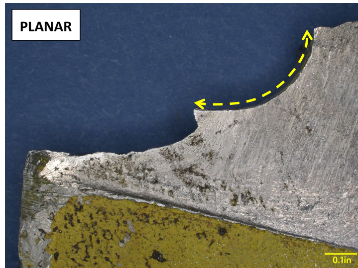
Figure 17. Digital microscope images of the fractured left lobe of the stabilizer fin attach plate. The red and orange dotted lines outline thumbnail-shaped fatigue regions on the fracture surface. The red brackets indicate the location at the forward face of the attach plate from which macro features of fatigue emanated. The yellow dashed lines indicate the edges of the attach hole.
