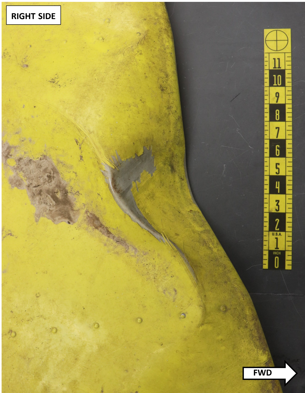
Figure 9. Close-up photo of a large area of buckling at approximately mid-length on the leading edge of the stabilizer.
