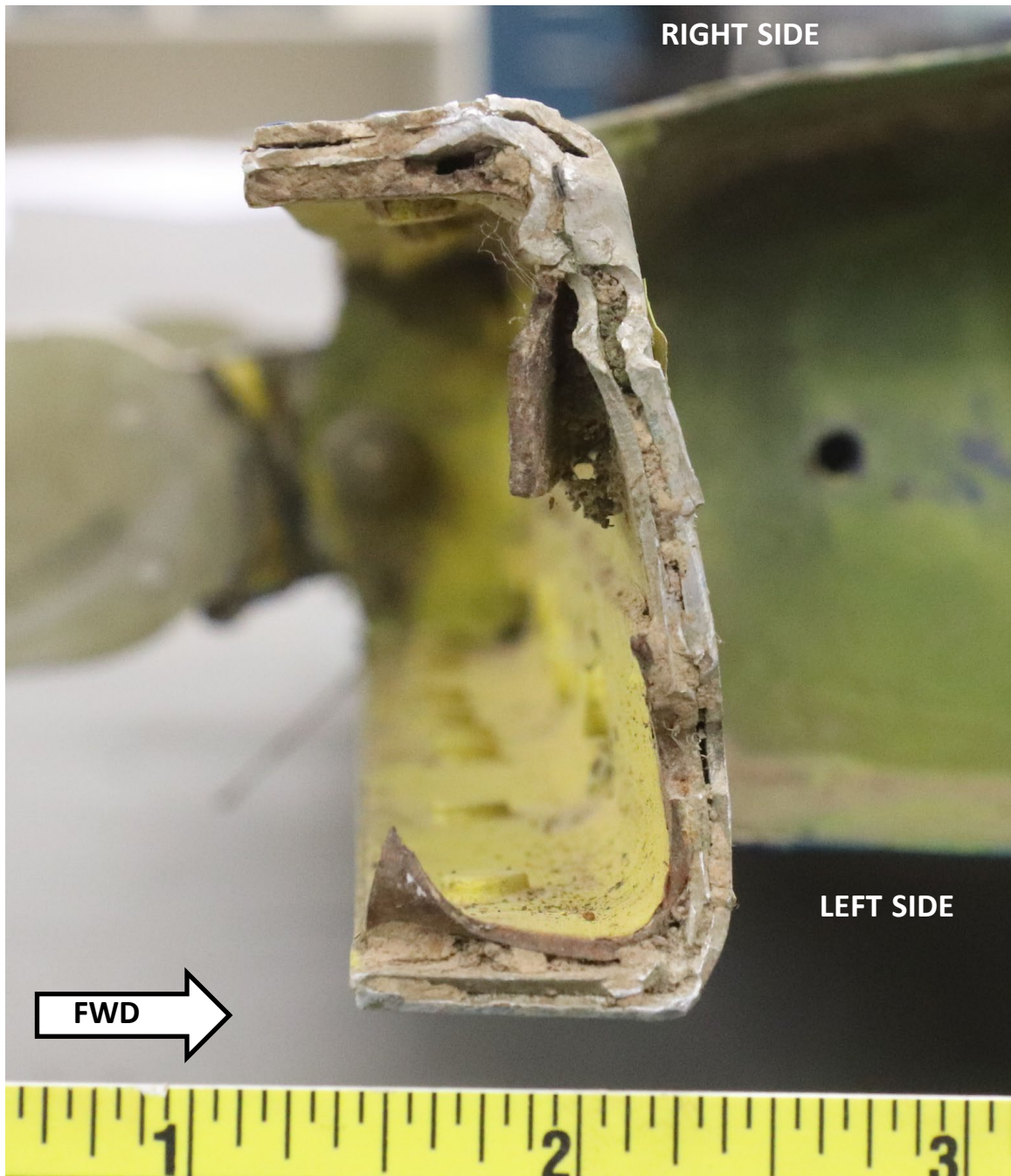
Figure 12. Close-up photo showing twisting of the rear spar of the stabilizer.
