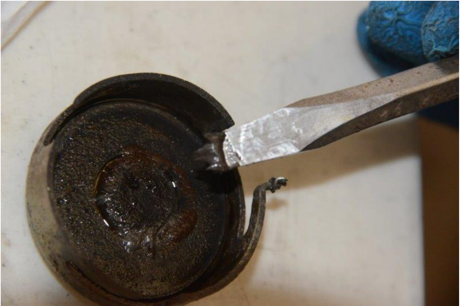
Photo 5 - View of the electric fuel pump cap.
