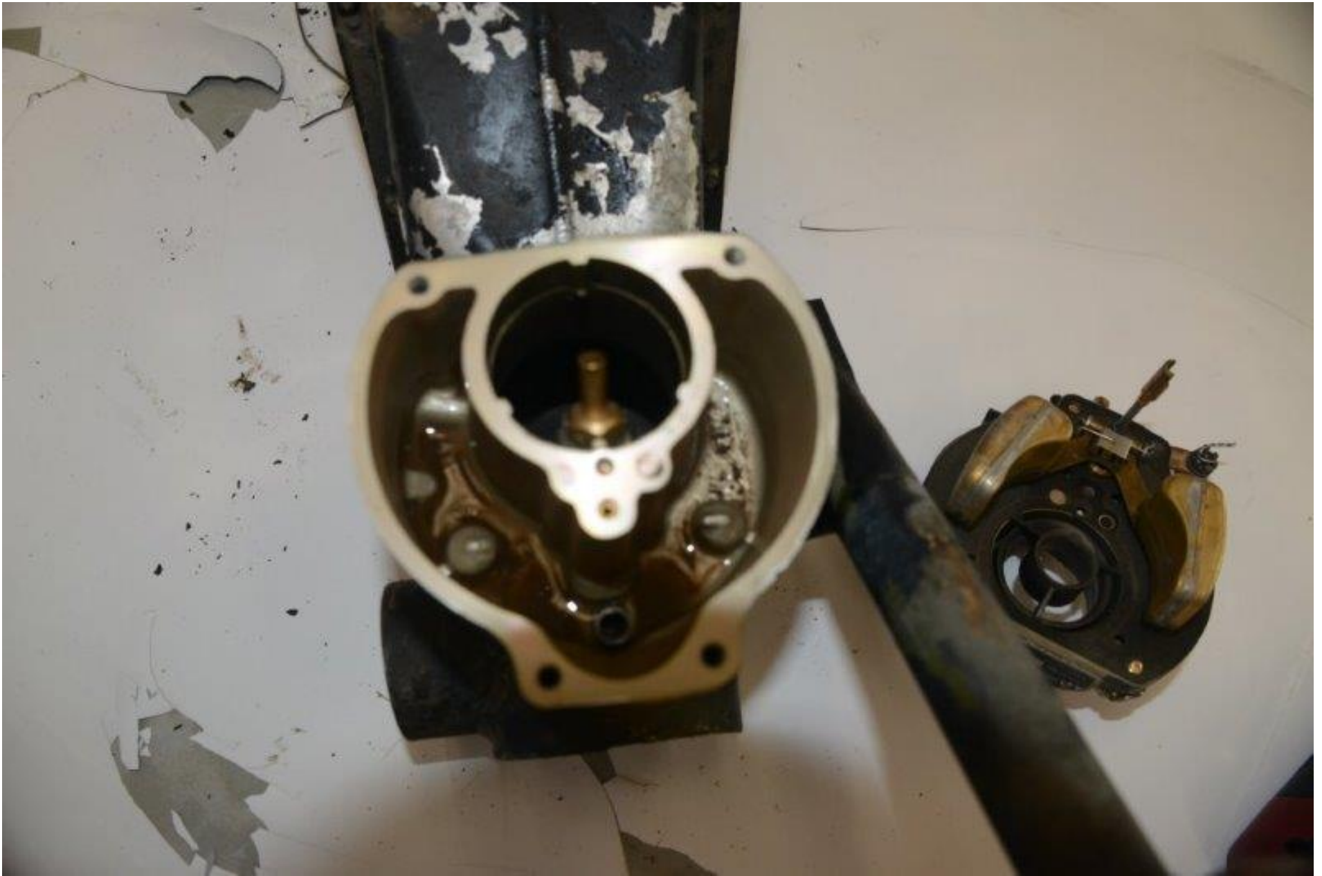
Photo 2 - View of the carburetor with liquid in its bowl.
