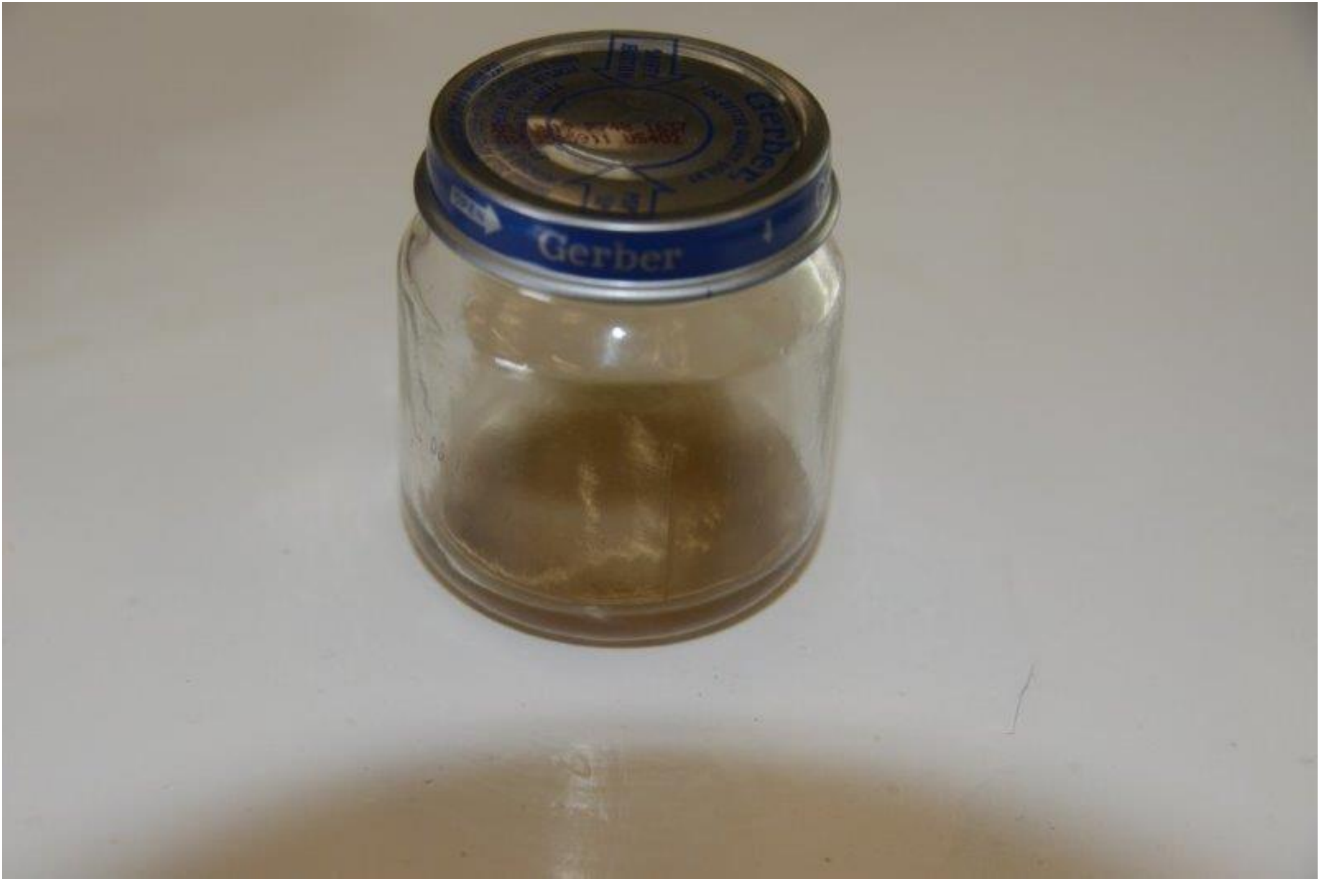
Photo 3 - View of the liquid from the carburetor bowl.
