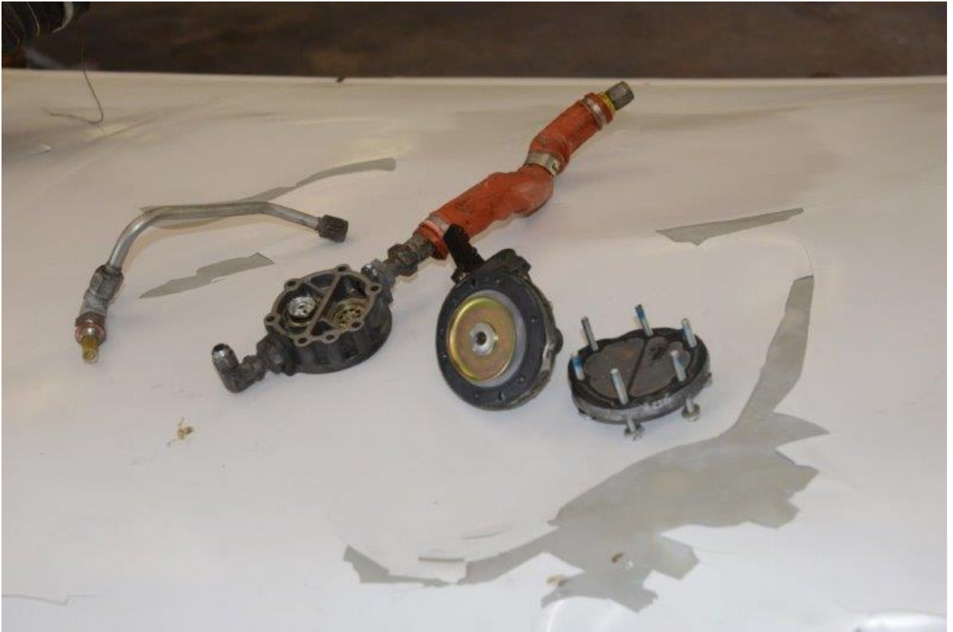
Photo 6 - View of the engine driven fuel pump and carburetor fuel screen.
