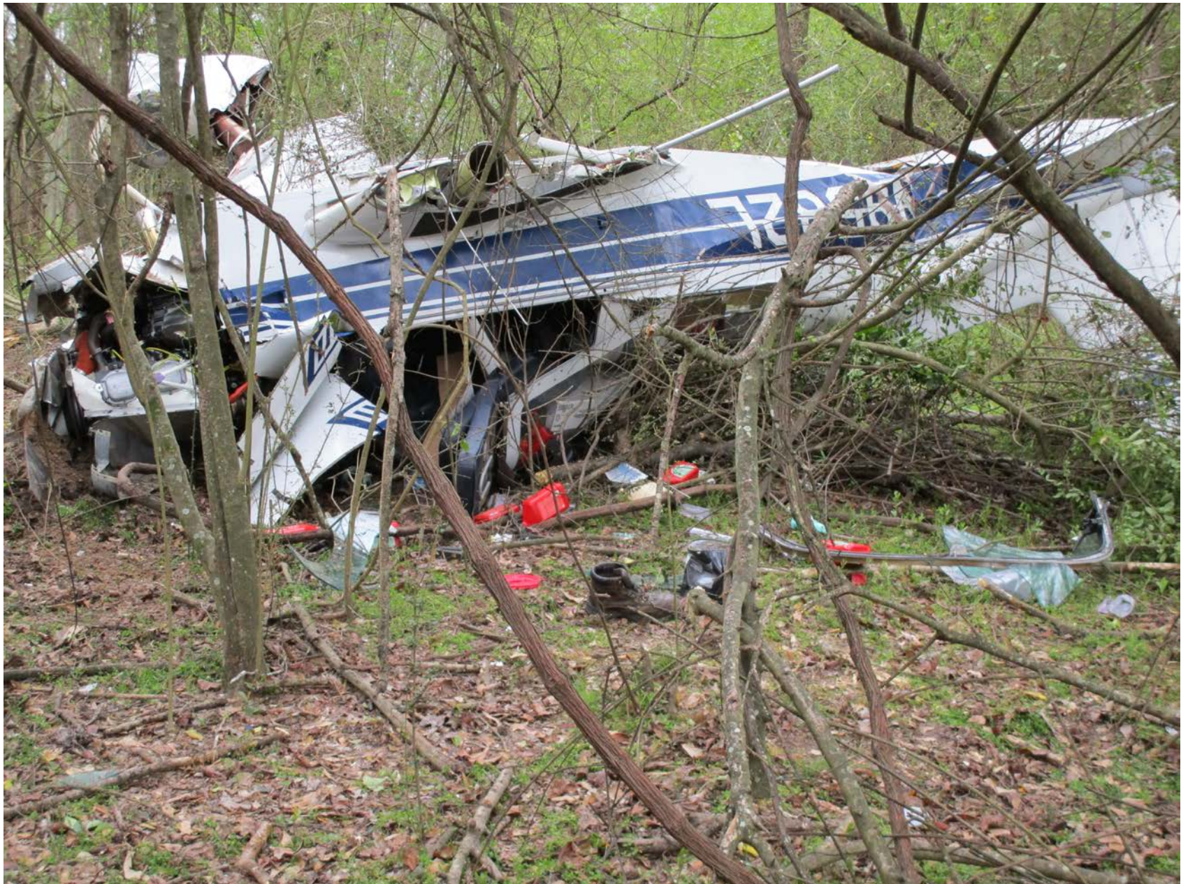
Photo 2 – Inverted right side of N9582L.
