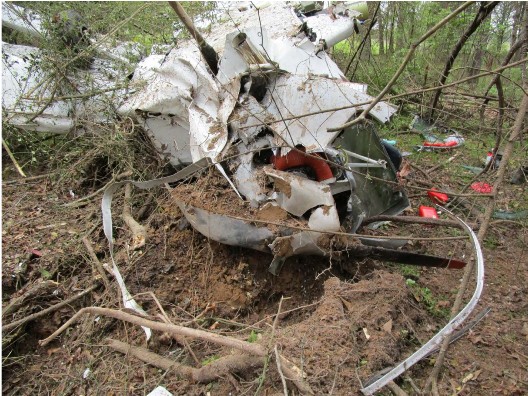
Photo 3 – The propeller still attached to engine after removal from crater.
