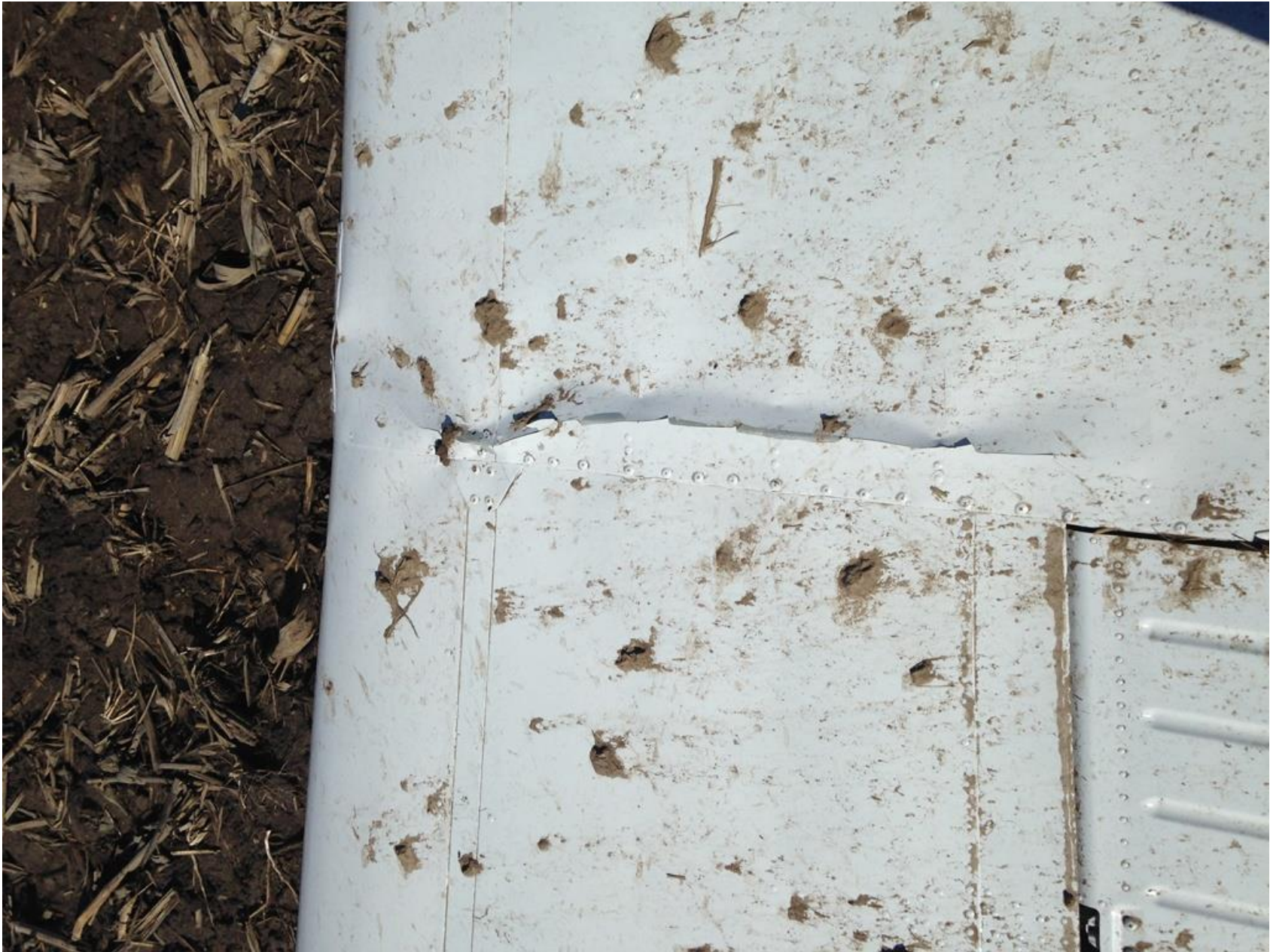
Photo 7 – Right Wing Damage
