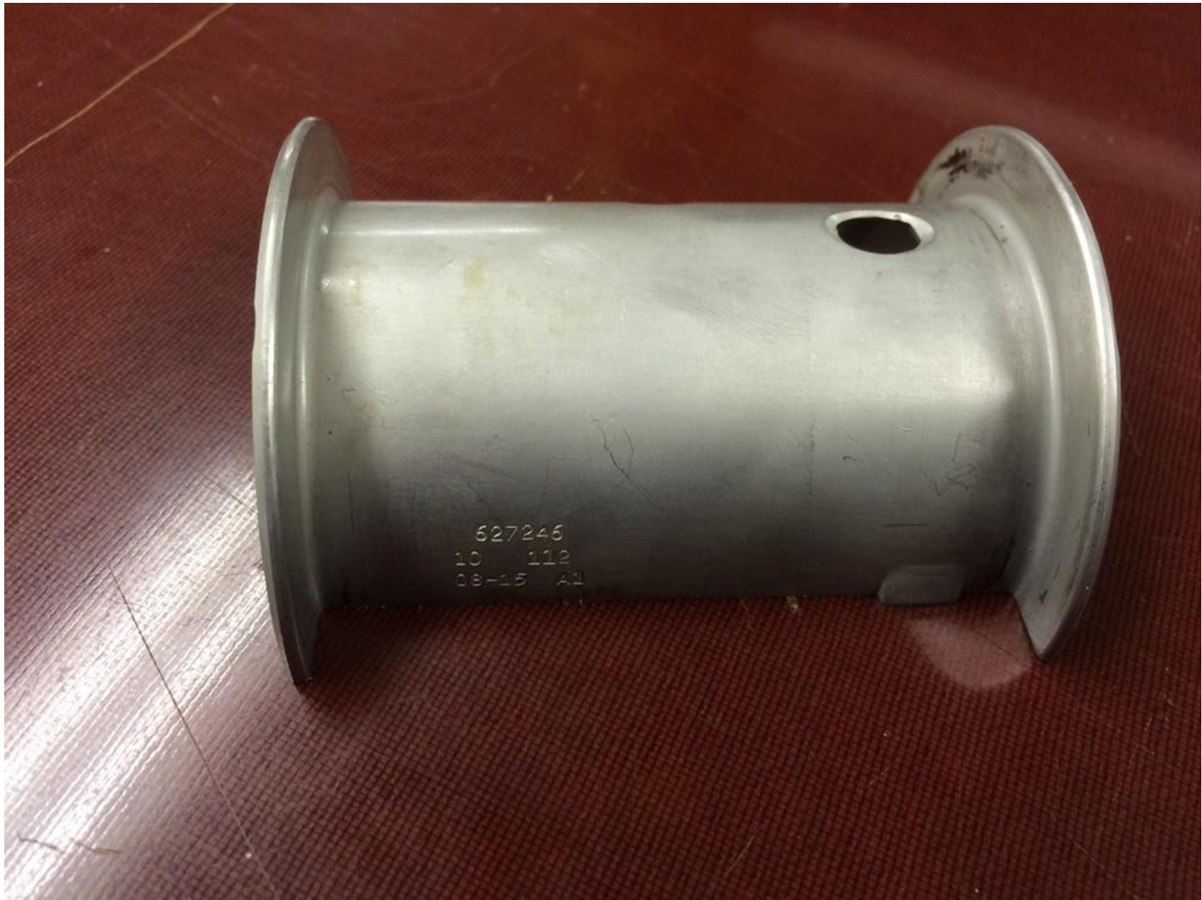
Photo 5 – Exemplar bearing and thrust washer assembly.
