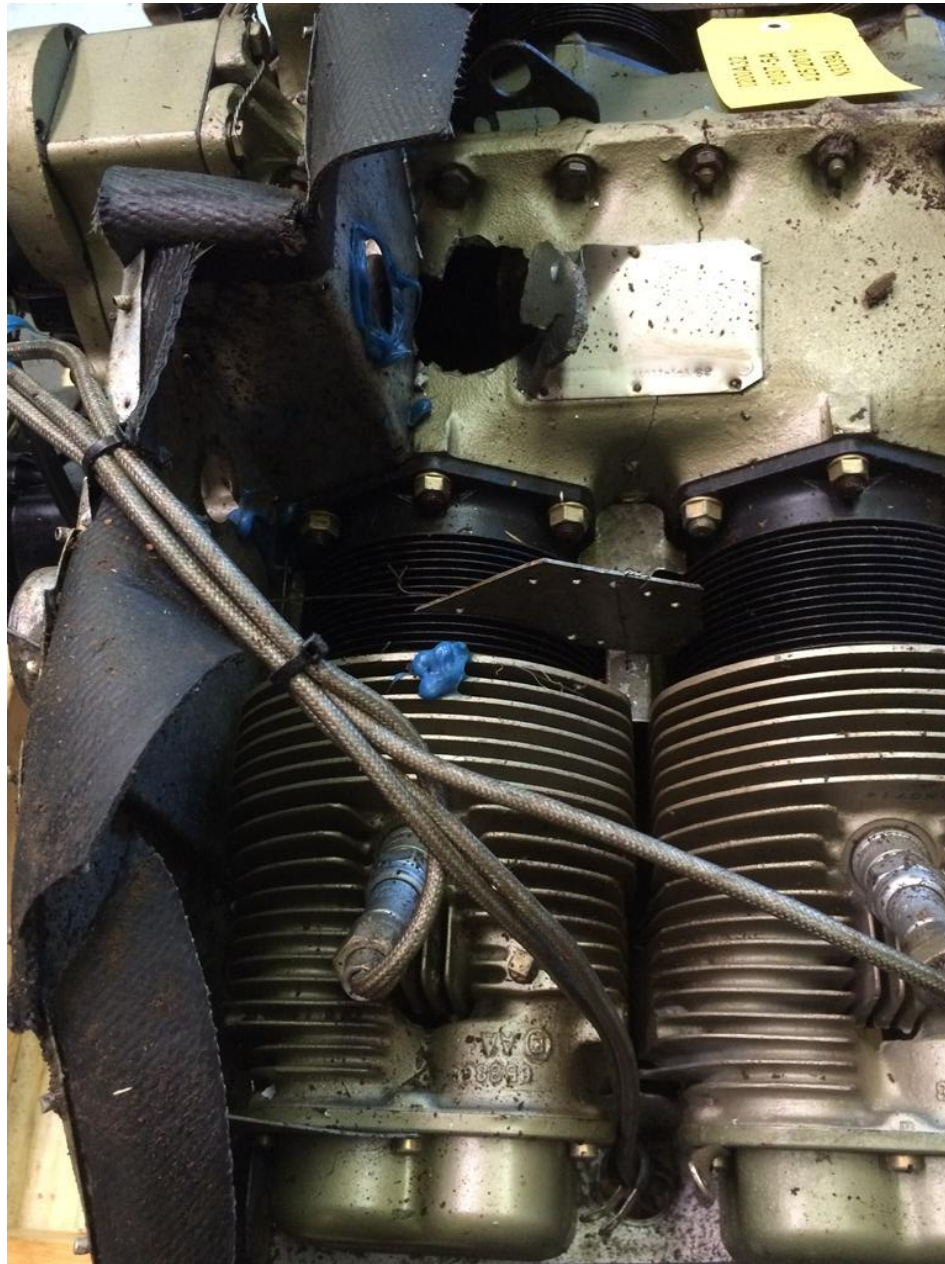
Photo 2 – Hole in the crankcase.
