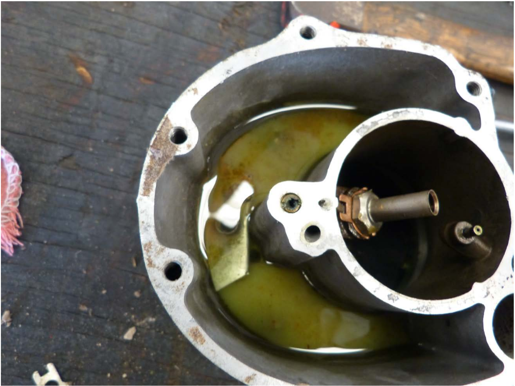
Photo 3 – Carburetor Bowl with Water Contamination
