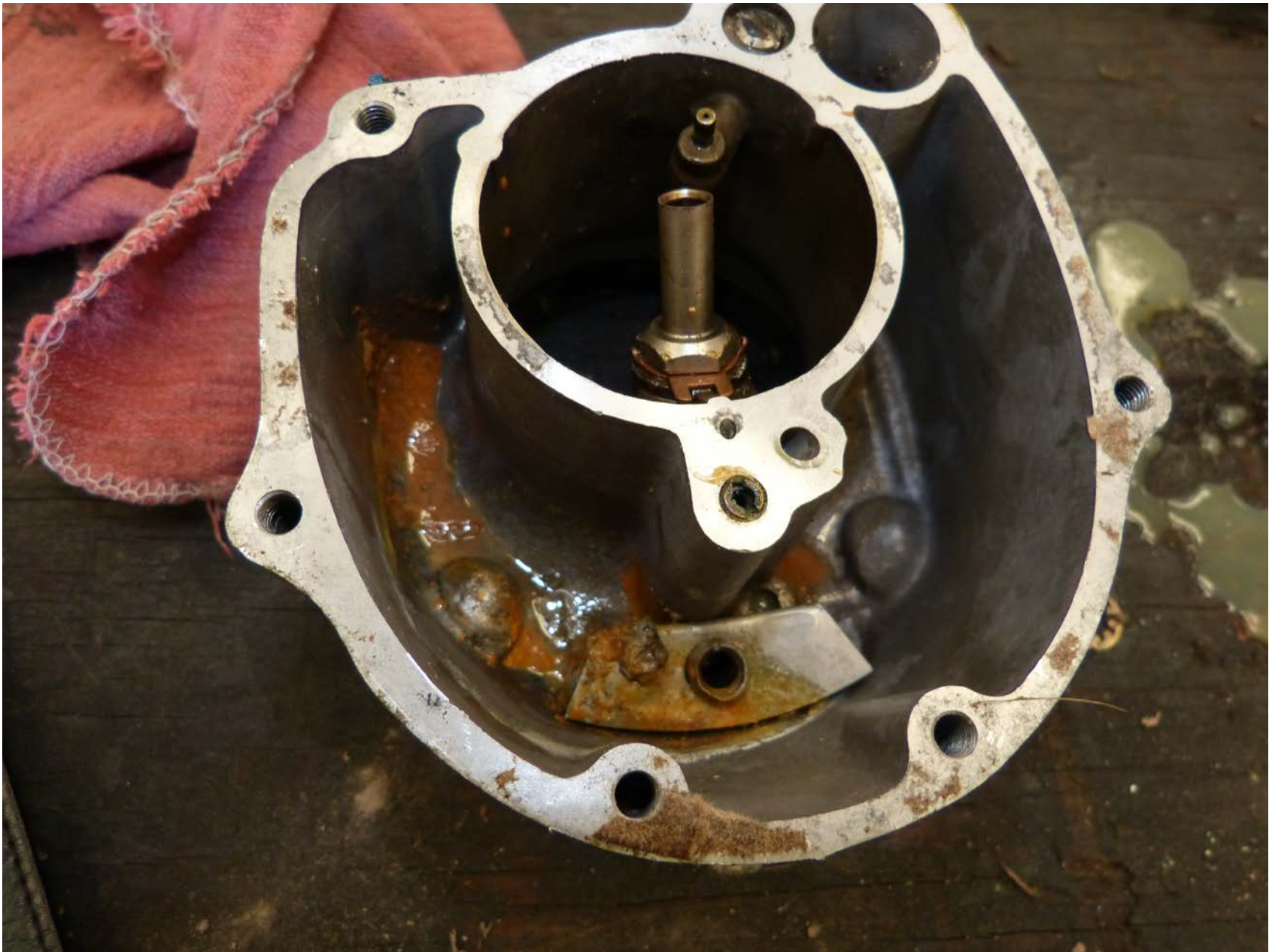
Photo 4 – Carburetor Bowl with Corrosion
