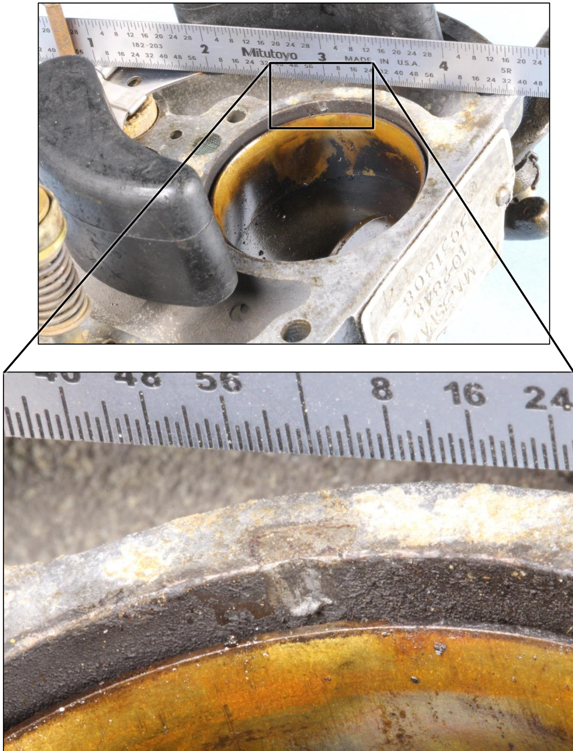
Figure 4. Contact mark in the area where legs of the primary venturi would contact the throttle body as assembled in the carburetor.
